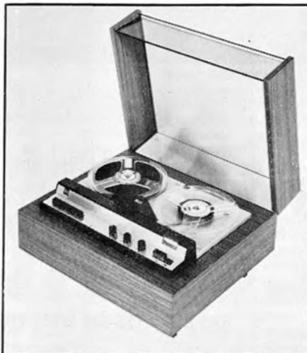
The main function switch near the centre of the control panel has a central 'stereo' position where each channel records and plays stereo signals from microphone, radio or gramophone. The adjacent gain controls can be locked together so that the volume of the two channels can be varied simultaneously by operation of either control.
