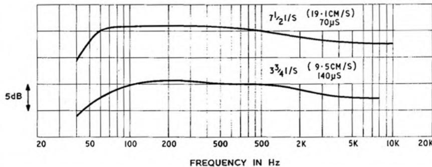
FIG. 3 DUAL TG27 RECORD/PLAY RESPONSE (GRAM INPUT TO MONITOR OUT)
