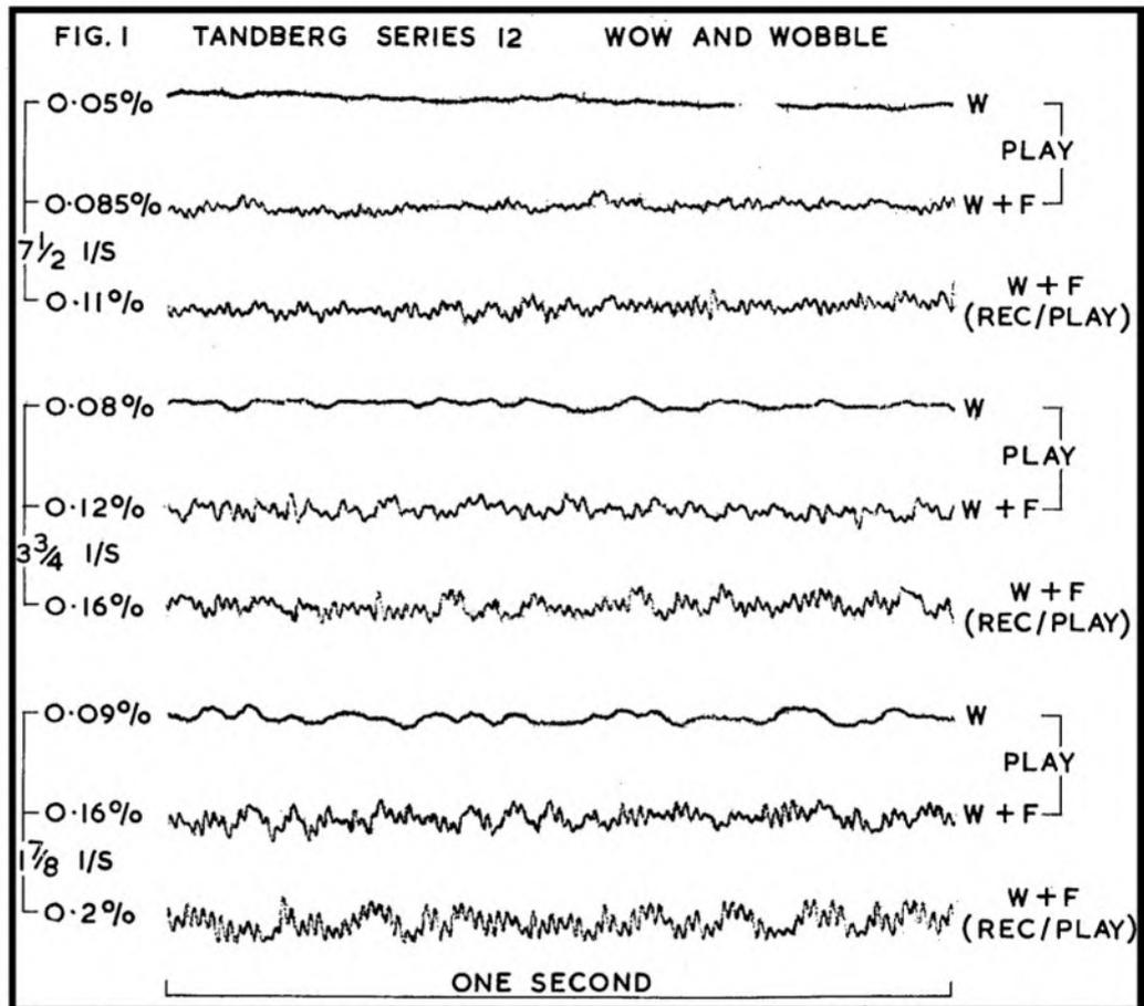
the play-only wobble of the machine under test. The lower traces are for record and play, where some components of the short-term speed
