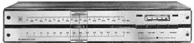
**BEOMASTER 5000.** Stereo F.M. Tuner with usable sensitivity of 1.5 $\mu$ V. Automatic Mono/stereo switching, 4 stage gang tuned R.F. section, 5 I.F. stages and A.F.C. Large radicator calibrated relative to signal strength. Cursor type tuning control with vernier adjustment. Variable muting and stereo levels. Aerial inputs for 75 ohm, 300 ohm and local. Identical in size and cabinet finish to match Beolab 5000.
