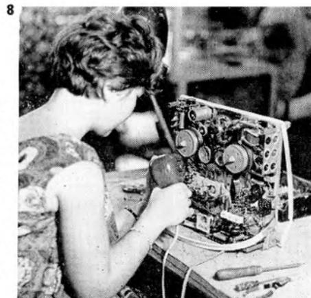
All the fundamental electrical units are assembled on printed circuit boards, mutually interconnected by cable forms. The boards are also made in the factory. I was surprised to find that, in this particular department, the well-known acid etching method has been completely abandoned. Heavy automatic presses cut out the required pattern of copper foil and glue it to cuprextite boards, into which they punch the necessary holes. This is done in one operation at remarkably high speed.
