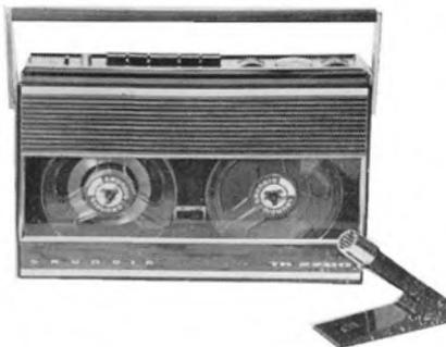
A 5 in. (13 cm.) spool capacity, brushless DC motor and twin contra-rotating flywheels are features of the *TK 2200* which supersedes the *TK 6*. Unlike the latter, however, it is designed solely for battery operation and weighs 10 lb. Speeds are 3½ and 1½ i/s (9.5 and 4.75 cm/s) with claimed respective frequency ranges of 40 Hz-15 kHz and 40 Hz-8 kHz. Dynamic range is 47 dB at the higher speed and 46 dB at the lower. Wow and flutter at 9.5 cm/s is ±0.25% and the price is £78 15s.
