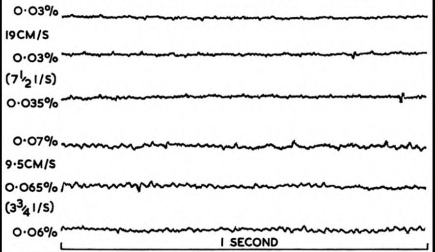
FIG. 2 REVOX A77 PLAY/ONLY RESPONSE (TEST TAPE TO LINE OUTPUT)
