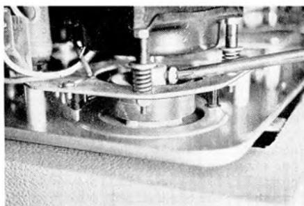
Underside of spool carrier of Magnavox Studio deck, showing screwed clamp which holds turntable to motor spindle. A Phillips screwdriver engages with one of the clamping screws. To the right can be seen the wirewound resistor that limits the supply to the motor.
