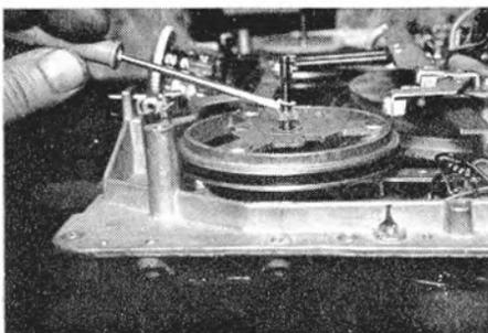
Philips turntable with individual lifting spindle to separate upper and lower halves. The neoprene washer is clearly seen, and the vulcan plugs inserted in the lower section. This is the left-hand, supply spool, turntable, but is similar to the take-up except for the shape of the step on the spindle.
