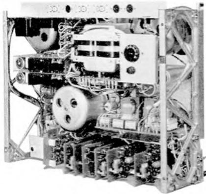
slightly eccentric pinch wheel which caused audible fluctuation of open-string guitar tones and sinewaves with certain thicknesses of tape. Although this measured only 0.06% RMS at its highest, the effect was worse than one might expect since it comprised almost entirely low frequency wow. This pair of trustworthy ears found wobble inaudible on slow orchestral and light popular music.
