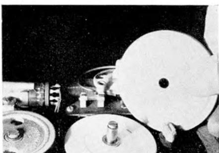
Grundig gravity clutch, showing the upper and lower halves separated. Note machining of spindle and bush in lower half. Felt disc is fixed to underside of upper half. Idler wheel at left gives direct drive for fast winding: for take-up, lower half of clutch assembly is driven by a belt coupled to the flywheel.
