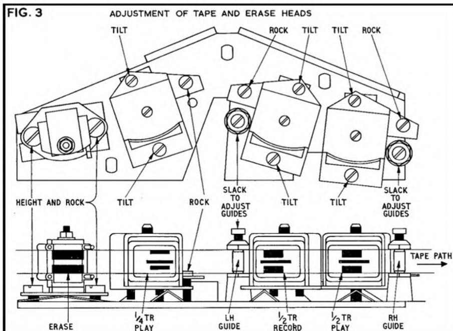
B & O 2000 head mounting, omitted from last month's column due to pressure on space.
