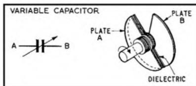
away from each other, it is possible to vary the capacitance over a small range. The tuning control on a radio receiver is generally a
