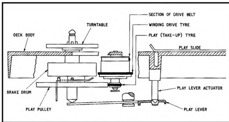
Fig. 8. Ampex 753 arrangement.
