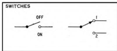
slightly more versatile *two-pole* switch is shown on the right.
