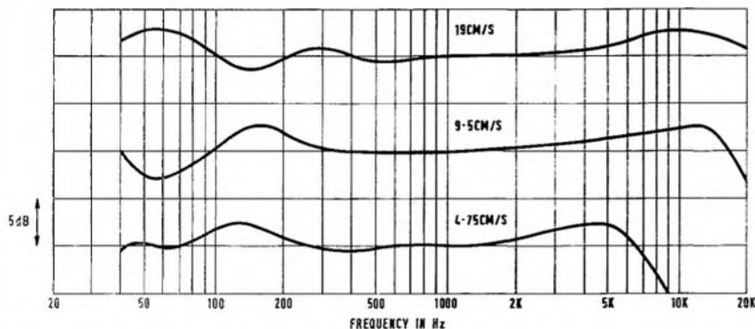
**FIG. 5** FERGUSON 3232 ACOUSTIC RESPONSE (WHITE NOISE TEST TAPE)
