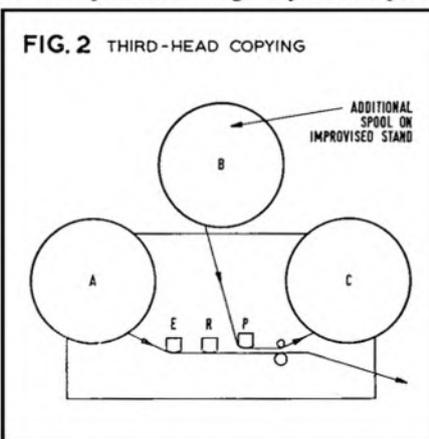
be copied is placed on the carrier (spool B in fig. 2) and threaded past the replay head and capstan to spool C. Spool A, on the left-hand turntable, contains the tape which will receive the copy. This is threaded in the normal way but travels from the capstan straight to a clean floor or wastepaper basket. There is absolutely no danger of tangling or damage, provided the
