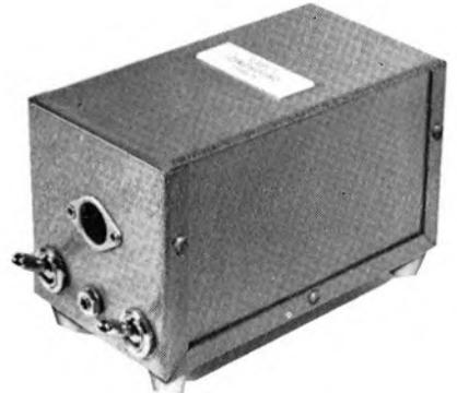
pulse generated within the camera to an inaudible pilot signal. This signal is recorded with the film sound on to a conventional single-channel tape recorder. The R.1 is battery powered, measures 10 x 5 x 4 cm, and incorporates a miniature jack pulse input and three-pin DIN tape output. A battery life meter is also fitted.
