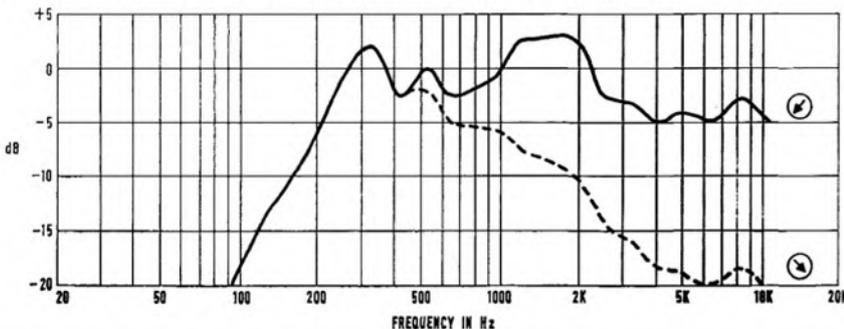
**FIG. 6** FERGUSON 3232 MICROPHONE RESPONSE (500 OHMS)
