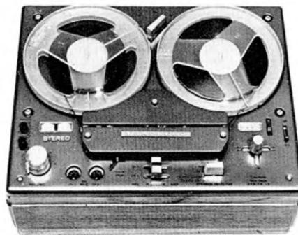
at the top corners, i.e., beneath the spools. The plate has two rubber mounts beneath these screws (the reassembling secret is a touch of wax), and the compression of these rubbers gives the last adjustment for deck level.
