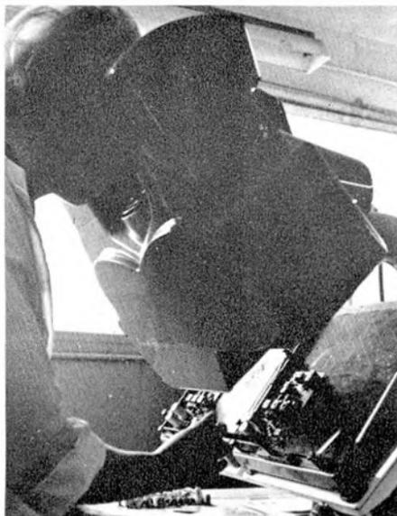
Checking Truvox IC FM tuner printed circuit board with a master board by means of a comparascope.
