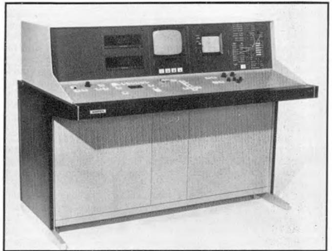
Ampex *HS-200* disc recording and computer-controlled editing system.
