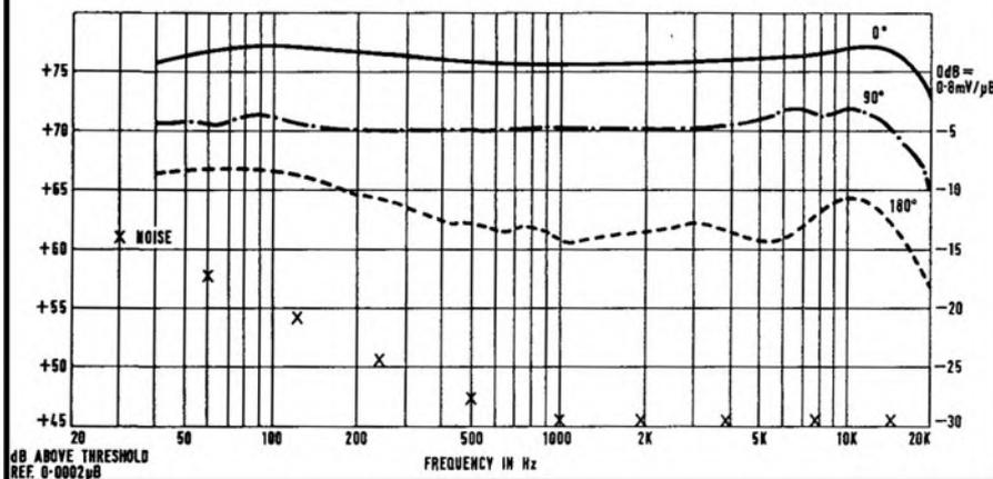
an output of 5 mV for a 26 mm diameter unit. The lowered sensitivity of the microphones under test is proportional to the drop in voltage to 65 V but this is inevitable with the relatively soft plastic diaphragms used in these microphones which would be pulled against the back plate by a higher polarising voltage.
