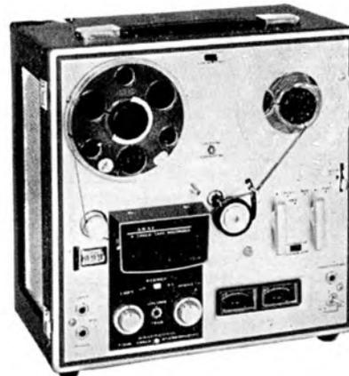
**AKAI I710W Stereo Tape Recorder (left).** The Shield Type Head for High S/N Ratio. 4-track stereo/monaural recording and playback. 3-speeds (1½, 3½ and 7½ ips (15 ips optional)). Automatic shut off. Pause lever. Tape cleaner. Tape shifter in fast forward/rewind operation. 4 hours maximum stereo recording capacity with a 1,200 feet tape. DIN jack, Stereo headphone jack. 3-digit index counter with reset button, VU meters. Finely oil-finished wooden cabinet. List price £109. Our price £89 10s.
