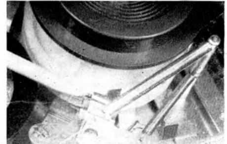
be small brass washers next to the slightly raised bearing bush on some models. In any case, the trick is to ensure that the lower washer is not gritted up. Remove and clean the wheel and its boss, the spindle and the washers, and refit with a single drop of oil. Then, after tightening, spin it freely and add a drop or two of oil to the reservoir at the top (felt ring).
