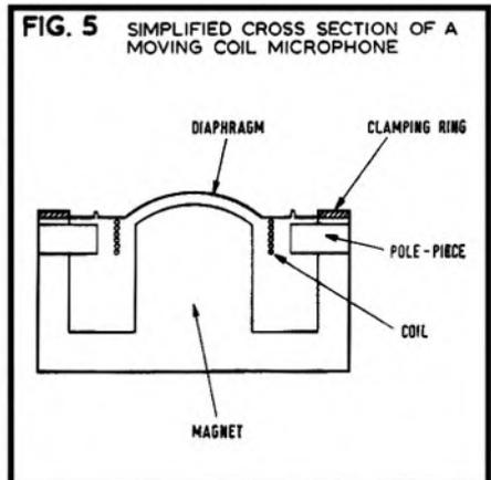
phase shift across the diaphragm and diffraction are less marked, but the smaller the microphone the lower the output level, so the size of the microphone is chosen to obtain a compromise between response and output level.
