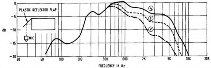
FIG.6 NATIONAL RS-790S MICROPHONE (1K IMPEDANCE)
