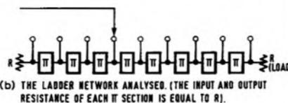
FIG. 8 EQUIVALENT CIRCUIT FOR A 600 OHM LADDER FADER AT MINIMUM ATTENUATION SETTING
