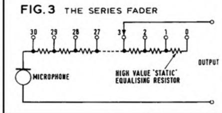
differences, and 0 dB is any arbitrary value.) This potentiometer is designed to have an input resistance ( $R_{in}$ ) of 600 ohms, and the load resistance ( $R_L$ ) is assumed to be high compared with  $R_P$  so that the shunting effect of the load on the potentiometer is negligible.
