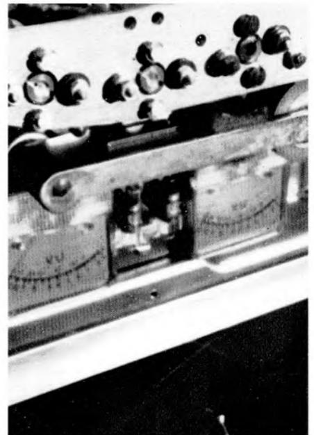
head return lead, measuring the resultant output at the cathode follower. As a reference, a 1 kHz signal is adjusted to give a reading of 70 mV output. Other readings are related to this input, and will vary a lot, depending on the equalisation. A few spot frequencies will give some idea of the response. These figures are for the 70  $\mu$ S equalisation curve: +19.5 dB at 40 Hz, +10 dB at 250 Hz, -4.5 dB at 4 kHz, -3.5 dB at 10 kHz, -2.5 dB at 10 kHz. This is with the speed selector at 19 cm/s.
