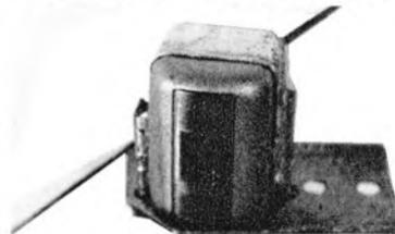
FIG. 8 Cut-away head bracket.
