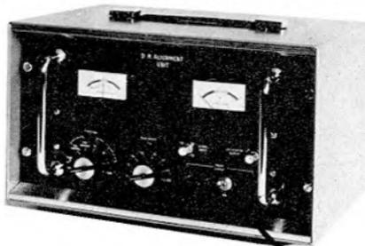
playback level, and frequency response. The 2nd harmonic test facility is included since, if greater than 1% distortion, it implies magnetised heads or guides. Tape speeds of 304 down to 2.325 cm/s may be accommodated. Dimensions are 364 x 237 x 213 mm.
