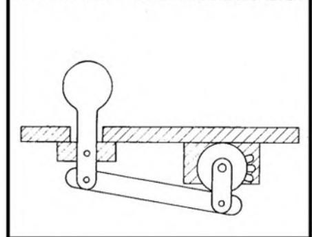
FIG. 30 IMPROVED METHOD OF OBTAINING POTENTIOMETER LEVER ACTION
