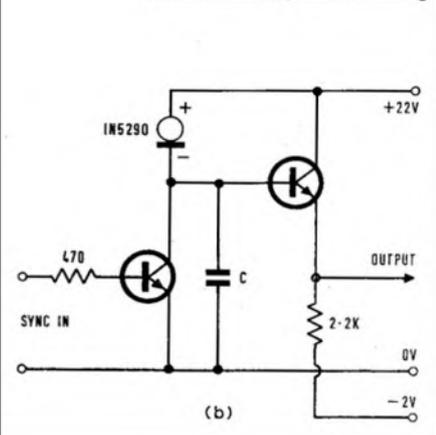
**FIG. 43** METHOD OF COUPLING A UNIJUNCTION OSCILLATOR TO A LOAD
