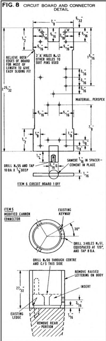
through the hole in the connector, and the connector fixing holes are marked through those in the body. The connector is removed, its insert taken out, and the three holes drilled and tapped. The board spacer is also drilled and tapped. Incidentally, the reason for using the spacer is not to support the board, but merely to allow the whole assembly, connector included, to be withdrawn as one unit, and it may be omitted at the expense of a slightly more fiddling assembly.
