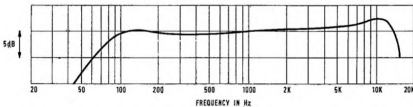
FIG. 4 PHILIPS 4307 ACOUSTIC RESPONSE (WHITE NOISE TAPE ON SPEAKER AXIS)
