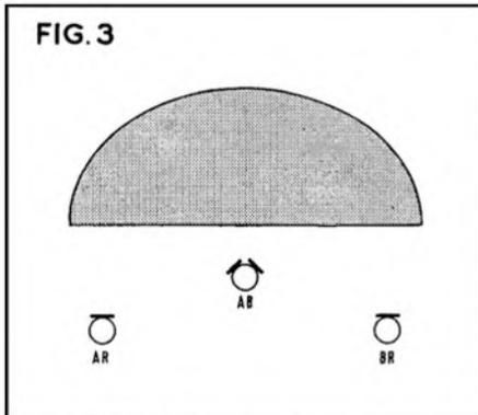
**Fig. 3.** Stereo microphone layout for either 2-channel or 4-channel stereo. In BBC usage AB might be a C12 or a pair of C24's and AR and BR individual C24s. This is one of a range of four microphone (or four-element) layouts which can readily be adapted to the four-channel system.
