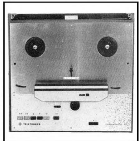
interesting to find that this level and distortion were obtained with bias set for maximum output of the 1 kHz tone and that overbiasing, to drop the 1 kHz signal by 1 dB and then resetting the level by 1 dB, gave no further improvement in distortion. This may be a function of the very low losses in the ferrite record head.
