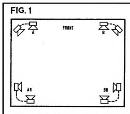
Fig. 1. Four-speaker layout. The arrangement should be symmetrical about a front-to-rear axis, but the rear speakers, AR and BR, need not be opposite the corresponding front speakers, A and B.
