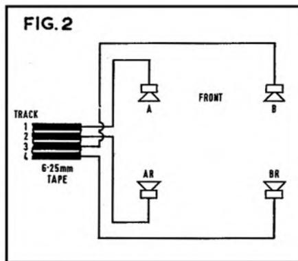
Fig. 2. The Vanguard track configuration for 6.25 mm tape.
