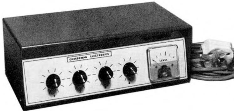
\*Mains powered    \*Two input levels per channel; low level for microphone, high for gram or tape
