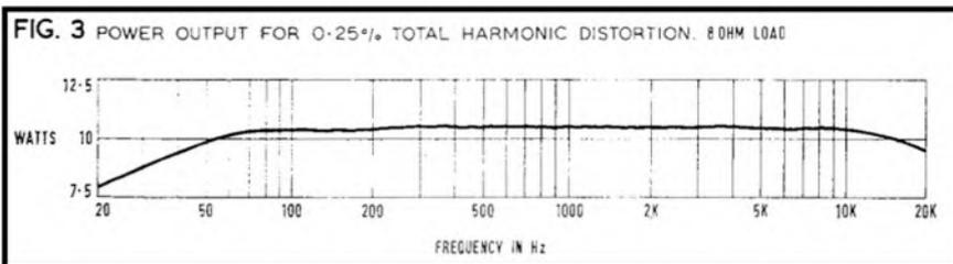
frequency between the beginning and the middle. The overall performance figures were obtained using BASF LH/LP35 tape on 18 cm spools.
