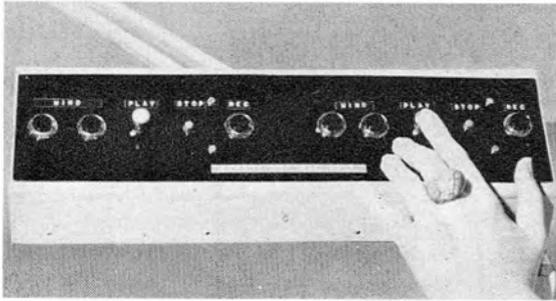
THE advantages of remote tape recorder control in a recording studio cannot be over-emphasized; it is almost a basic necessity. Indeed, even for the amateur it can be a great asset. The Revox A77 recorder is supplied wired for remote control and the remote control connection appears at the rear of the chassis on a Hirschmann *Wist* 10-way socket. The plug is supplied with the machine with Pins 1 and 2 shorted together.
