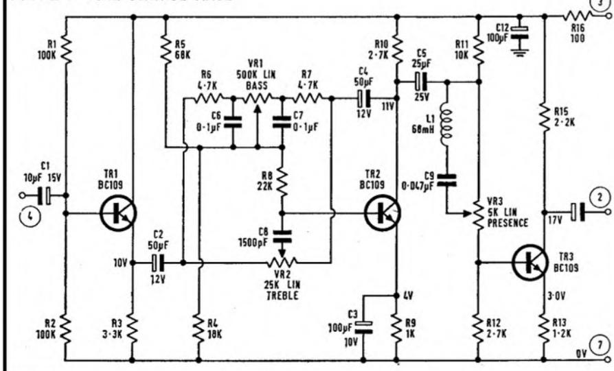
the second transistor and at the same time variable feedback is applied to the first stage by C2 and VR1, which raises the input impedance so that the transformer is correctly loaded by R1 only. VR1 appears as a front panel control, and is used to present roughly the amount of gain required so that the quadrant faders, which are the main controls per channel, are all approximately in the same position; this makes for easier mixing.
