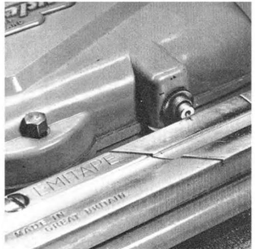
EMI jointing block mounted to operate Ferrograph pause control.
