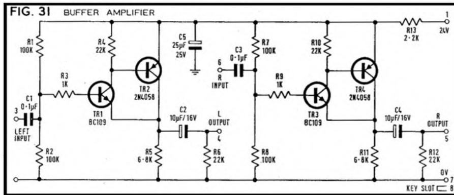
and has been described already for use in the plug-in front panel modules; for completeness the circuit is shown again in fig. 31, which also shows that one small internal card will accommodate two such buffers, quite independently.
