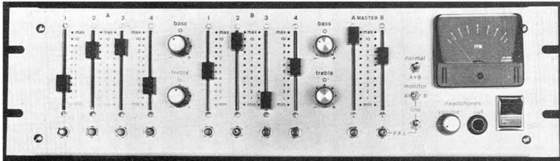
OUR NEW EIGHT INPUT MONO/STEREO MIXER. AVAILABLE ON SHORT DELIVERY. FITTED WITH ANY INPUTS FROM OUR EXCLUSIVE AUDIO MODULE RANGE. BROADCAST STANDARD P.P.M. OR VU, PREFADE LISTEN AND 2 WATT MONITOR AMP. EXTERNAL "CURVE BENDING" FACILITY. TWIN 600 OHM FLOATING BALANCED LINE OUTS. SIMPLE, RELIABLE. AND IT DOES NOT COST THE EARTH.
