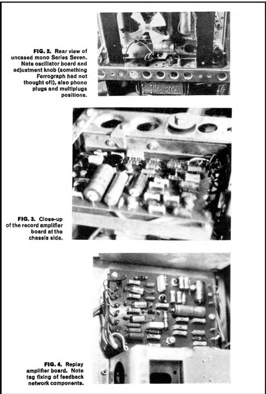
**FIG. 2.** Rear view of uncased mono Series Seven. Note oscillator board and adjustment knob (something Ferrograph had not thought of), also phono plugs and multiplugs positions.
