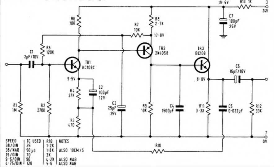
FIG. 28 STEREO COMBINER CIRCUIT
