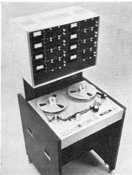
and, when connected to mains, will record at 72 cm/s. Electronics are resin-encapsulated in metal-screened plug-in modules. Items in the Sennheiser range of capacitor microphones were shown, and the HD414 stereo headphones and Audio Engineering PPMs demonstrated.
