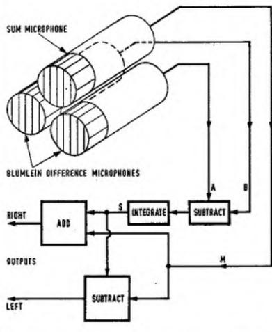
distance  $d$  is 2.5 cm, the three-microphone arrangement gives a reasonable unilobe characteristic and excellent stereo separation up to a frequency of  $\frac{1}{2}(c/d) = 6.8$  kHz, and the stereo separation virtually disappears at a frequency of about  $(c/d) = 13.6$  kHz. Thus good stereo can be obtained by using the Blumlein difference technique with three microphones, even with a microphone separation of 2.5 cm. The results with smaller microphone separations will be even better.
