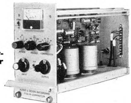
The new F700 Compressor provides a range of compression slopes from less than 2:1 to greater than 25:1; switched attack control for special effects; switched release control from 25mS. The threshold level is switched with compression slope to provide a constant level of output for 17dB reduction. Normal output level (unattenuated) +8dBm. Noise better than -75dB below Limit level Distortion: 0.1% for 25dB reduction.
