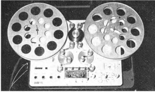
Sondor M3 sprocketed film sound recorder
