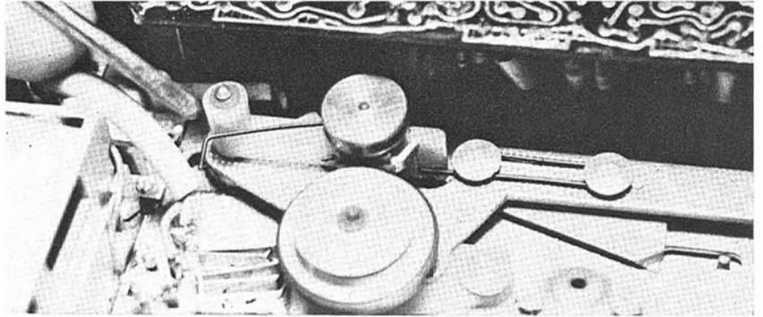
**Fig. -** The main function knob controls all switch actions and drive engagement, including this clutch pivot. The flywheel has been removed to show the hairpin spring on the main function lever.
