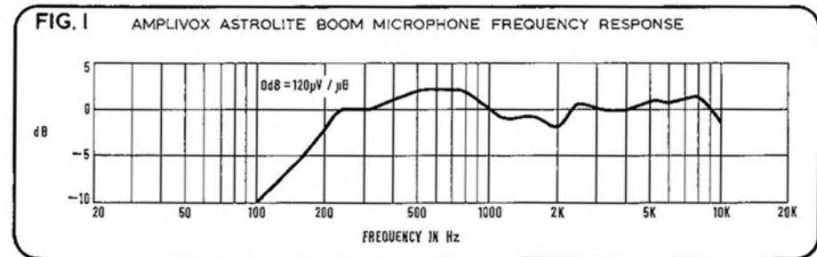
is shown in fig. 1. The response did not alter with distance from the sound source, indicating that the microphone has a pure pressure response. There are noise reduction properties due to pressure gradient effects. The bass cut below 250 Hz explains the better speech balance when listening to the microphone-headset combination.
