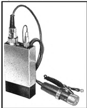
Of the range designed and made by Audio Limited, Receiver RMS 7 with Transmitter A.U.18 find particular favour where total concealment and maximum freedom of movement are essential. **AUDIO TRANSMITTER A.U.18** has a frequency from 100MHz to 175MHz, crystal controlled, with an audio response from 30Hz to 15KHz ± 2dB overall from transmitter to receiver output.
