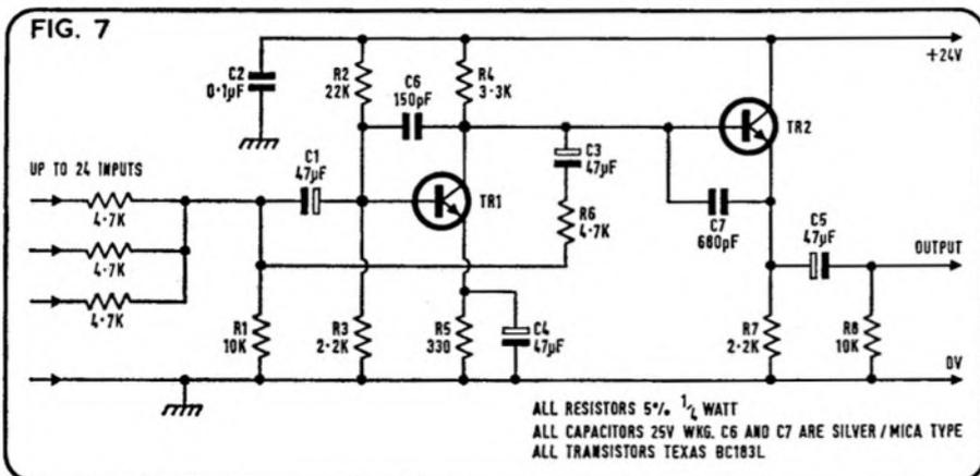
IN order to understand the operation of the virtual earth amplifier, it is necessary to be familiar with certain basic facts of negative feedback. A brief and non-mathematical approach to the methods used will first be given.
