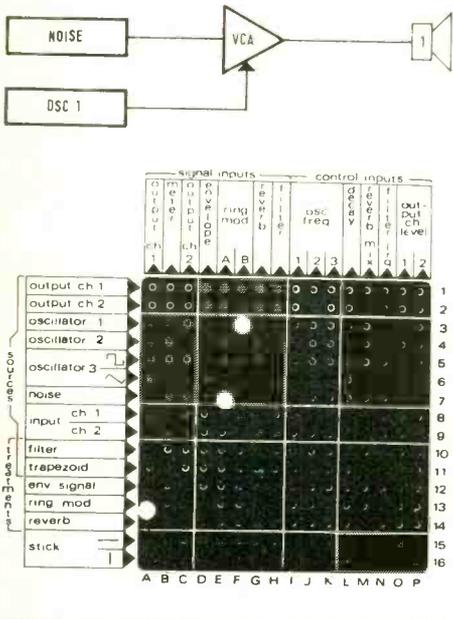
to input A of the ring modulator. A second pin at 3F routes the output of oscillator One to input B. Setting a 1 Hz sinewave from oscillator One (fig. 5), the vca integrates this with the noise signal to produce a 1 Hz rise and fall in noise amplitude: a very approximate steam engine. Tones may be similarly interacted, perhaps the greatest value of the ring modulator being its ability to produce relatively complex waveforms from the three basic shapes generated by the oscillators.
