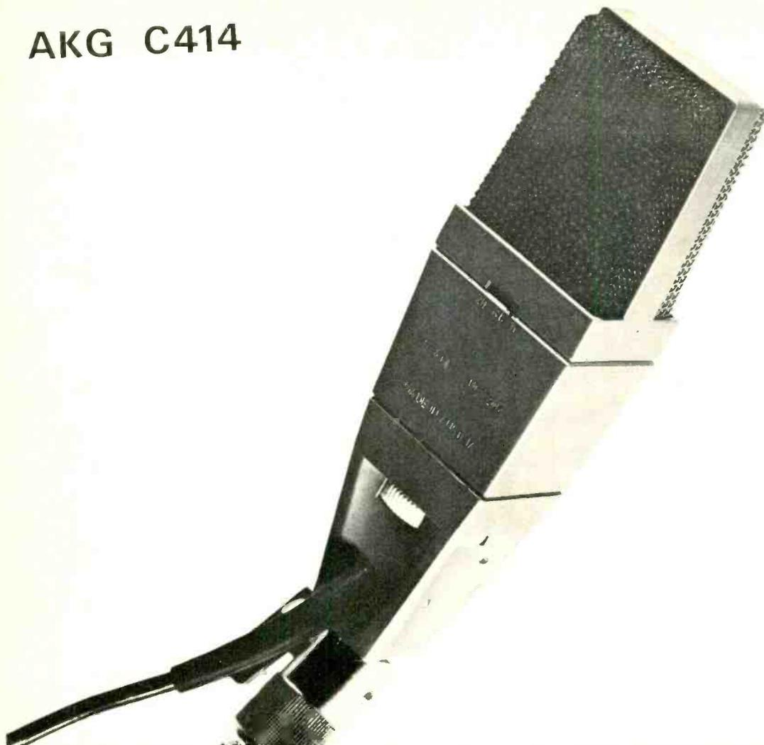
Take a good look at the NEW AKG STUDIO FET CONDENSER MICROPHONE TYPE C414. The pattern selector offers the choice of cardioid, hyper-cardioid (cottage-loaf), omni-directional and figure-of-eight characteristics. It also has bass attenuation device and 10 db pad.
