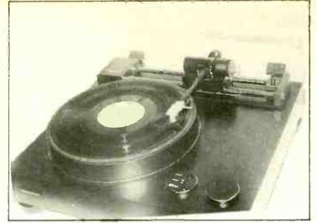
Pioneer turntable system with hanging rotor motor and linear motor drive tangential tracking tone arm
