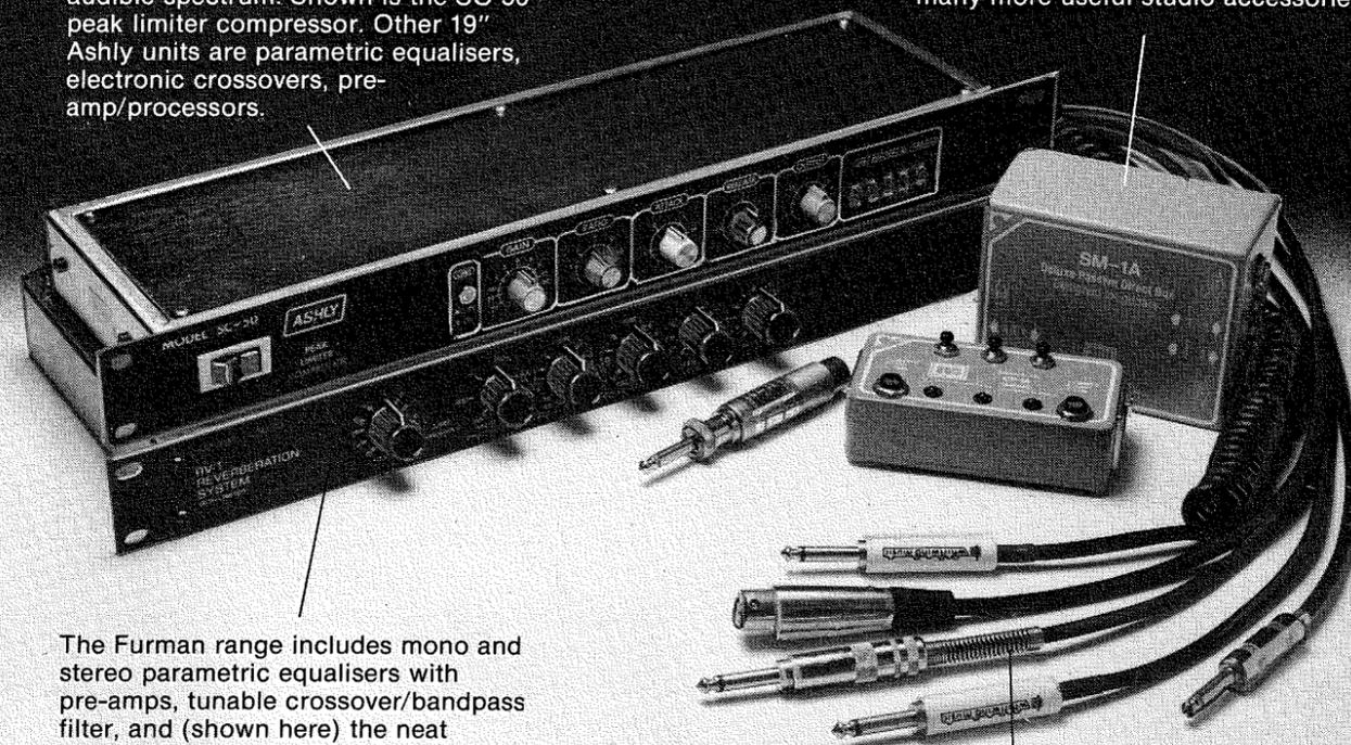
The Furman range includes mono and stereo parametric equalisers with pre-amps, tunable crossover/bandpass filter, and (shown here) the neat reverb system with limiter and equaliser. The simple layout and wide range of control gives full scope for creative engineering at a price which gives great value for money.
