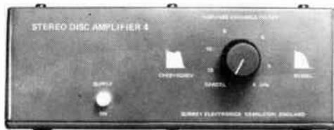
Supercedes Stereo Disc Amplifier 2. Unique Response Variable Filter which provides, through a single control knob, a 3dB turnover frequency variable between 13 and 4kHz but always with an appropriate phase and amplitude characteristic for psychoacoustic considerations. Ring or write for full specifications:
