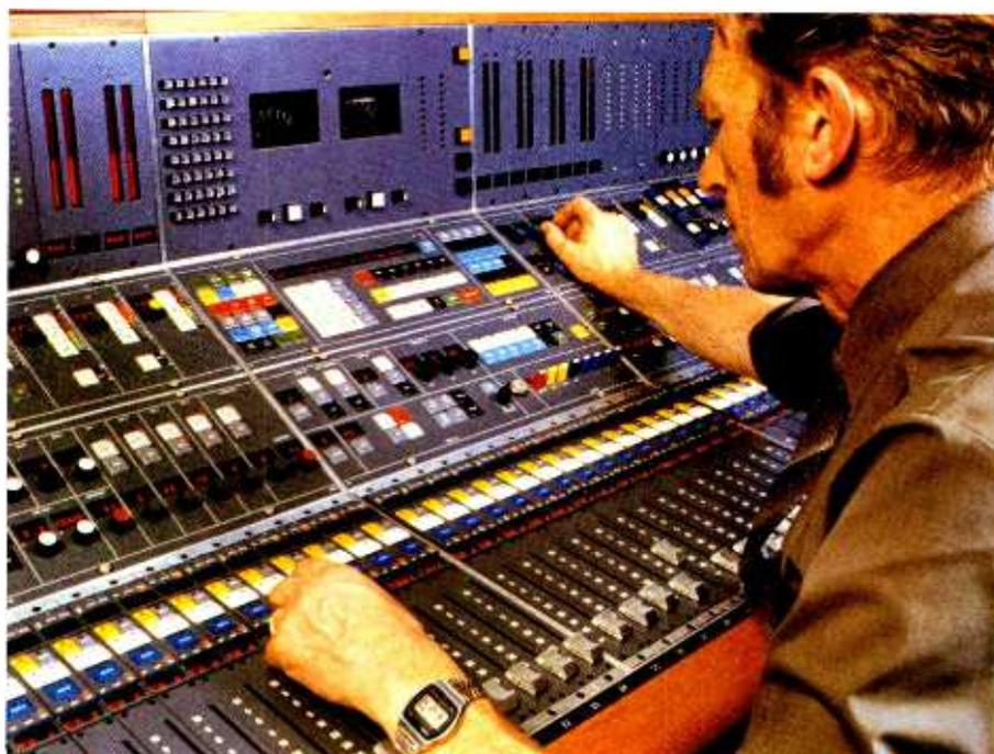
controls, faders, equalisers and compressors work by operating on the actual digital audio signals. The DSP console connects directly to digital tape machines and PCM links without intervening D/A and A/D conversions, thereby preserving every detail of signal quality.
