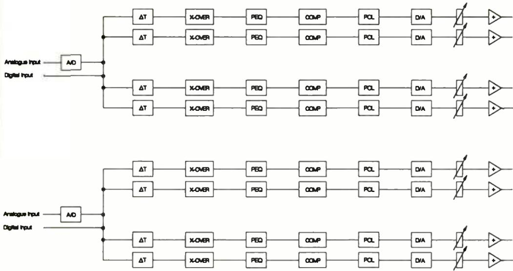
Fig.20: Block schematic for Yamaha D2040
