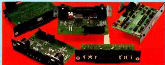
**OPEN INPUT ARCHITECTURE™** Flexible input cards allow the amplifiers to be configured with a variety of signal processing electronics.
