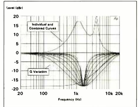
Fig.3: Parametric equaliser—combining effects and variation of bandwidth
