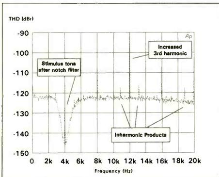
**Fig.14: As figure 13 but with 3982Hz stimulus characteristics**
