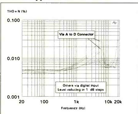
**Fig.11: Total harmonic distortion plus noise, no filtering, emphasis OFF**
