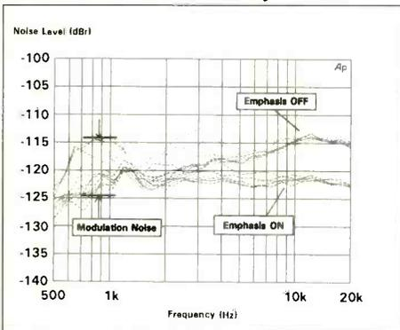
**Fig.10: Modulation noise—difference between upper and lower curves**
