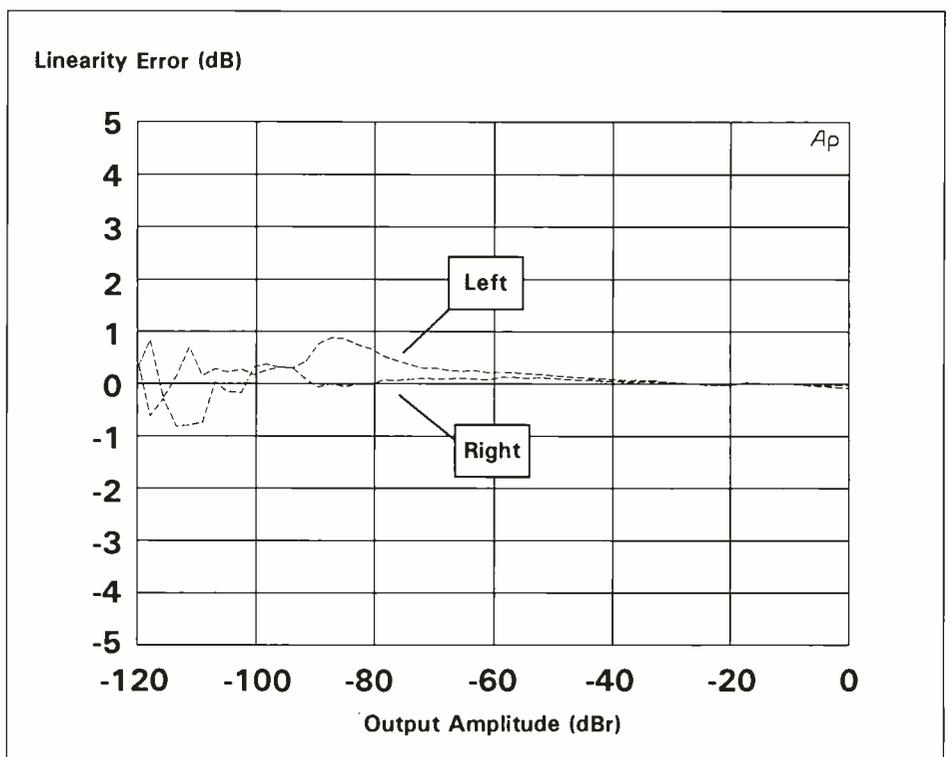
Fig.8: A-D plus D-A convertor linearity error
