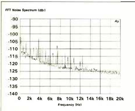
Fig.5: Noise spectrum, analogue input terminated in 50Ω emphasis ON
