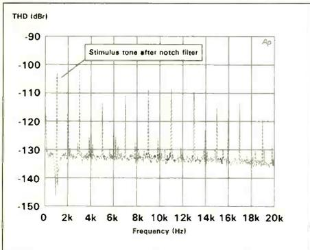
**Fig.13: THD Spectrum with 997Hz digital stimulus at -1dBFS**
