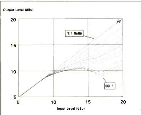
**Fig. 18: Compressor-limiter—effect of ratio variation**
