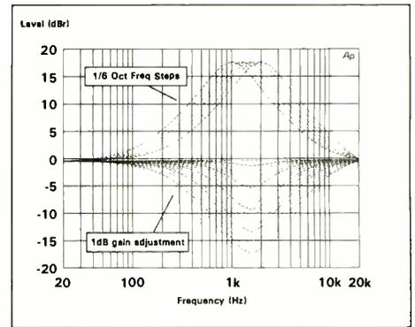
Fig.2: Parametric equaliser—frequency and level variation
