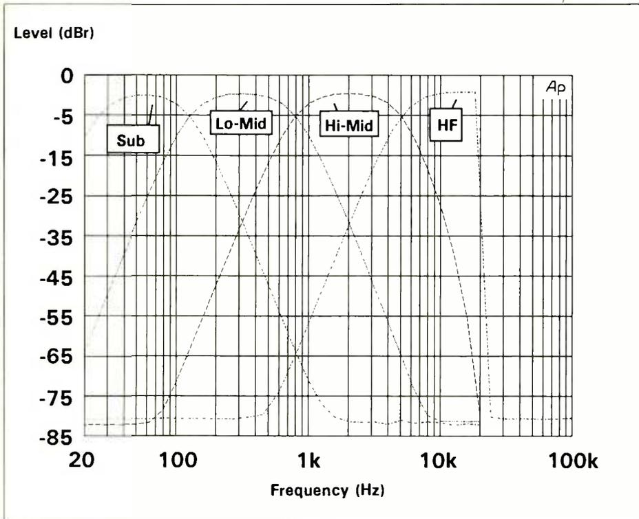
Fig.1: Typical four-way crossover characteristics
