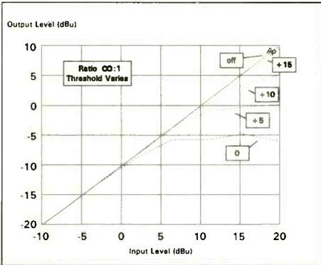
**Fig. 17: Compressor-limiter—effect of threshold variation**
