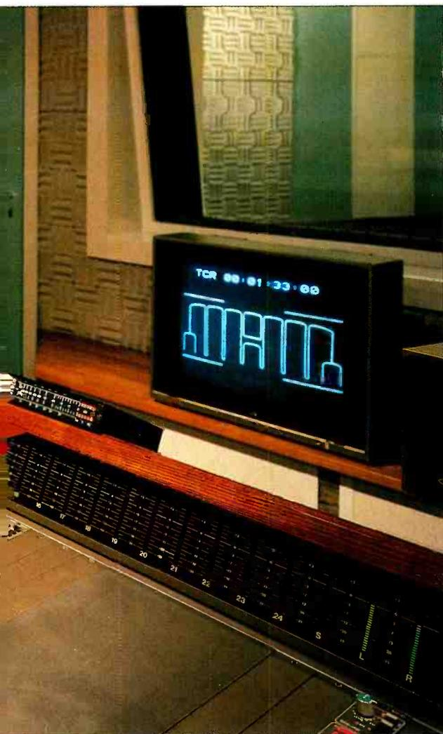
these, using all six digital channels, would consist of front left, right, centre and subwoofer and with left and right surround channels at the back. A moving display along the bottom of the screen enables the engineer to see forthcoming audio events before they arrive.
