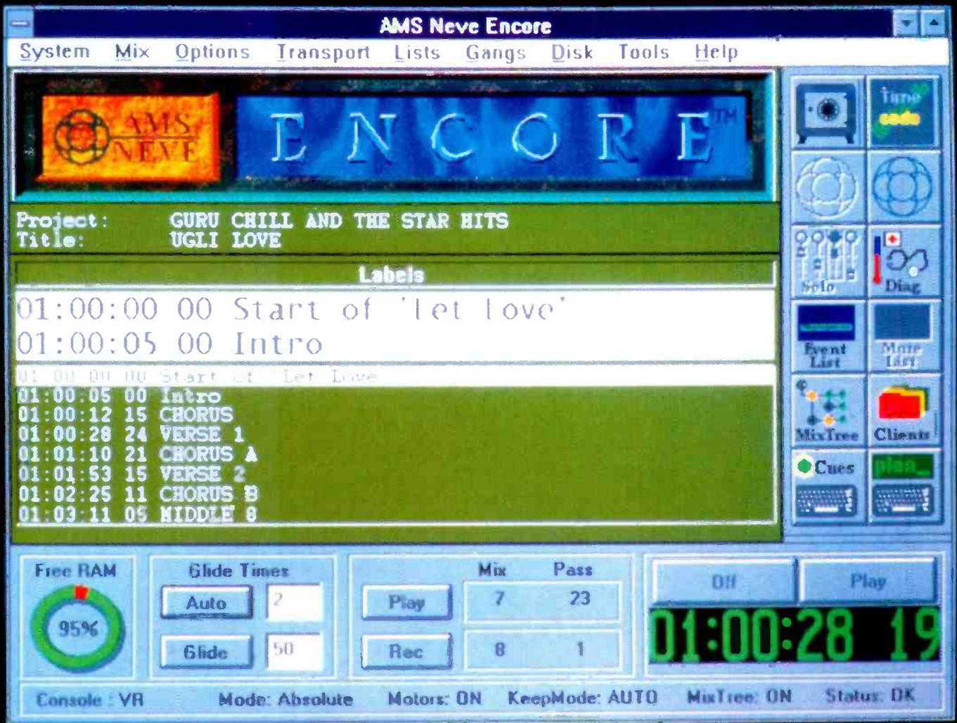
**P**ROBABLY. AMS Neve is introducing ENCORE™, a powerful new automation system. Encore uses a Pentium Processor, runs under Windows NT and combines the best innovations of AMS Neve's automation packages.
