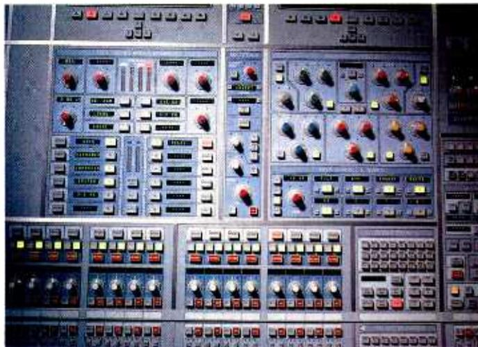
Close up of area of control surface covering EQ, dynamics, channel flow and multitrack
