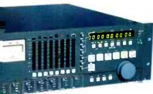
Paste style editing with full overlay and insert functions. Audio scrub and variable speed replay are included and the OMR 8 can record in the industry standard OMFI-compatible disk format.
