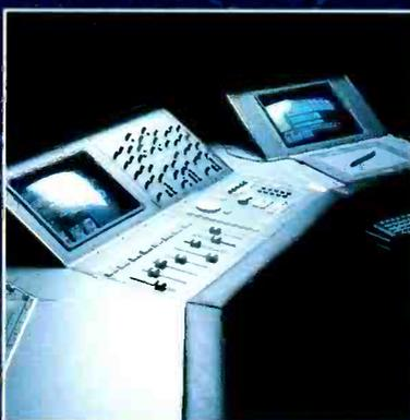
World-beating digital audio recording, editing and mixing system. Combines a 24-track random access recorder, multi-channel editor, 38-channel digital mixer, and random access video.
