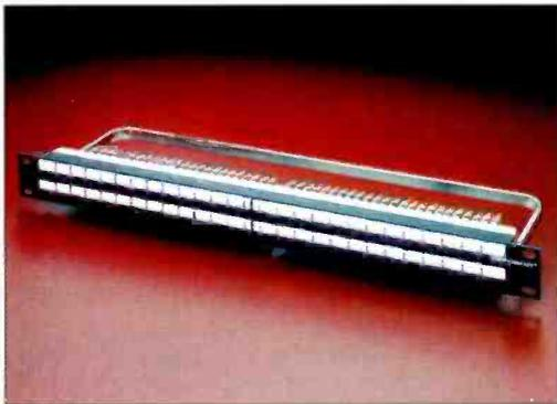
Switchcraft's new TTP96 Series Jack Panel (shown in photo) is built to last. It features corrosion resistant nickel-plated jacks, a steel frame for superior jack life and an aluminum, black anodized face and cable support bar. Switching arrangements available in full normal, half normal and open circuit. Fanned solder terminals make solder connections simple, and an offset ground terminal makes common ground buss connection easy.
