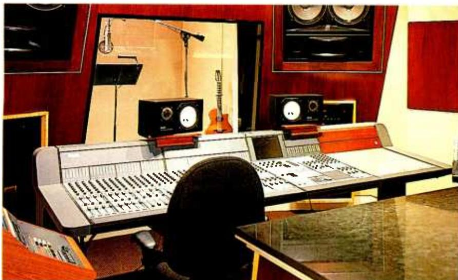
With the Euphonix, every keyboard is normalised into the board and available at the touch of a button.
