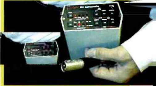
table digital and analogue output levels, plus channel ident on CH-B digital and right channel analogue. Validity bit selection for audio/data identification is also provided. LM1 monitor supports the same sample rates and has a headphone output with volume control. Accurate level indication is given for digital and analogue inputs, plus digital status and error monitoring.
