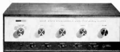
Model SA-2000 All-Transistor Integrated Stereo Amplifier. 36 watts IHFM music power (18 watts per channel). Response flat ( $\pm 1$  db at 1 watt, normal listening level) from 8 to 25,000 cps. Direct speaker coupling without output transformers results in speaker damping factor of 25:1. Complete controls and stereo headphone jack. \$159\*.
