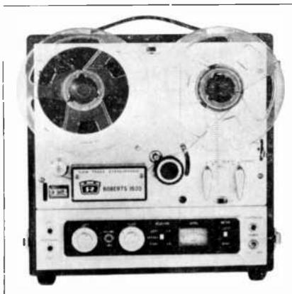
A nice recorder for the tape enthusiast with a limited budget. It doesn't have some of the convenience features and facilities found on more expensive recorders, but those it has are adequate and work well. Before proceeding with any of the instrument tests, we recorded on both channels with a low priced microphone and found that the Roberts 1630 gave a most pleasing account of itself. Later we recorded multiplex FM from an unfiltered tuner and found not a trace of beats from mix-
