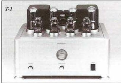
Marantz also displayed the spectacular Project T-1 Class A triode, push-pull 50 watt amplifier. The amplifier features four-300Bs in the front-end driving a pair of 845 transmitting triodes. Two additional 845s are used as rectifiers for the high voltage plate supply to the output tubes. Each 50 watt RMS amplifier has seven transformers (including three chokes) and is priced at \$25,000.
