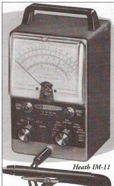
made a good VOM in a rugged Cyclolac plastic case, which was also sold as a kit by Heathkit. Small portable meters include the Simpson 160 and the Triplet 310. Many Asian meters, ranging in quality from terrible to excellent, were made at much lower costs than the American equivalents. However, even the best were generally less rugged than the better American models.
