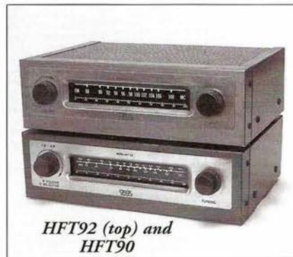
FM radio began to expand in the mid-Fifties and EICO wanted a piece of the action. Their first FM mono tuner was the HFT90 (\$39.95). A very compact, self-powered unit, the HFT90 featured a unique fluorescent "!" tuning indicator that doubled as the station indicator. These tuners are still very common and can still be seen at many electronic swap meets, probably because they can be unstable and prone to drifting.
