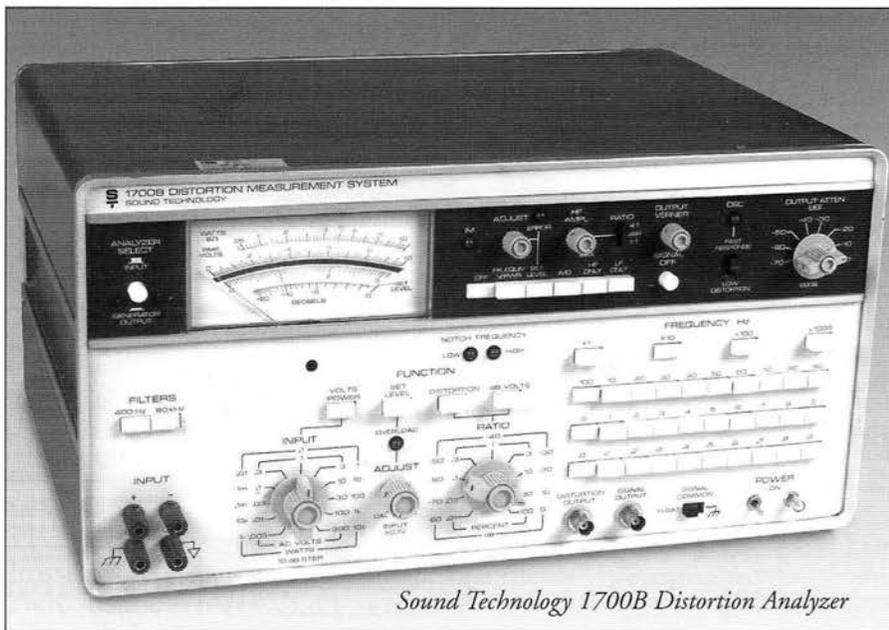
*Sound Technology 1700B Distortion Analyzer*
