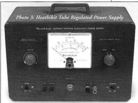
Photo 3: Heathkit Tube Regulated Power Supply
