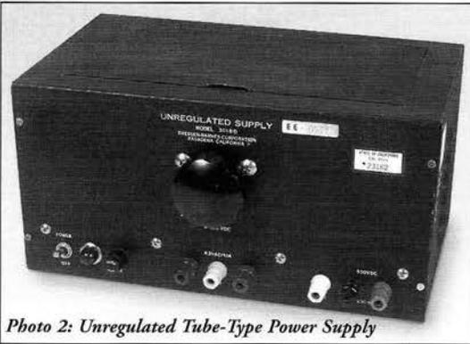
Photo 2: Unregulated Tube-Type Power Supply
