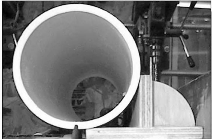
**PHOTO 17:** Slicing PVC pipe on the jig.
