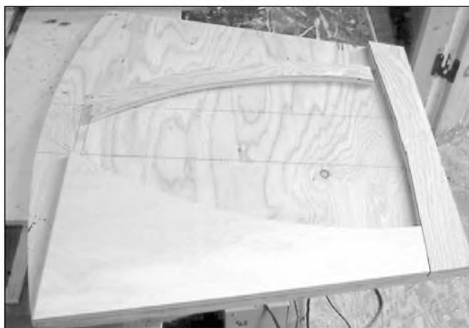
PHOTO 7: Checking brace patterns against cabinet top.
