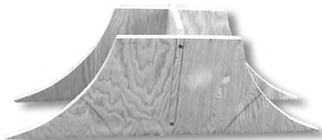
PHOTO 8: The throat horn sides and throat divider assembled.
