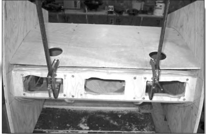
**PHOTO 15:** Attaching the mouth horn sheathing.
