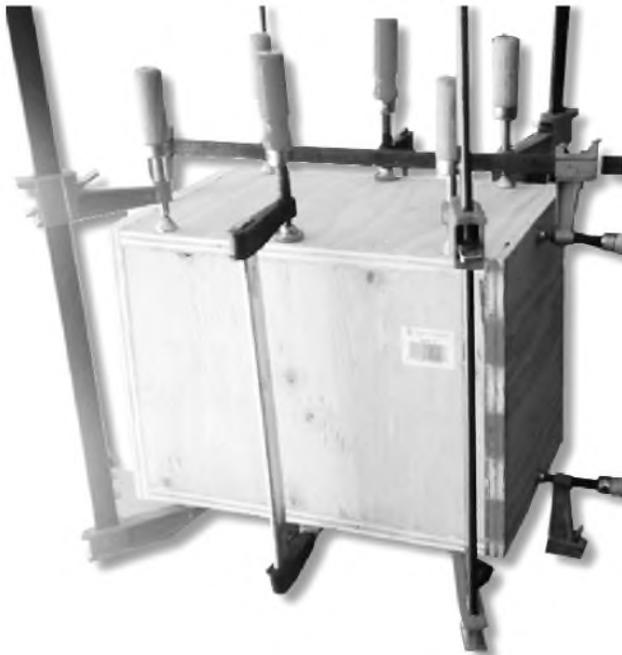
**PHOTO 1: The box glued and thoroughly clamped.**
