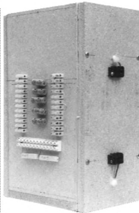
**PHOTO 2: Block and European-style connectors mounted on exterior of testing enclosure for ease of changing connections and components of network.**
