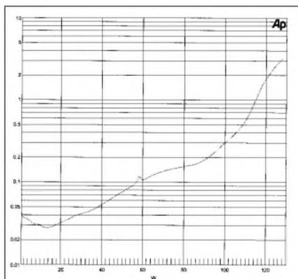
**FIGURE 7: THD versus power (input = 100Hz). All figures use load = 4Ω, with Astrodyne power supply.**
