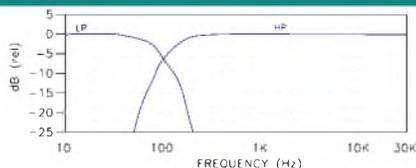
FIGURE 1: Crossover output response versus frequency.
