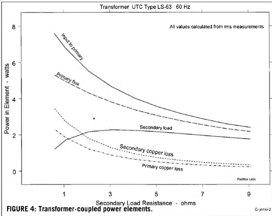
FIGURE 4: Transformer-coupled power elements.
