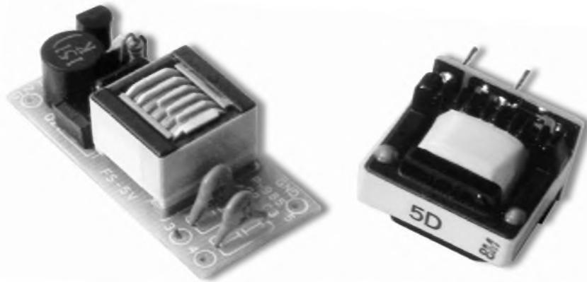
PHOTO 3: Left, JKL fluorescent lamp power module; right, Seiko EL-lamp power module.
