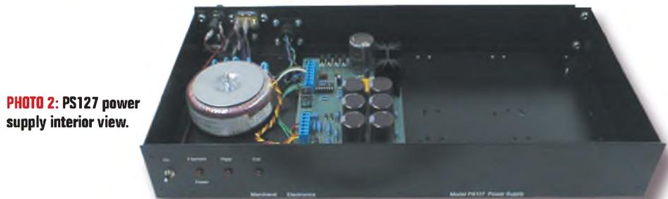
**PHOTO 2:** PS127 power supply interior view.
