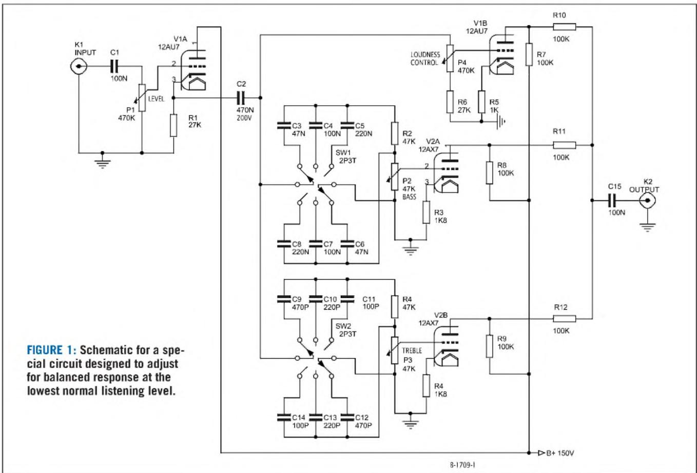
**FIGURE 1:** Schematic for a special circuit designed to adjust for balanced response at the lowest normal listening level.
