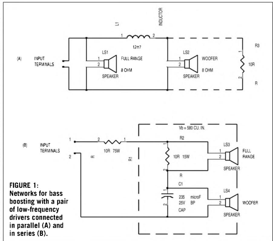
FIGURE 1: Networks for bass boosting with a pair of low-frequency drivers connected in parallel (A) and in series (B).
