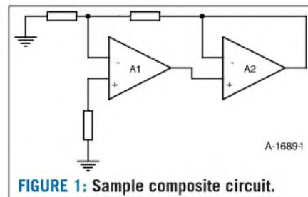
FIGURE 1: Sample composite circuit.
