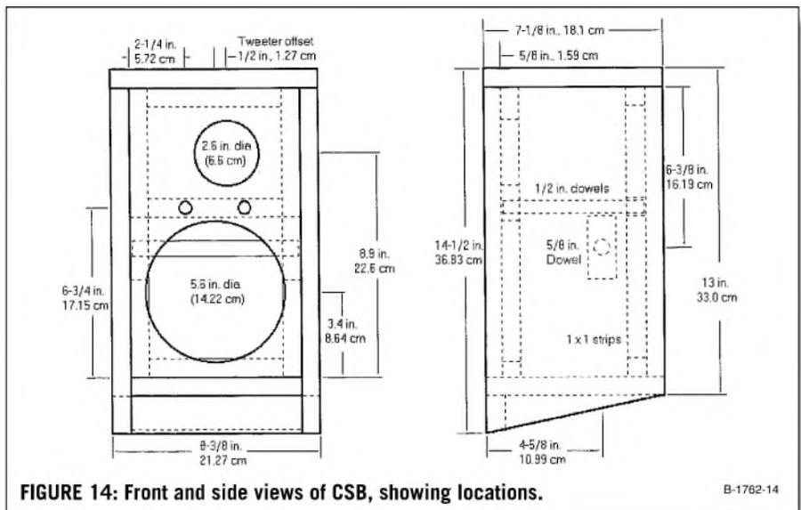
**FIGURE 14:** Front and side views of CSB, showing locations.
