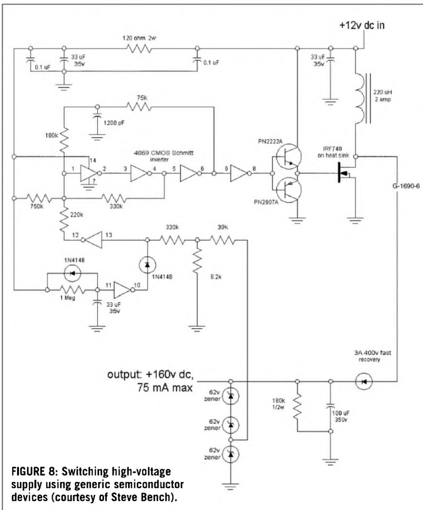
FIGURE 8: Switching high-voltage supply using generic semiconductor devices (courtesy of Steve Bench).
