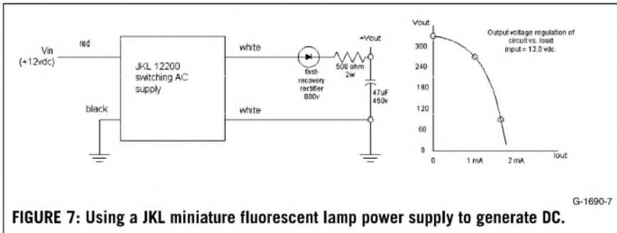
FIGURE 7: Using a JKL miniature fluorescent lamp power supply to generate DC.
