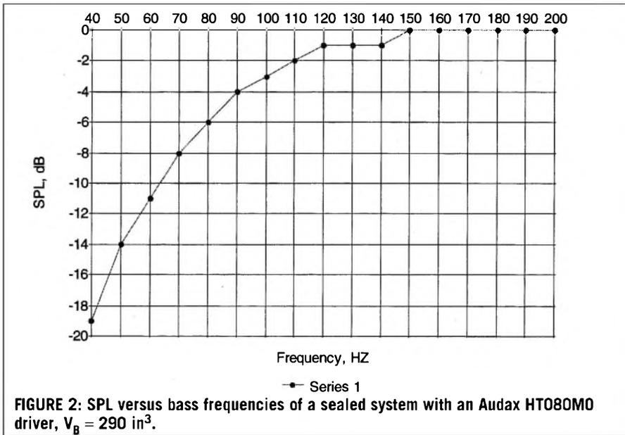
**FIGURE 2:** SPL versus bass frequencies of a sealed system with an Audax HT080MO driver,  $V_b = 290 \text{ in}^3$ .
