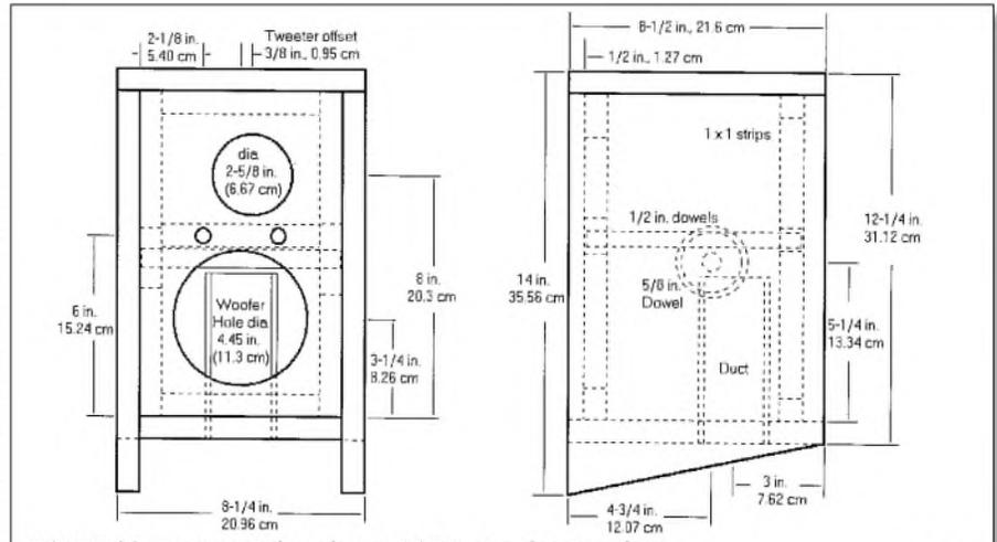
FIGURE 11: Front and side views of CSA, showing locations.
