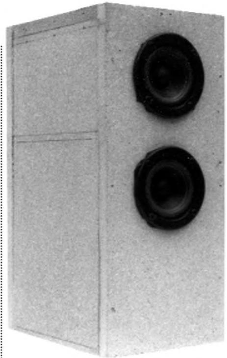
PHOTO 1: Testing enclosure with internal volume conforming to the golden ratio,  $W = 5.25"$ ,  $H = 14"$ ,  $D = 8"$ .
