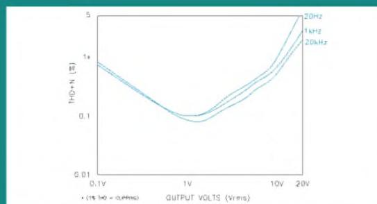
FIGURE 1: THD+N versus output power, CF mode.
