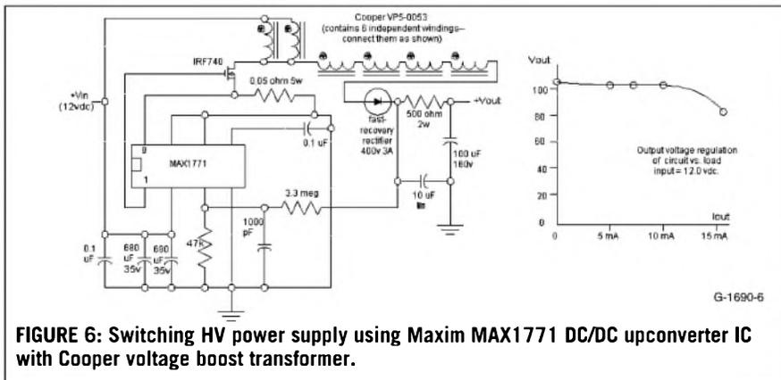
FIGURE 6: Switching HV power supply using Maxim MAX1771 DC/DC upconverter IC with Cooper voltage boost transformer.
