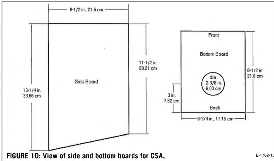
**FIGURE 10:** View of side and bottom boards for CSA.
