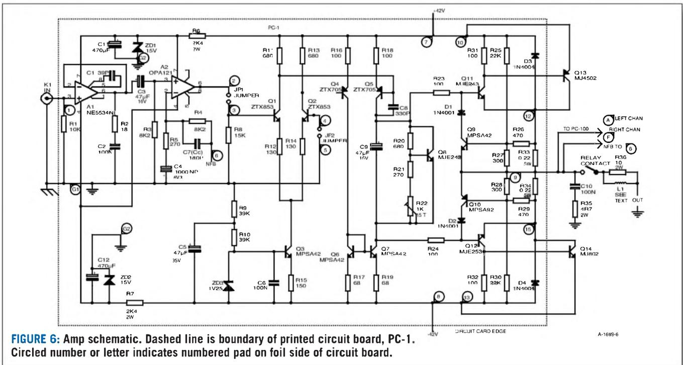
the best low-noise performance.<sup>3</sup> I would prefer it to be about an octave lower. Normally, it is possible to restrict bandwidth by using a small capacitor across the feedback resistor, but in this composite that space is already occupied by Cf. So I added a unity-gain, low-pass, active filter ahead of the composite.
