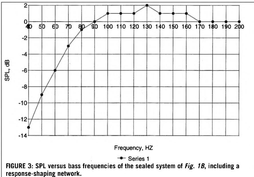
**FIGURE 3:** SPL versus bass frequencies of the sealed system of Fig. 1B, including a response-shaping network.
