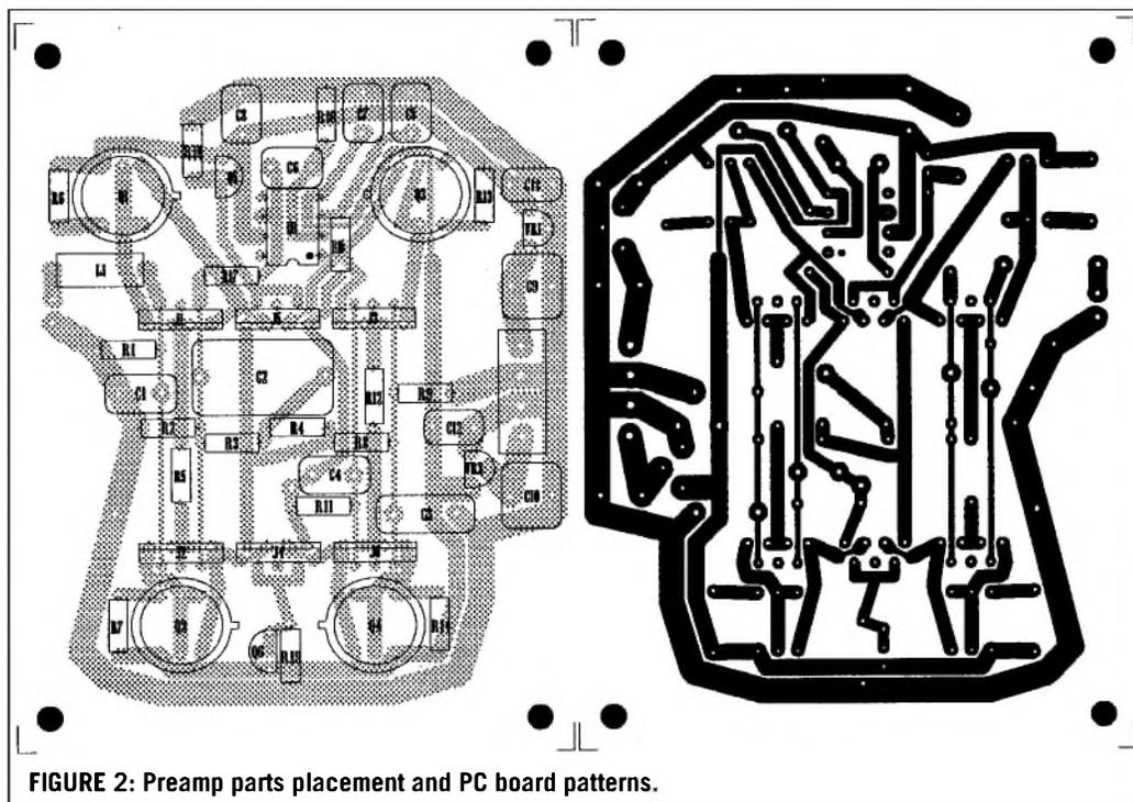
FIGURE 2: Preamp parts placement and PC board patterns.
