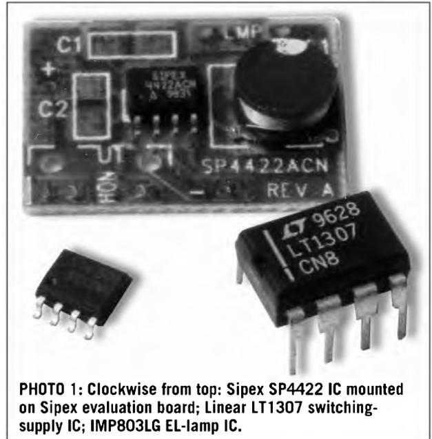
**PHOTO 1:** Clockwise from top: Sorex SP4422 IC mounted on Sorex evaluation board; Linear LT1307 switching supply IC; IMP803LG EL-lamp IC.
