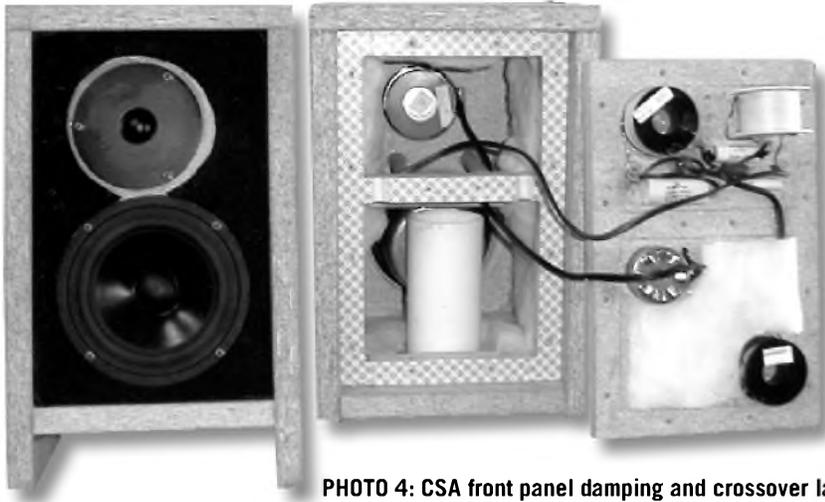
PHOTO 4: CSA front panel damping and crossover layout.
