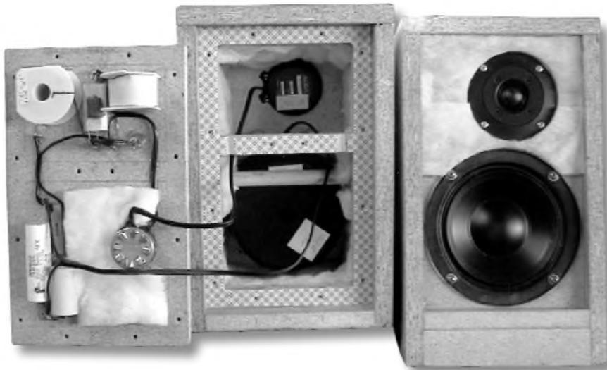
PHOTO 6: CSB front panel damping and crossover layout.
