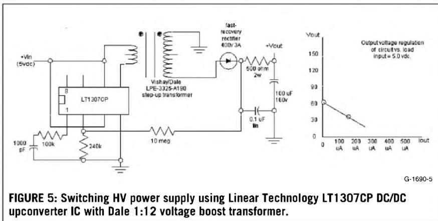
FIGURE 5: Switching HV power supply using Linear Technology LT1307CP DC/DC upconverter IC with Dale 1:12 voltage boost transformer.
