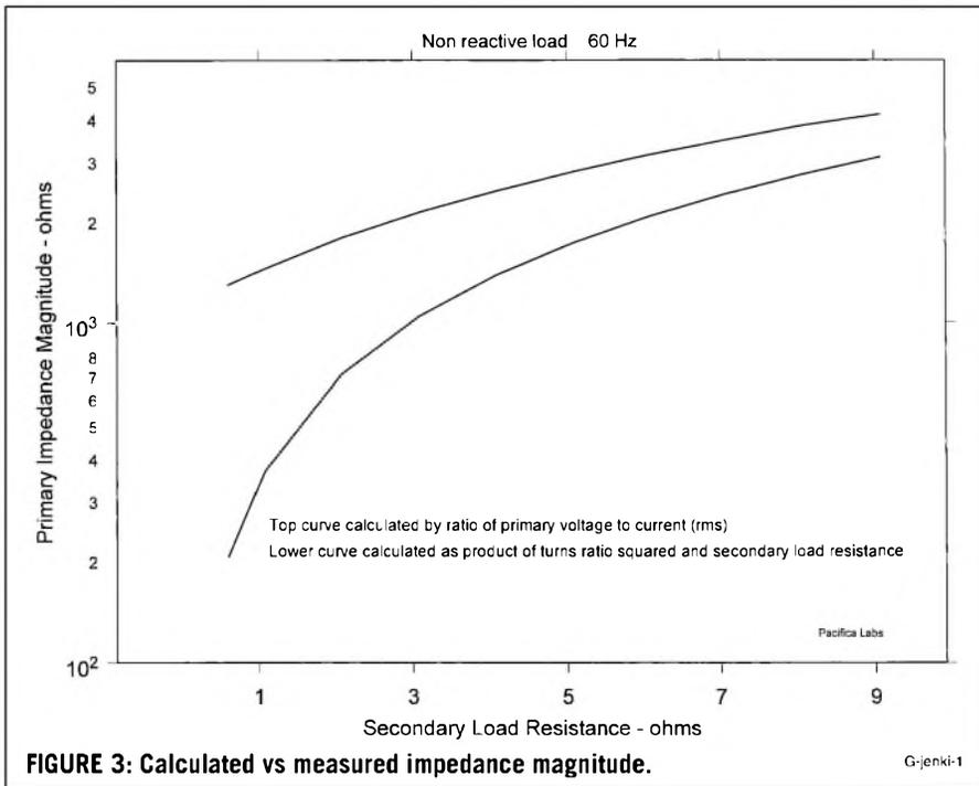
FIGURE 3: Calculated vs measured impedance magnitude.
