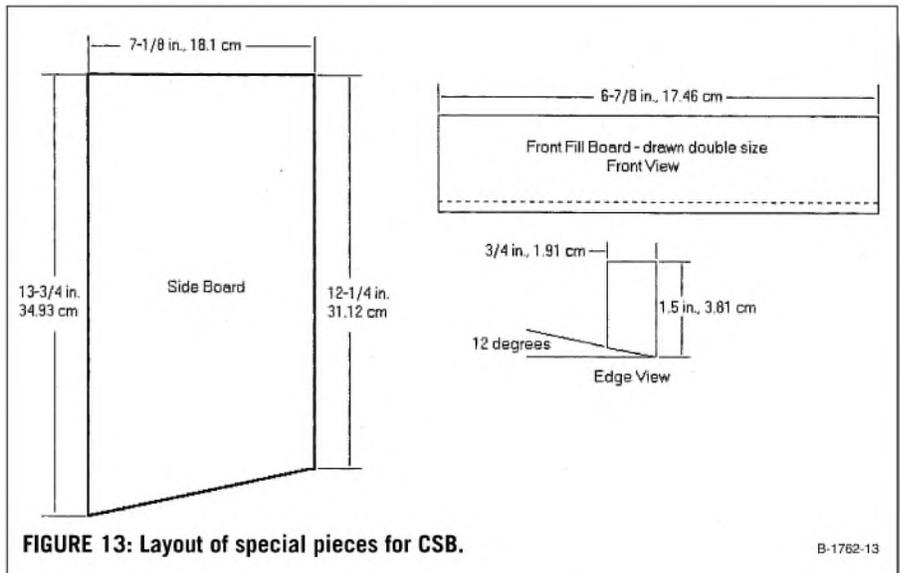
**FIGURE 13:** Layout of special pieces for CSB.
