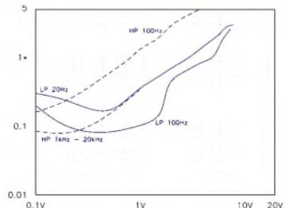
FIGURE 2: THD+N versus output voltage.
