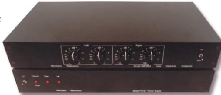
**PHOTO 1:** Crossover and power units stacked and connected.
