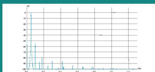
FIGURE 6: Spectrum of 50Hz sine wave, SRPP mode.
