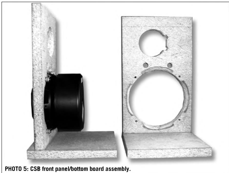
PHOTO 5: CSB front panel/bottom board assembly.
