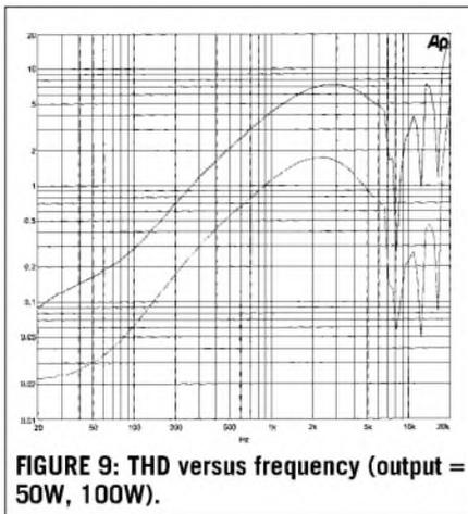
FIGURE 9: THD versus frequency (output = 50W, 100W).
