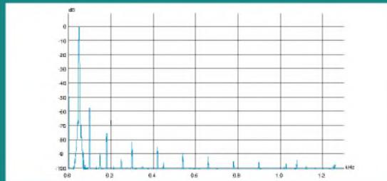
FIGURE 5: Spectrum of 50Hz sine wave, CF mode.
