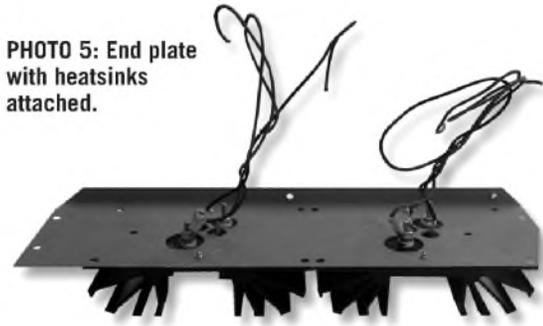
PHOTO 5: End plate with heatsinks attached.
