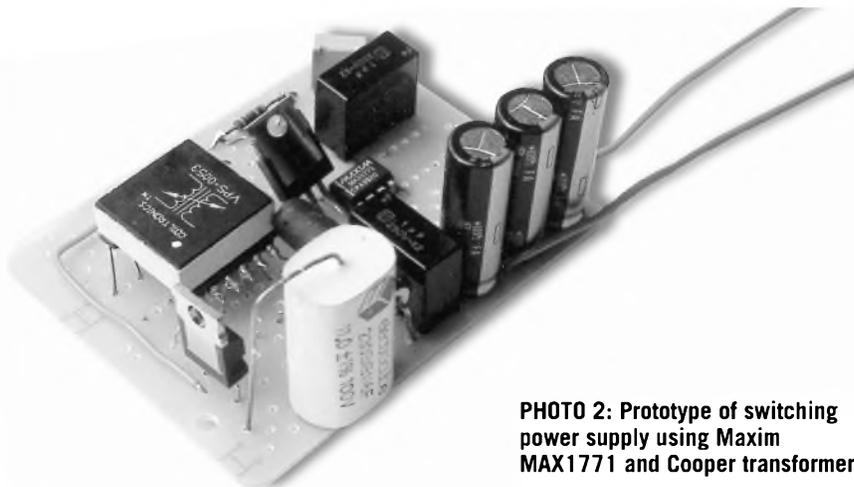
PHOTO 2: Prototype of switching power supply using Maxim MAX1771 and Cooper transformer.
