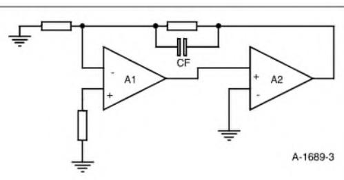
FIGURE 3: Composite amp circuit used for this project.
