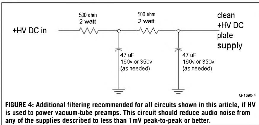
FIGURE 4: Additional filtering recommended for all circuits shown in this article, if HV is used to power vacuum-tube preamps. This circuit should reduce audio noise from any of the supplies described to less than 1mV peak-to-peak or better.
