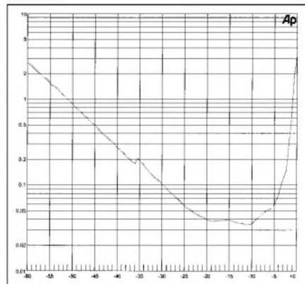
**FIGURE 8: THD versus input amplitude (input = 100Hz).**
