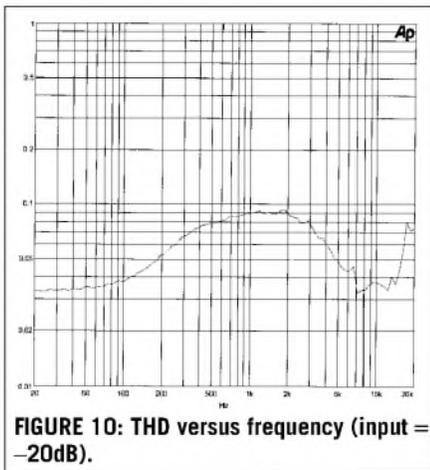
FIGURE 10: THD versus frequency (input = -20dB).
