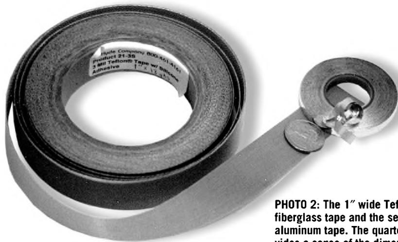
**PHOTO 2: The 1" wide Teflon-fiberglass tape and the sensing aluminum tape. The quarter provides a sense of the dimensions.**
