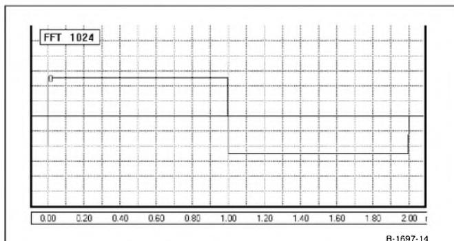
FIGURE 14: Simulated response to a 500Hz square-wave input.
