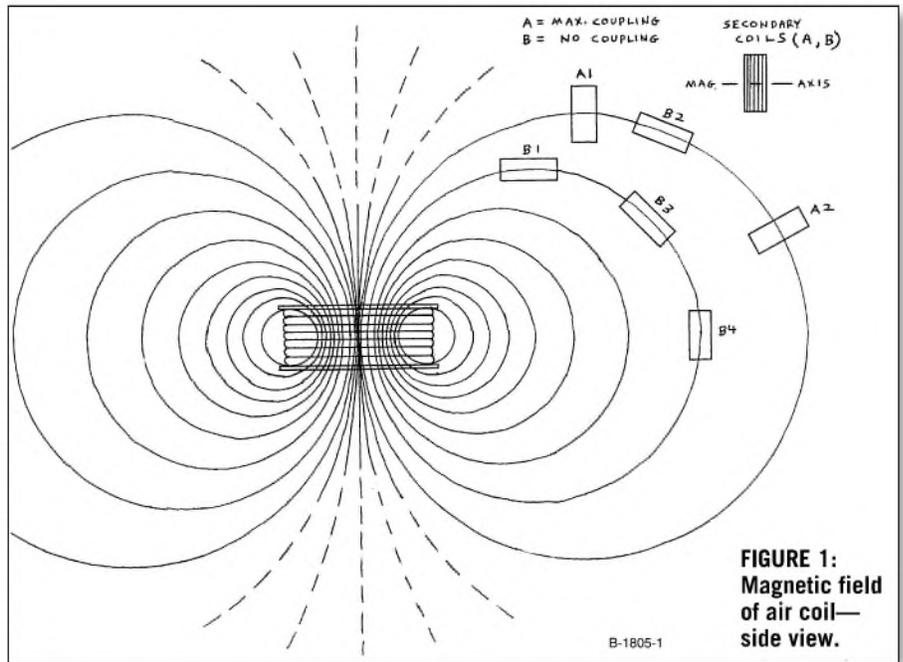
FIGURE 1: Magnetic field of air coil—side view.
