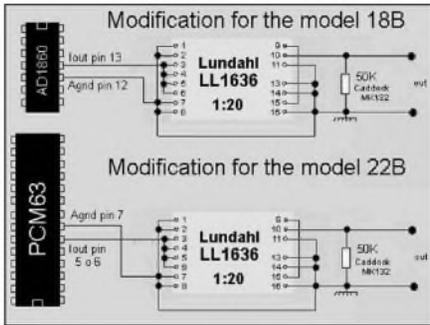
**FIGURE 5: Model 18B (top) and Model 22B modifications.**
