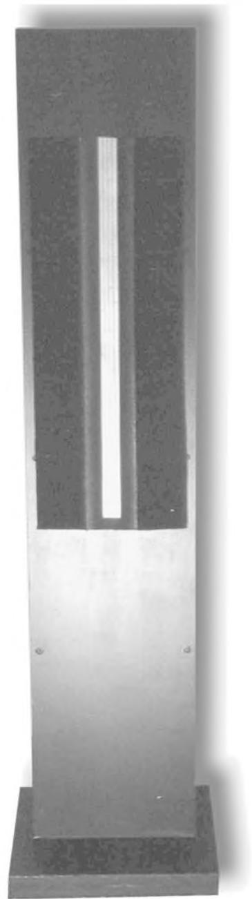
**PHOTO 1: Front view of ribbon speaker, finished with flat black paint.**
