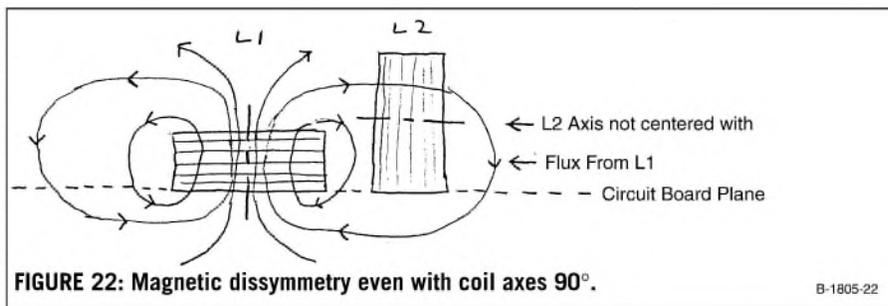
perpendicular to that of the other, and centered in the plane of the other. Each coil can be offset along its axis, or rotated in the plane of the other coil, without (ideally) causing any coupling.
