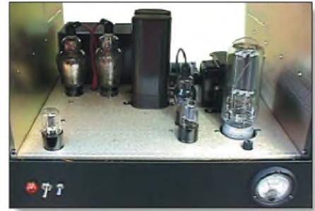
**PHOTO 5: Front view of amp showing front-panel controls. Power indicator, far left. Switch next to power indicator is the main power switch. Far-right switch is the 211 filament "operate/standby" switch. Right-hand side of panel, contains an optional current meter to monitor 211 output tube current.**
