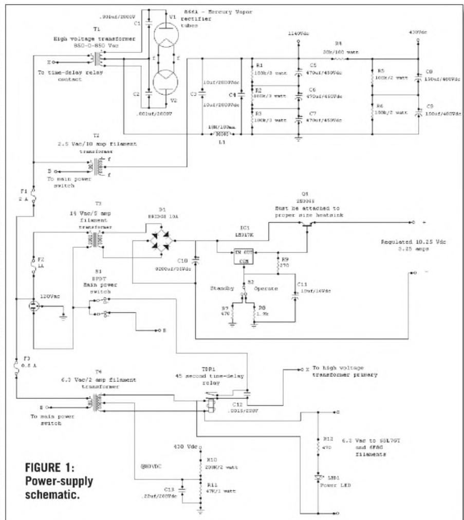
FIGURE 1: Power-supply schematic.
