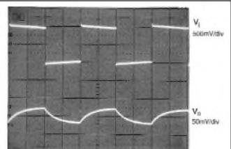
PHOTO 3:  $R_L = 50\Omega$ . Overdamped. HF  $F - 3dB = 4.7kHz = \frac{R_L}{2\pi L}$
