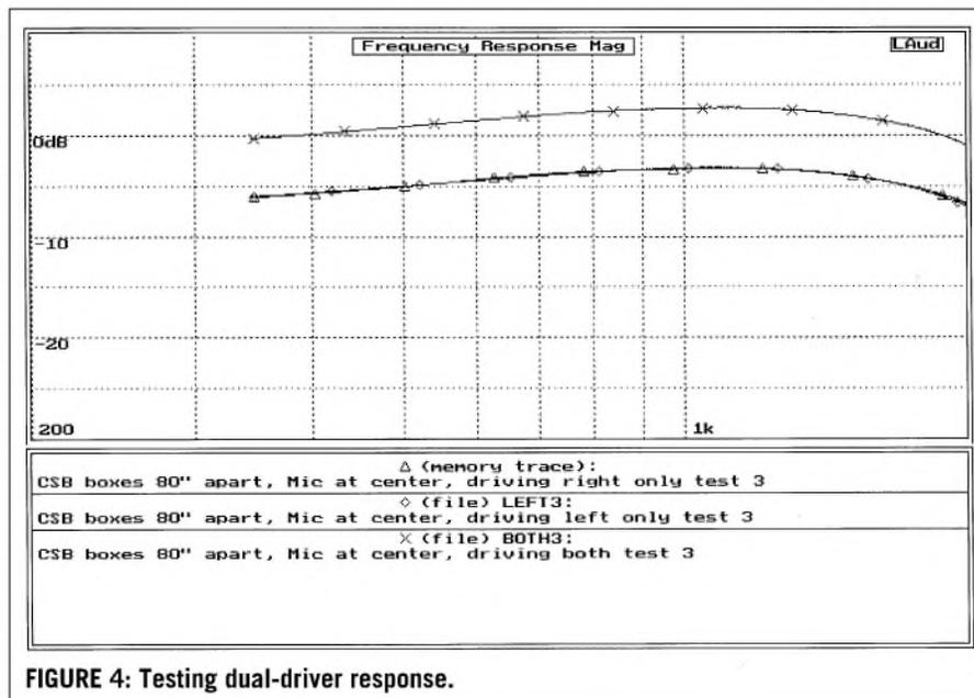
FIGURE 4: Testing dual-driver response.
