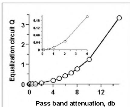
FIGURE 11:  $Q$  of required equalization circuit.
