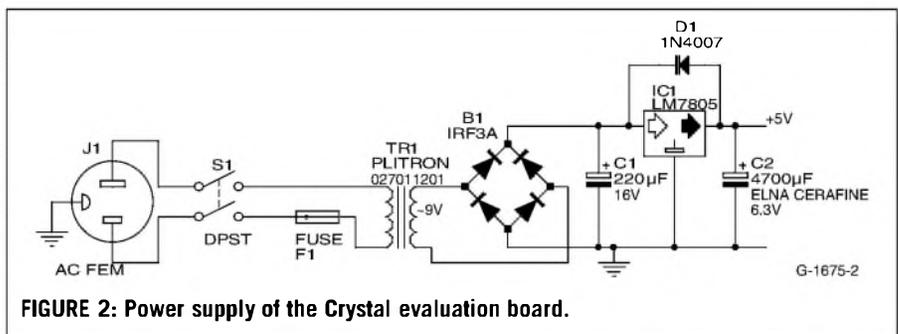
FIGURE 2: Power supply of the Crystal evaluation board.
