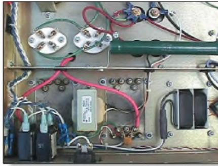
**PHOTO 4: Main high-voltage transformers and power-supply section. Mercury vapor tubes/sockets (upper-left corner). Voltage divider resistor for input tube section (big resistor in center). 211 filament transformer (bottom right).**
