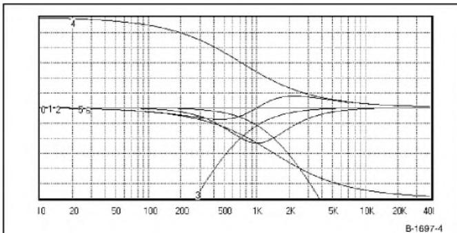
**FIGURE 4:** Summed second-order overlapped Linkwitz-Riley crossover at 1kHz following Lipshitz and Vanderkooy;<sup>2</sup> overlap parameter = 2; scale: 3dB/division.
