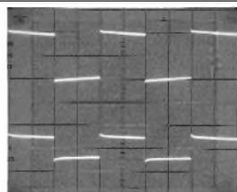
PHOTO 2:  $R_L = 1.8K\Omega$ . BW  $-3dB \approx 200Hz - 300kHz$ . LF  $F - 3dB = \frac{2.25\Omega}{2\pi L}$
