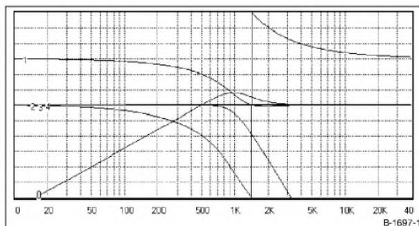
FIGURE 1: Constant-voltage crossover HP and LP sections using a third-order Butterworth low-pass filter; 0—HP amplitude response, 1—HP phase response; scale: 5dB/division.
