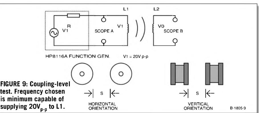
FIGURE 9: Coupling-level test. Frequency chosen is minimum capable of supplying 20V<sub>p-p</sub> to L1.
