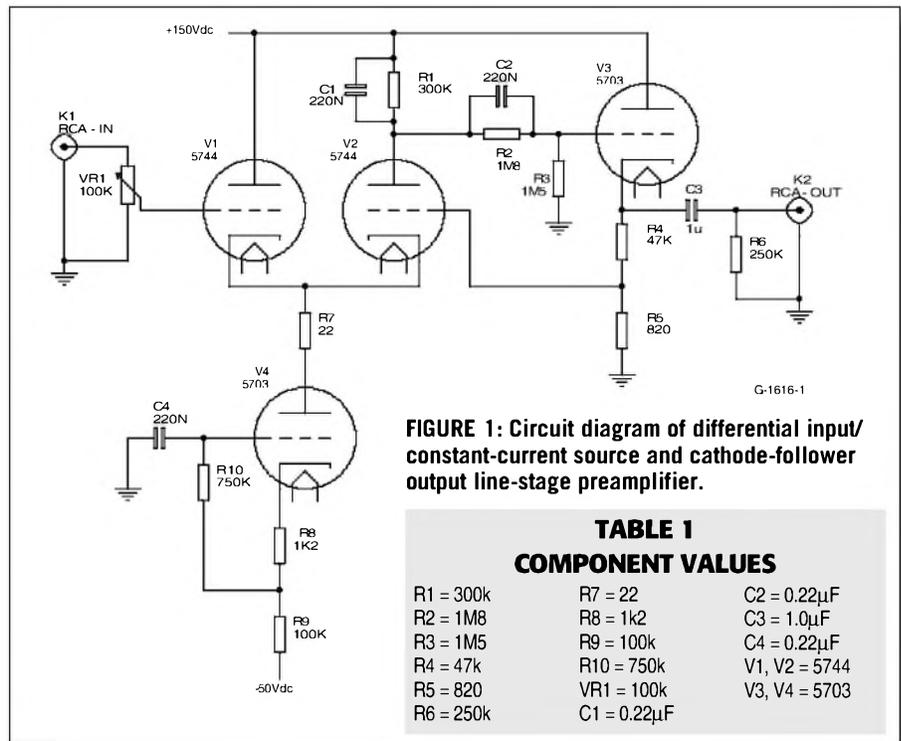
FIGURE 1: Circuit diagram of differential input/constant-current source and cathode-follower output line-stage preamplifier.
