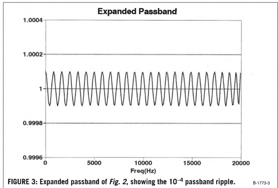
FIGURE 3: Expanded passband of Fig. 2, showing the  $10^{-4}$  passband ripple.
