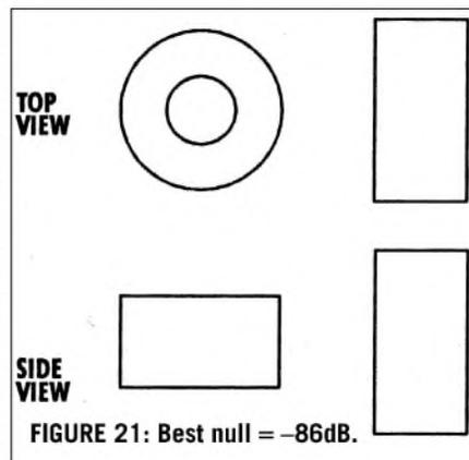
try possible. This configuration, with one degree of symmetry, is very sensitive to positional and angular offset. A 3° departure from perpendicularity of the true magnetic axes (not so symmetrical in real-world coils) resulted in 20dB more coupling than the best null. (To keep this in perspective, however, even with 3° error, and with coils touching, the coupling was only -60dB.)
