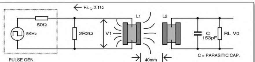
FIGURE 8: Pulse-response test. L1, L2 = 1.7mH ferrite (Madisound).  $R_{DC} = 0.15\Omega$ .
