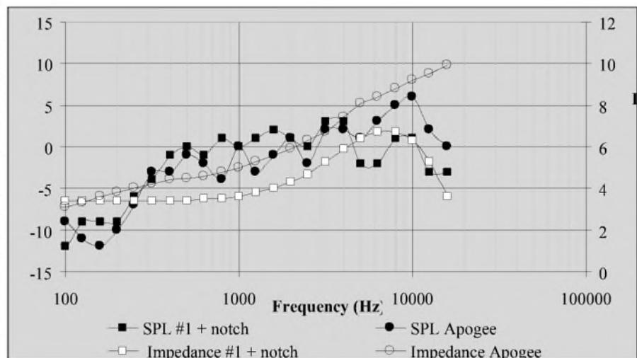
FIGURE 4: Frequency and impedance curves of ribbon speaker #1 and an Apogee Duetta MKII ribbon.
