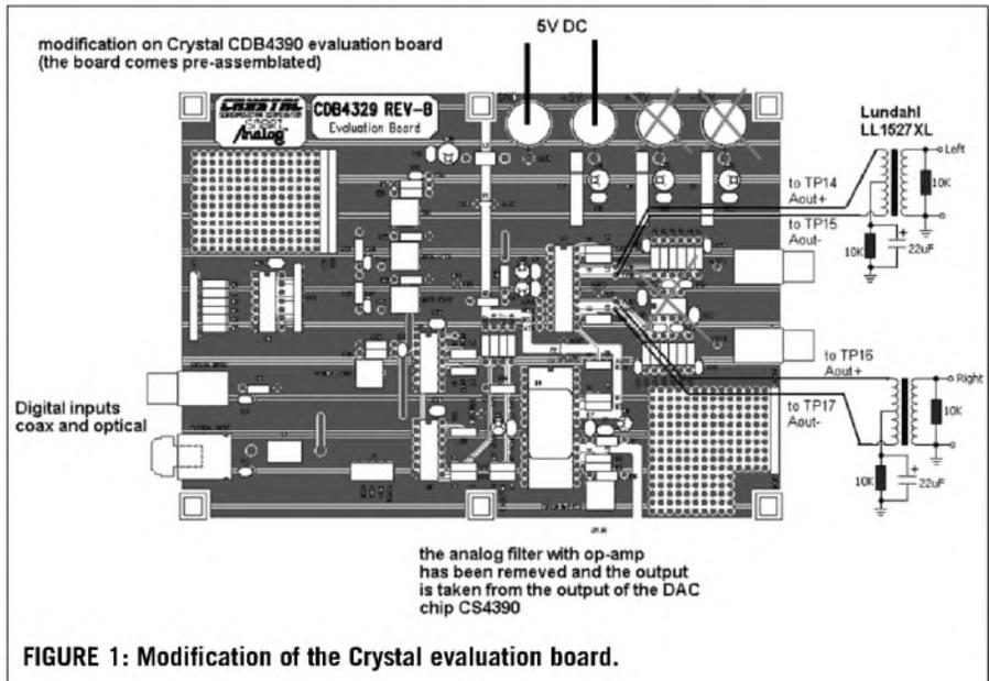
FIGURE 1: Modification of the Crystal evaluation board.
