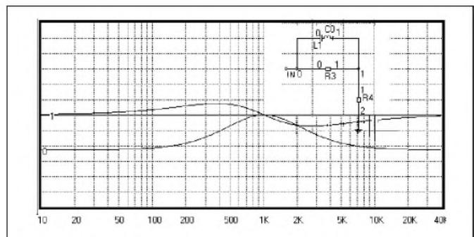
**FIGURE 7:** Passive equalization circuit for overlapped second-order Linkwitz-Riley crossover; scale: 3dB/division.
