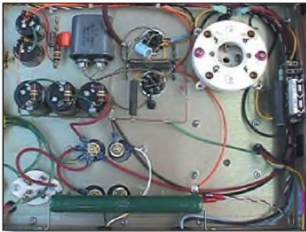
**PHOTO 6: Main amplifier section and part of the power supply. 211 tube (top right corner). 6SL7 and 6F8G input section (top center). Bias resistor and bypass capacitor mounted to side of chassis (right center).**
