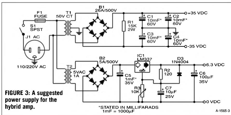
FIGURE 3: A suggested power supply for the hybrid amp.
