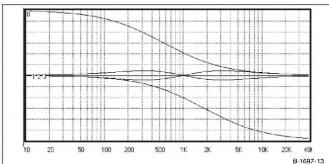
FIGURE 13: Phase response of unequalized HP and LP sections; summed unequalized phase; and phase of equalization circuit; scale: 30° per division.
