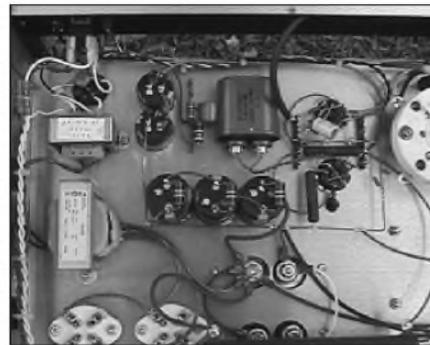
**PHOTO 2: High voltage/filament power-supply section for the 6SL7 and 6F8G. Time-delay relay (upper-left corner). Part of amplifier section (top-right corner).**
