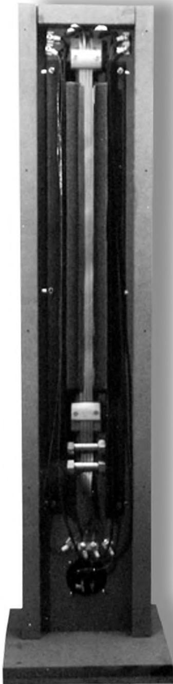
**PHOTO 4: The back plate of an assembled ribbon speaker. Note the two bolts and nuts below the lowest ribbon clamp for closing the magnet circuit.**
