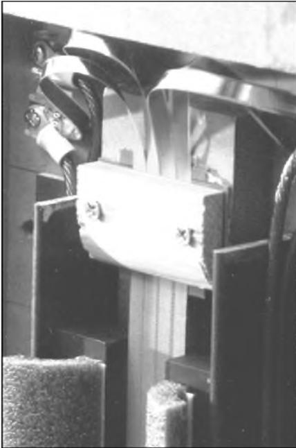
**PHOTO 3:** The ribbon clamp (center) and the termination of the foil using foil block connectors (used in security systems). Note how the ring terminals are easily attached onto these blocks. The lower part shows the quarter-round cylinder copper-pipe insulating foam used for decreasing diffraction.
