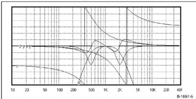
**FIGURE 5:** Summed third-order overlapped Butterworth crossover at 1kHz following Lipshitz and Vanderkooy;<sup>2</sup> overlap parameter = 4; scale: 3dB/division.
