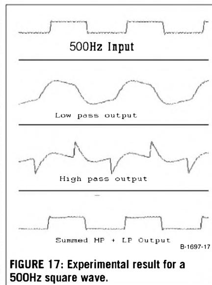
FIGURE 17: Experimental result for a 500Hz square wave.
