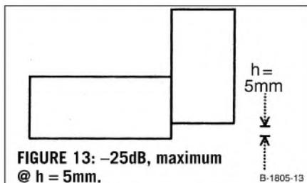
ties  $a_H$  and  $a_V$  are simply a practical measure of the -40dB coupling extension of an inductor, relative to its own maximum size dimension.
