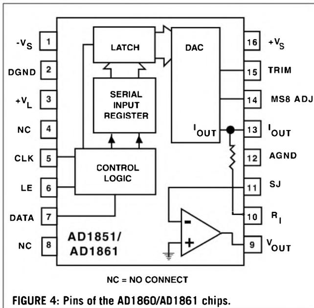
FIGURE 4: Pins of the AD1860/AD1861 chips.
