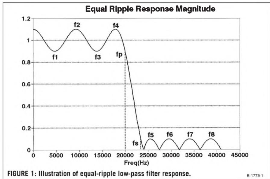
FIGURE 1: Illustration of equal-ripple low-pass filter response.
