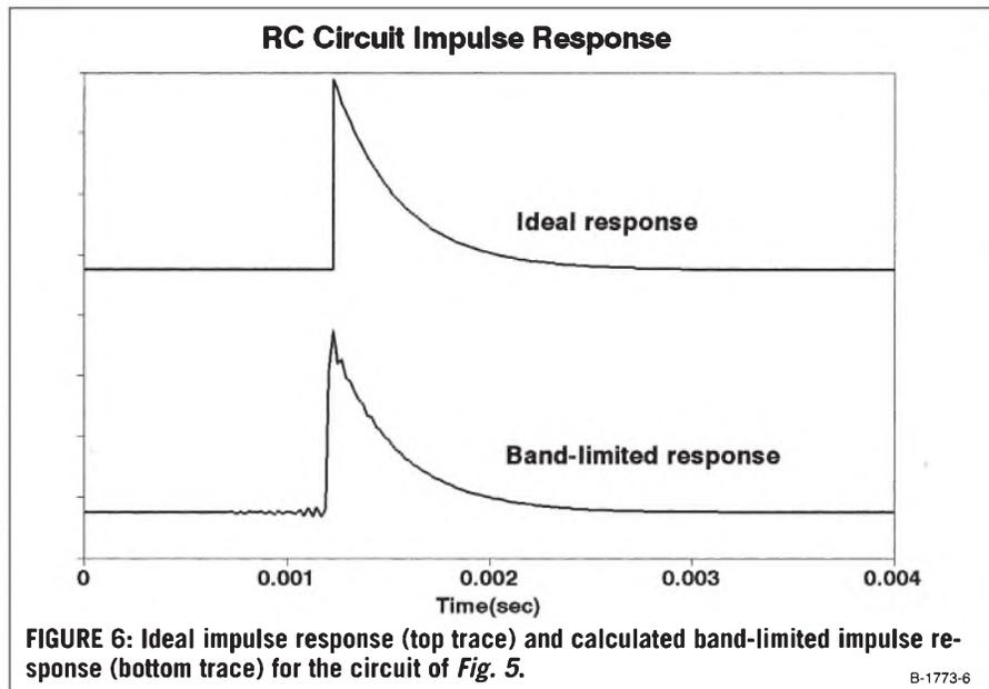
FIGURE 6: Ideal impulse response (top trace) and calculated band-limited impulse response (bottom trace) for the circuit of *Fig. 5*.
