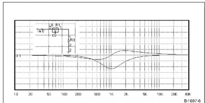
**FIGURE 6:** Trap circuit having a response similar to overlapped L-R crossover; scale: 3dB/division.
