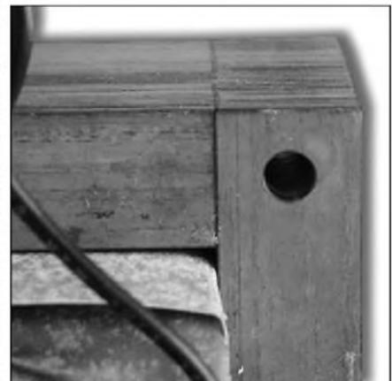
PHOTO 5: Close-up of the lamination gaps in an EI-core transformer.
