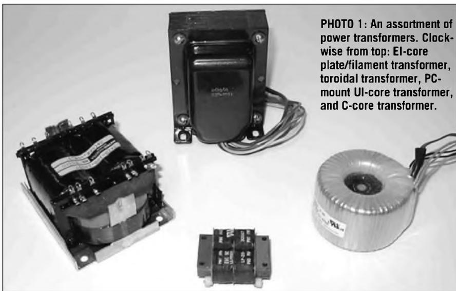
**PHOTO 1:** An assortment of power transformers. Clockwise from top: EI-core plate/filament transformer, toroidal transformer, PC-mount UI-core transformer, and C-core transformer.
