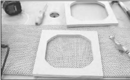
**PHOTO 5:** Here is the first pattern  $\frac{5}{8}$ " larger than driver. After two more repetitions, it will be  $\frac{1}{8}$ " larger.
