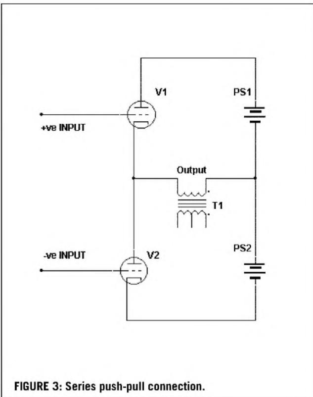
**FIGURE 3: Series push-pull connection.**
