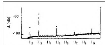
**A 2 × 200W amplifier. The sound is especially harsh and unpleasant, “metallic.” Note the effect of the “self-compensating” distortion circuit canceling out only the harmonics of even-numbered order.**
