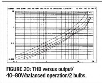
**FIGURE 20: THD versus output/40-80V/balanced operation/2 bulbs.**
