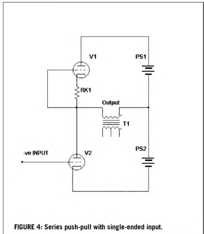
**FIGURE 4: Series push-pull with single-ended input.**
