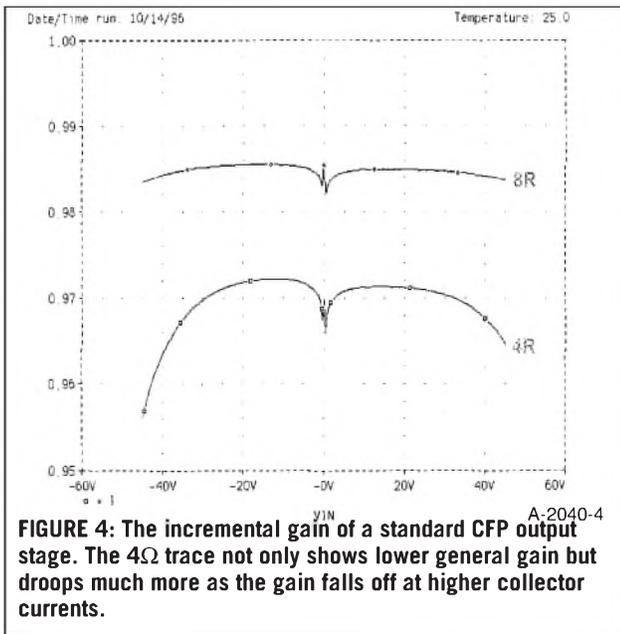
**FIGURE 4:** The incremental gain of a standard CFP output stage. The 4Ω trace not only shows lower general gain but droops much more as the gain falls off at higher collector currents.
