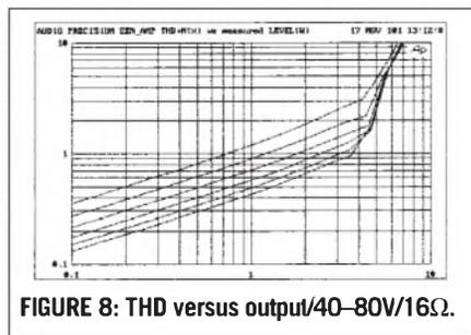
FIGURE 8: THD versus output/40–80V/16Ω.
