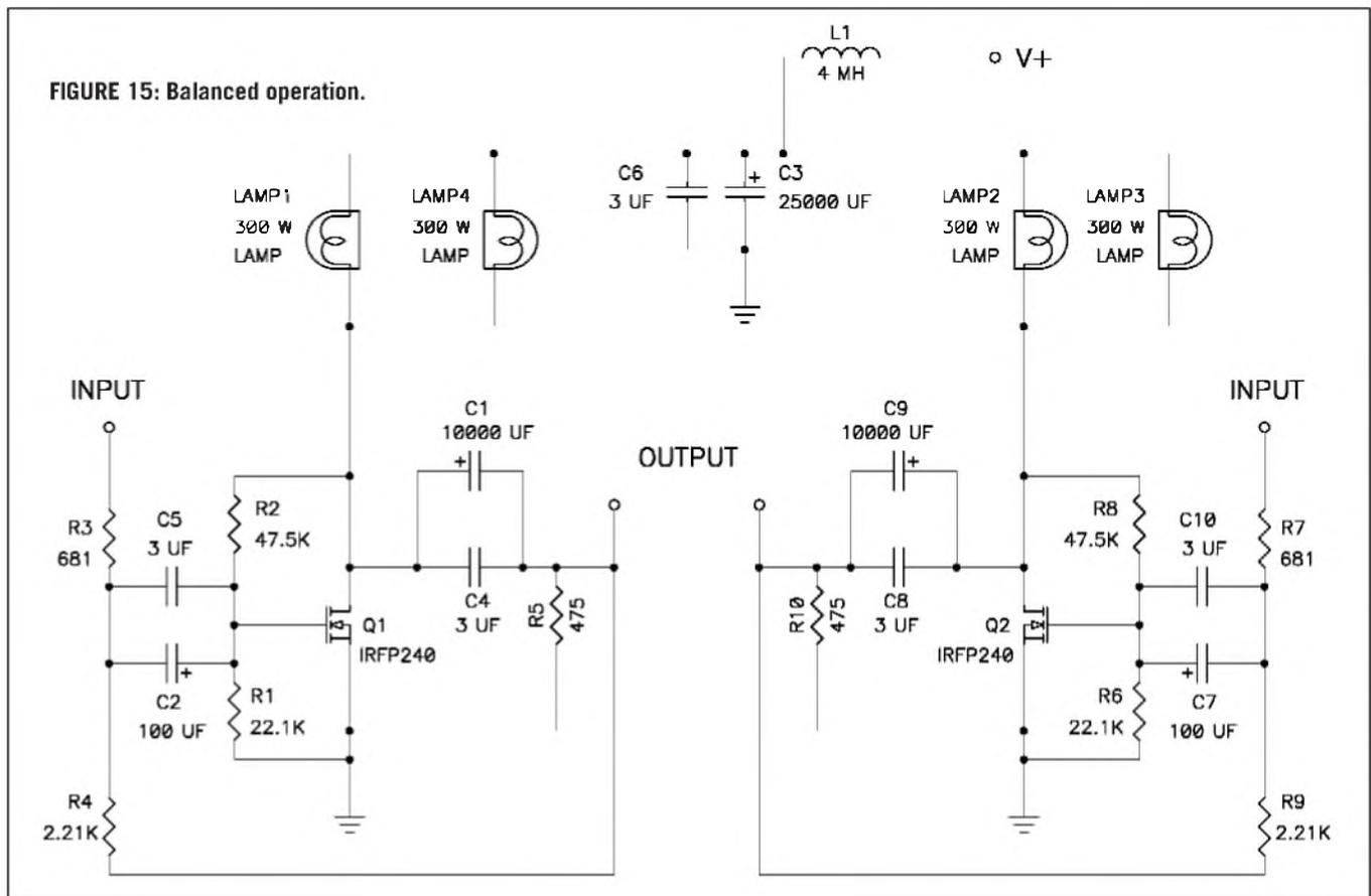
FIGURE 15: Balanced operation.
