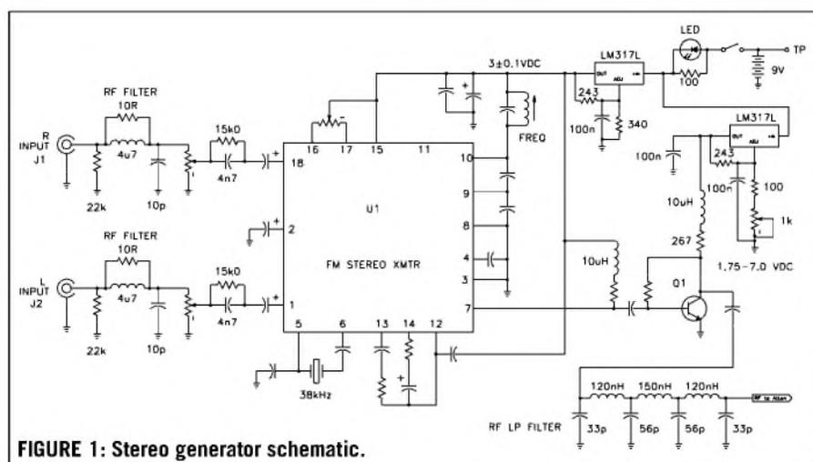
**FIGURE 1: Stereo generator schematic.**
