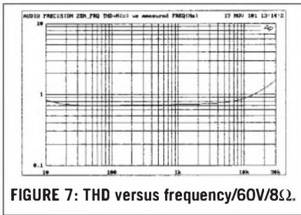
FIGURE 7: THD versus frequency/60V/8Ω.
