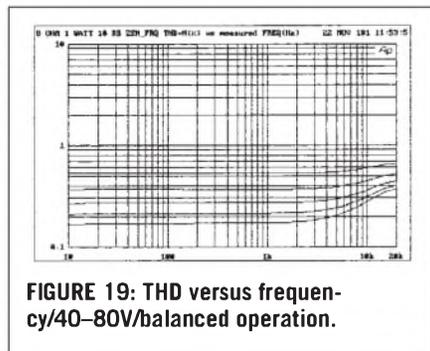
**FIGURE 19: THD versus frequency/40-80V/balanced operation.**
