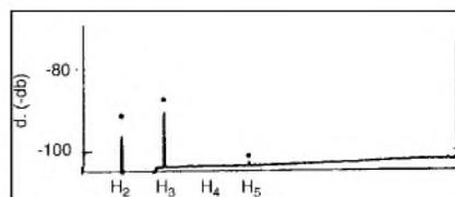
**A high-powered amplifier (400W) characterized by a sound that is dynamic, but very harsh and lacking in definition. Note the troubling predominance of H<sub>3</sub> (highly perceptible to the ear), the absence of H<sub>4</sub> (circuit of partial negative feedback in the power stage), and the absence of harmonics of high order (high overall rate of feedback).**
