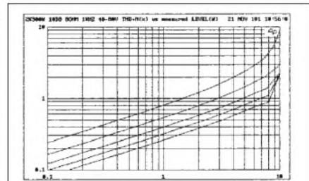
FIGURE 10: THD versus output/40–80V/IRFP040.
