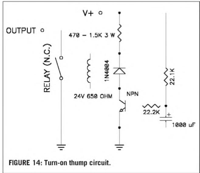
FIGURE 14: Turn-on thump circuit.
