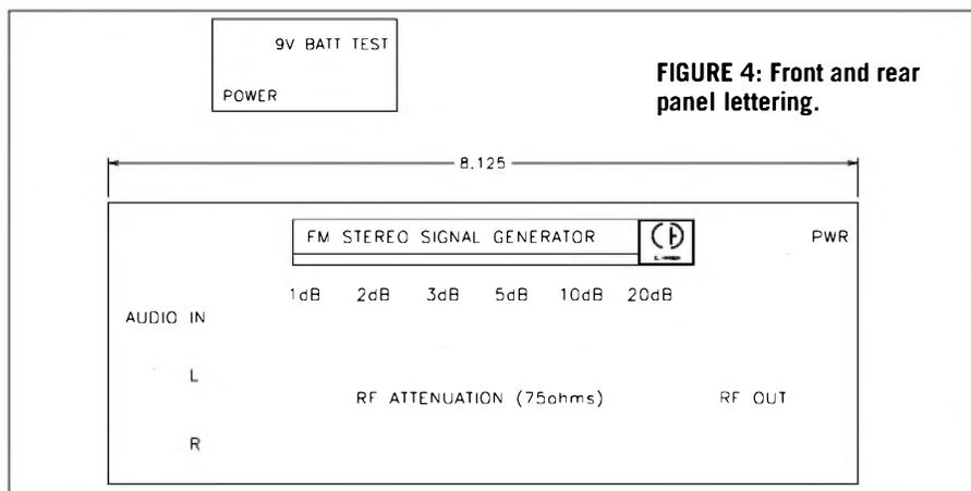
**FIGURE 4: Front and rear panel lettering.**
