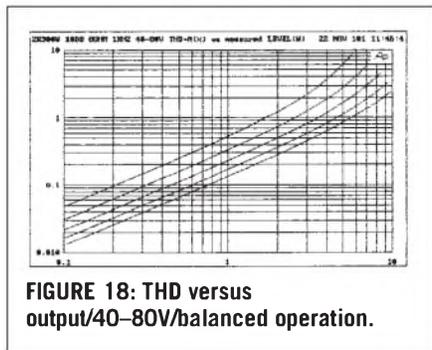
**FIGURE 18: THD versus output/40-80V/balanced operation.**
