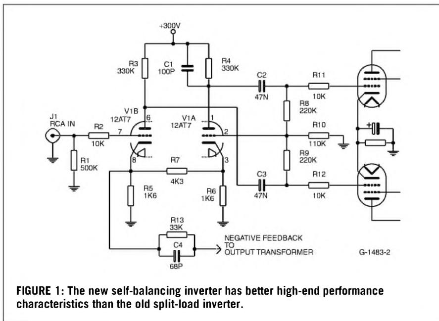
phase” inverter.<sup>4</sup> This circuit (*Fig. 1*) allows the original style for the input of the negative-feedback signal to remain, and also retains the same plate and cathode-biasing scheme.
