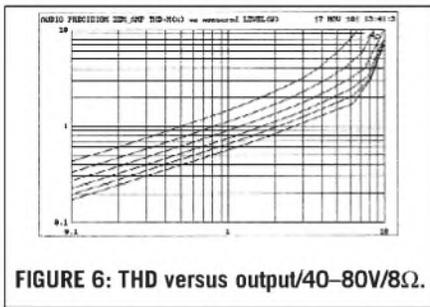
FIGURE 6: THD versus output/40–80V/8Ω.
