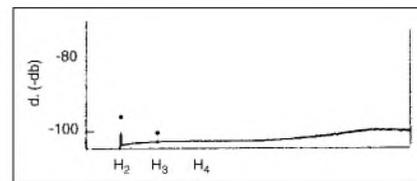
**A Class-A amplifier of 2 × 50W. Renowned for its musicality and its exemplary definition. Note the regular gradation, in which the top part is masked by the background noise (−100dB).**
