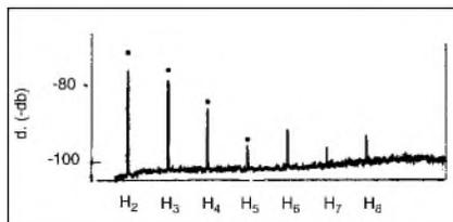
**A 2 × 30W amplifier, moderately priced but having good musicality. Note the presence of the principal harmonics, the presence of H<sub>6</sub> and H<sub>8</sub>, predominating slightly in comparison to the harmonics of odd-numbered order.**
