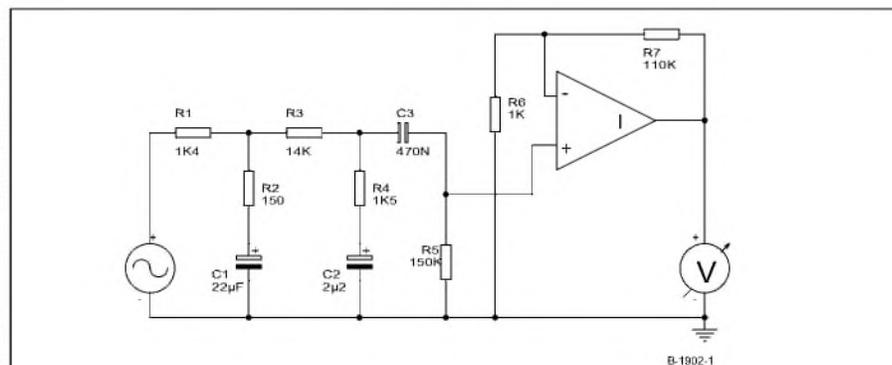
**FIGURE 1:** Using a small cabinet, incorporating a rigid-coned speaker and mounted against a wall, offers many benefits over traditional bass enclosures. The drawback is that such a speaker needs considerably more power as frequency falls. This filter provides boost rising to 20dB at 15Hz.
