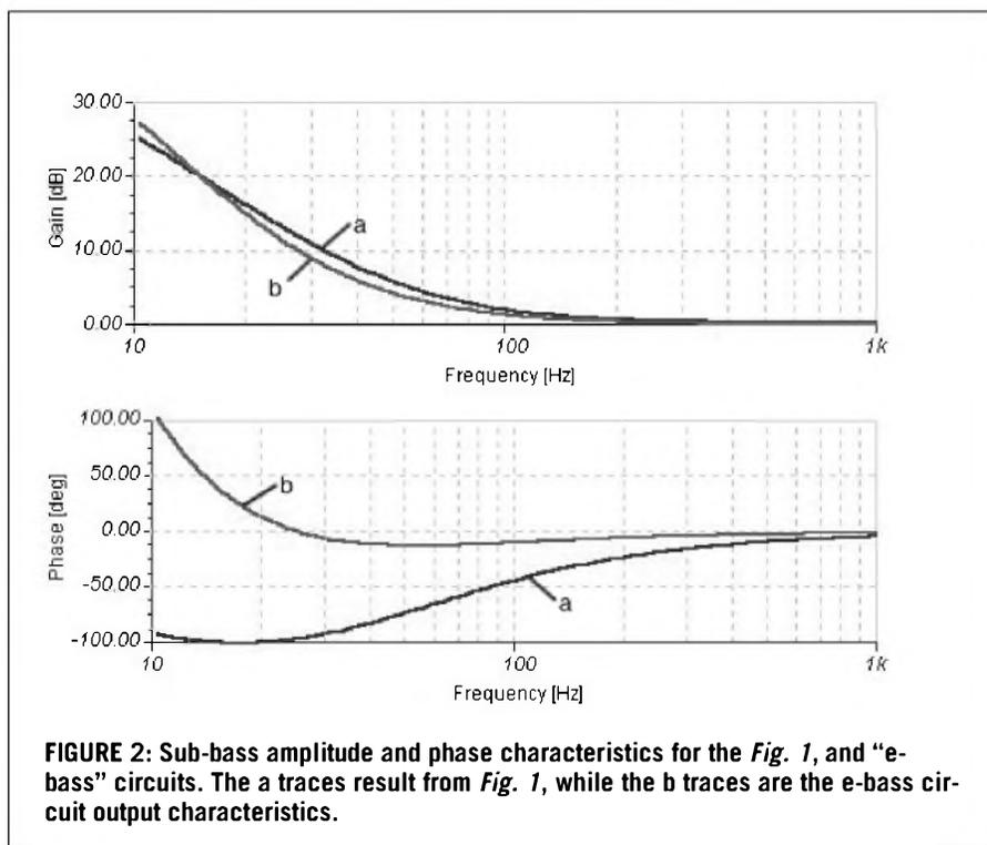
**FIGURE 2:** Sub-bass amplitude and phase characteristics for the Fig. 1, and “e-bass” circuits. The a traces result from Fig. 1, while the b traces are the e-bass circuit output characteristics.
