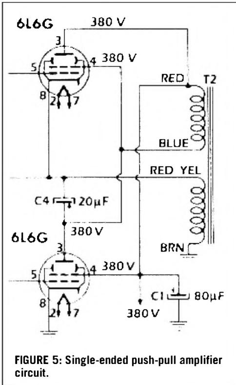
**FIGURE 5: Single-ended push-pull amplifier circuit.**
