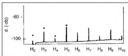
**A high-powered amplifier (2 × 300W) operating in Class B. Note the absence of harmonic 2 and the predominance of the harmonics of odd-numbered order. The sound, a little more defined than that of the 400W amplifier, seems subjectively as if “shifted” toward the top of the spectrum. In Class B, the origin of these flaws seems to be the presence of several zener diodes and imperfect complementary transistors.**
