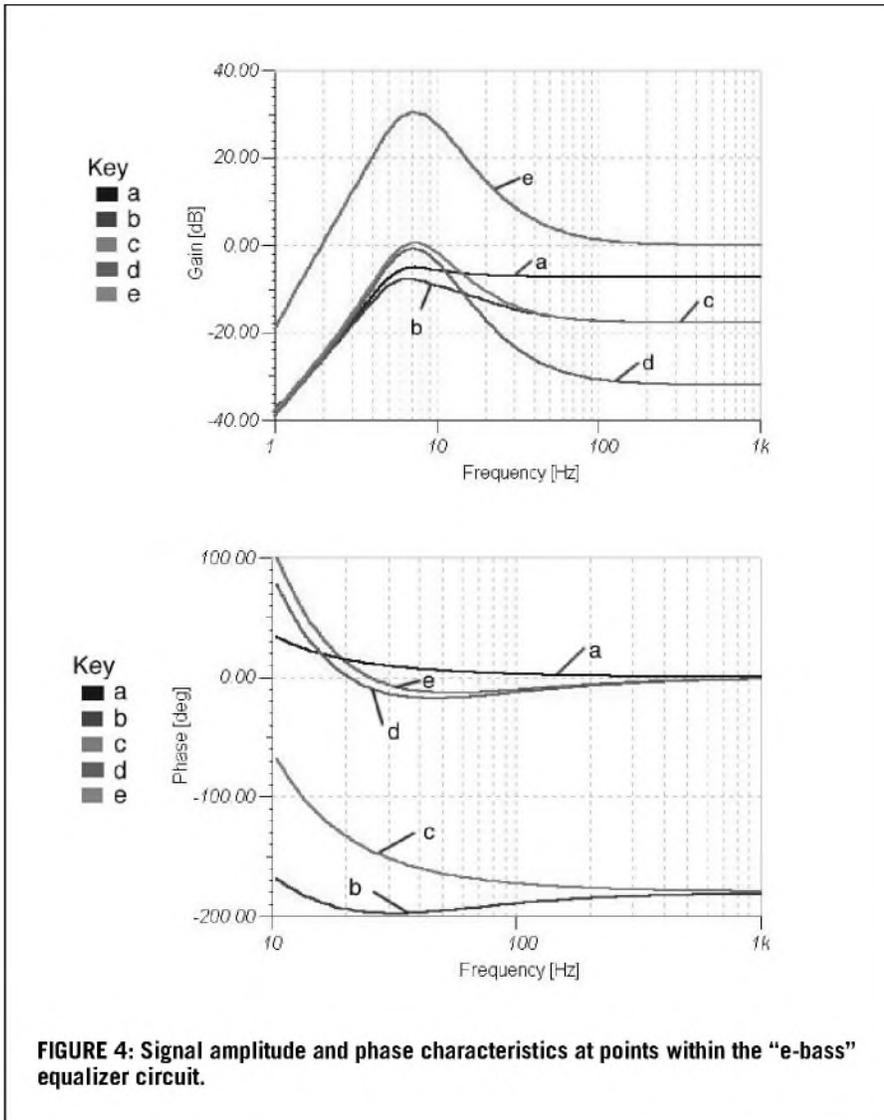
**FIGURE 4: Signal amplitude and phase characteristics at points within the "e-bass" equalizer circuit.**
