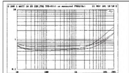
FIGURE 11: THD harmonic distortion versus frequency/60V (see text).
