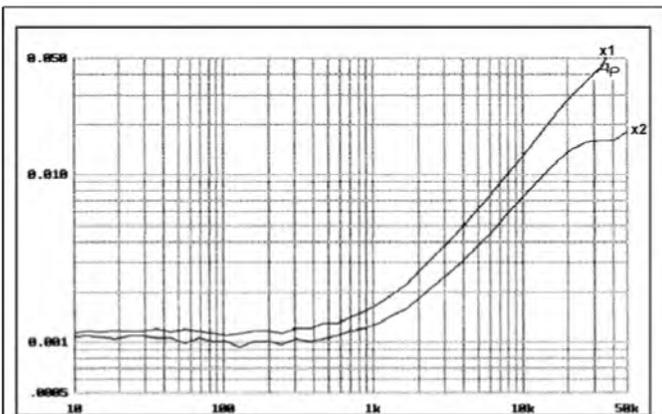
FIGURE 6: 4 $\Omega$  distortion is reduced by 1.9 $\times$  upon doubling standard (MJ15024/15025) output transistors. 30W/8 $\Omega$ .
