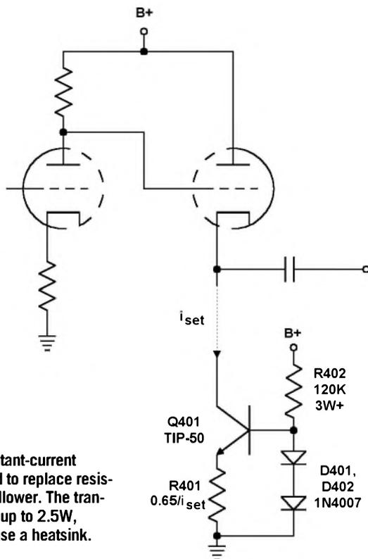
**FIGURE 20: Constant-current source, designed to replace resistor in cathode follower. The transistor dissipates up to 2.5W, worse case, so use a heatsink.**
