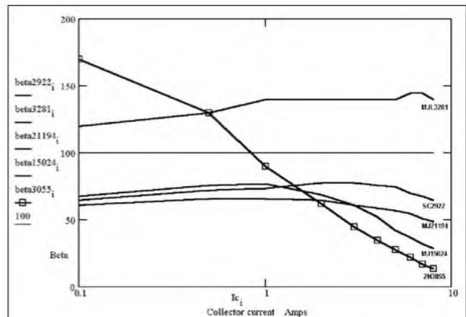
FIGURE 7: Power transistor beta falls as collector current increases. Data points shown on 3055 curve (from manufacturers' data sheets).
