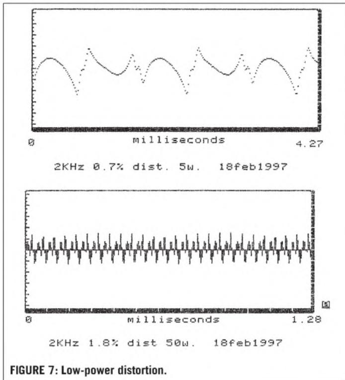
FIGURE 7: Low-power distortion.
