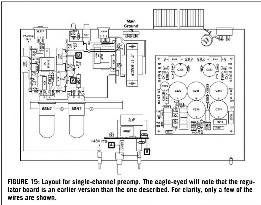
**FIGURE 15:** Layout for single-channel preamp. The eagle-eyed will note that the regulator board is an earlier version than the one described. For clarity, only a few of the wires are shown.
