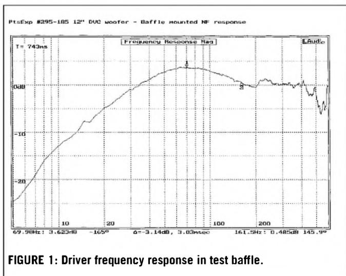
**FIGURE 1: Driver frequency response in test baffle.**
