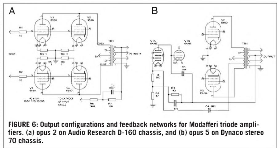
**FIGURE 6: Output configurations and feedback networks for Modafferi triode amplifiers. (a) opus 2 on Audio Research D-160 chassis, and (b) opus 5 on Dynaco stereo 70 chassis.**
