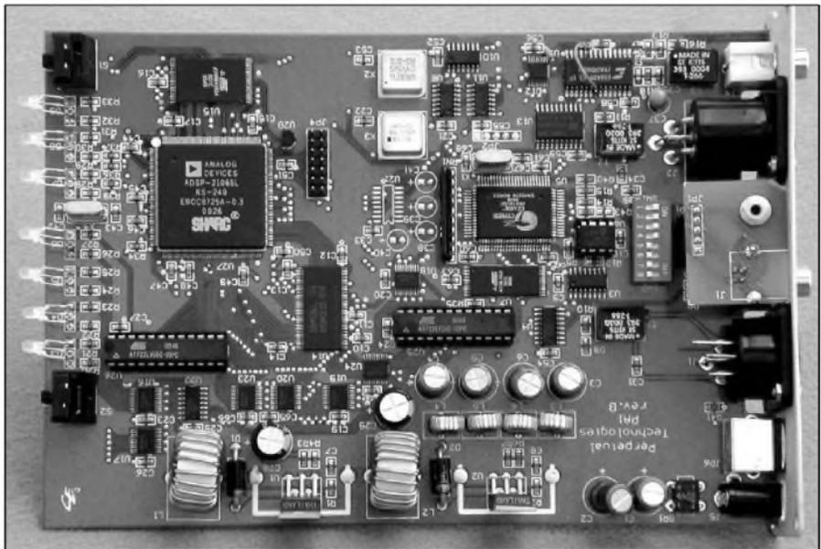
**PHOTO 2:** PC board for the P-1A. Analog Devices' ADSP-21056L (upper left) is the heart of the digital signal processing used for loudspeaker correction. Cirrus Logic's CS8420 sampling rate converter (upper right) upsamples all digital inputs to 96kHz.
