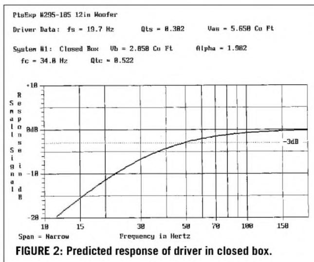
**FIGURE 2: Predicted response of driver in closed box.**
