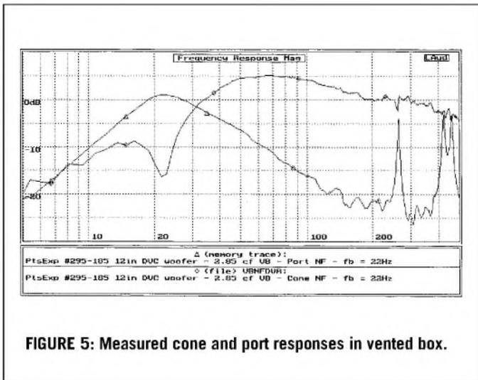
FIGURE 5: Measured cone and port responses in vented box.
