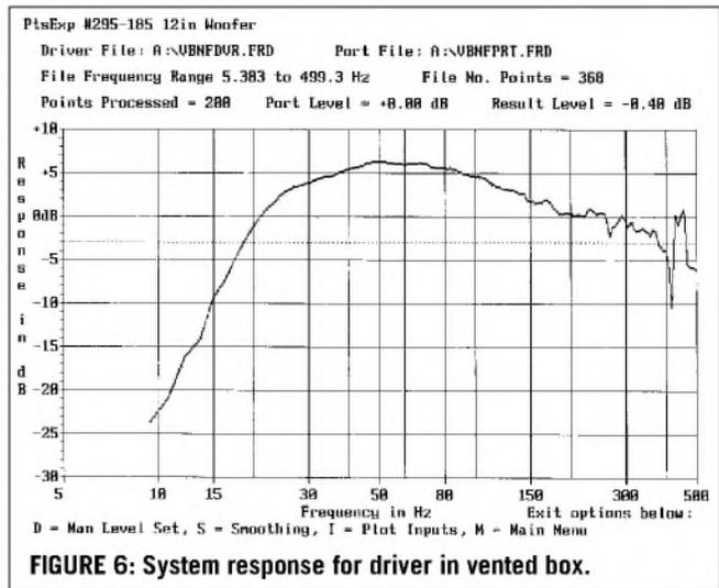
FIGURE 6: System response for driver in vented box.
