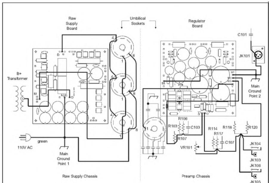
**FIGURE 16: Grounding scheme; ground connections shown as heavy lines. Each channel has a single main grounding point, connected to the chassis. Note that VR101's ground connects to the second stage's input resistors, not directly to ground. R120 and JK105–106 are used only in the double-output design.**
