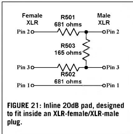
**FIGURE 21: Inline 20dB pad, designed to fit inside an XLR-female/XLR-male plug.**
