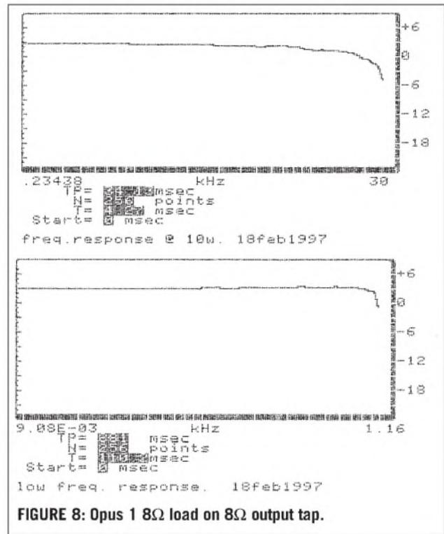
FIGURE 8: Opus 1 8Ω load on 8Ω output tap.
