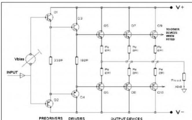
FIGURE 12: The triple-EF output stage, using multiple output devices with individual emitter resistors. Shown for N=3; i.e., three output devices.
