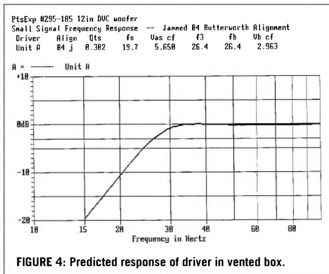
**FIGURE 4: Predicted response of driver in vented box.**
