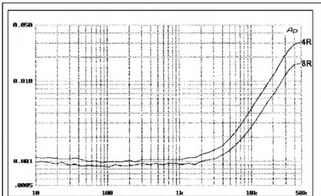
FIGURE 8: THD at 40W/8Ω and 80W/4Ω with single 3281/1302 devices.
