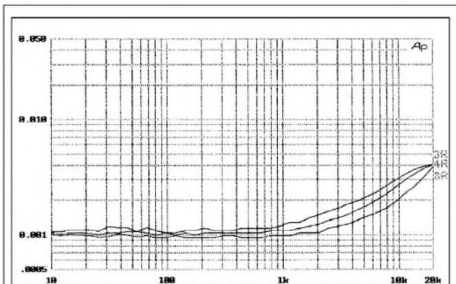
FIGURE 11: Distortion for 3, 4, and  $8\Omega$  load, double 3281/1302 devices. Power as Fig. 10.
