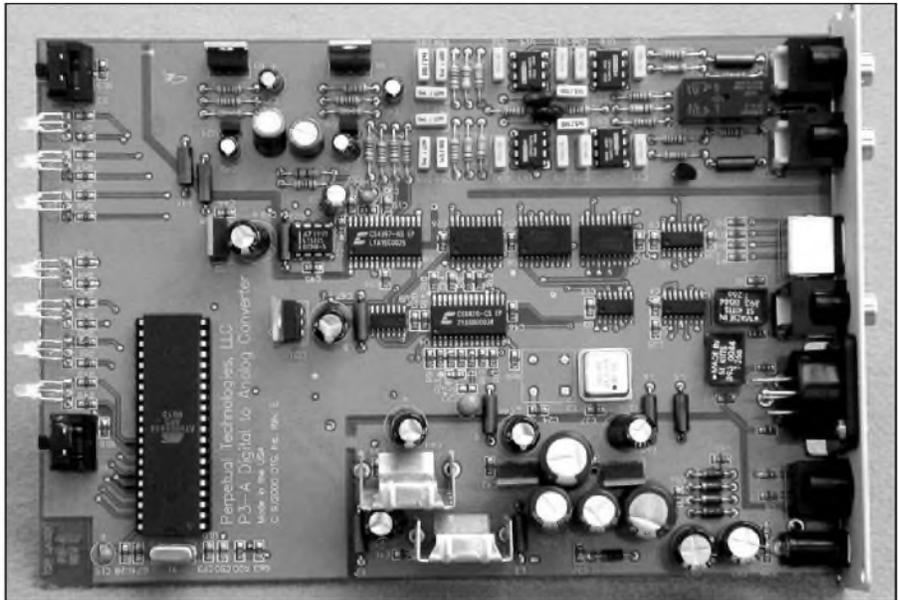
**PHOTO 1:** PC board for the P-3A D/A converter. This product also contains a CS8420 sampling rate converter, along with Cirrus Logic's CS4397 combination digital filter and D/A converter chip. Analog circuitry consists of four Burr-Brown OPA134 op-amps.
