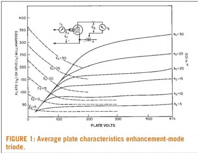
**FIGURE 1: Average plate characteristics enhancement-mode triode.**
