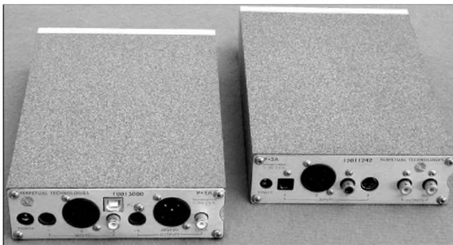
PHOTO 4: Rear views of the P-1A (left) and P-3A. The P-1A includes S/PDIF, AES/EBU, and Audio Alchemy-style I<sup>2</sup>S inputs and outputs. The P-3A includes the same three inputs, plus a Toslink optical input, along with stereo audio outputs.
