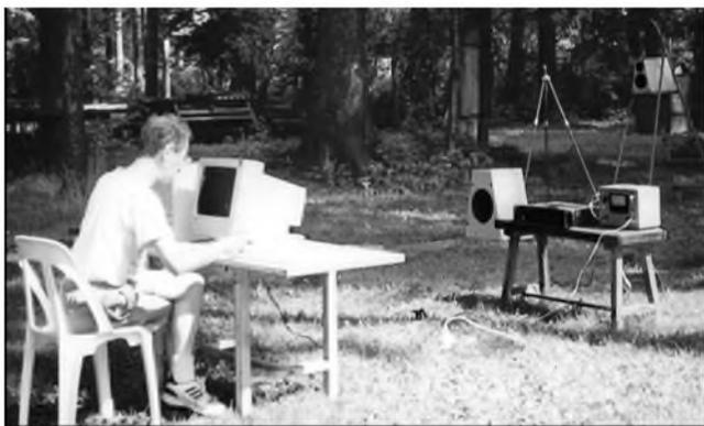
PHOTO 4: Ground plane and gated measurement of the drivers in cabinets.
