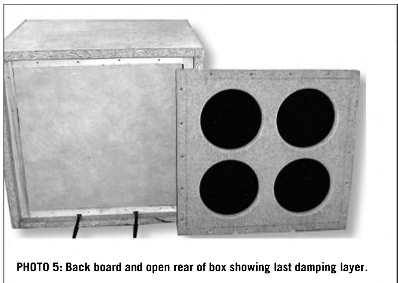
The back also has holes for 1 1/4" long #8 flat-head wood screws for attachment. Space these screws about every 3", since the back will tend to move because of the pressure on the damping layers. To keep all of the fiberglass-based damping material in-
