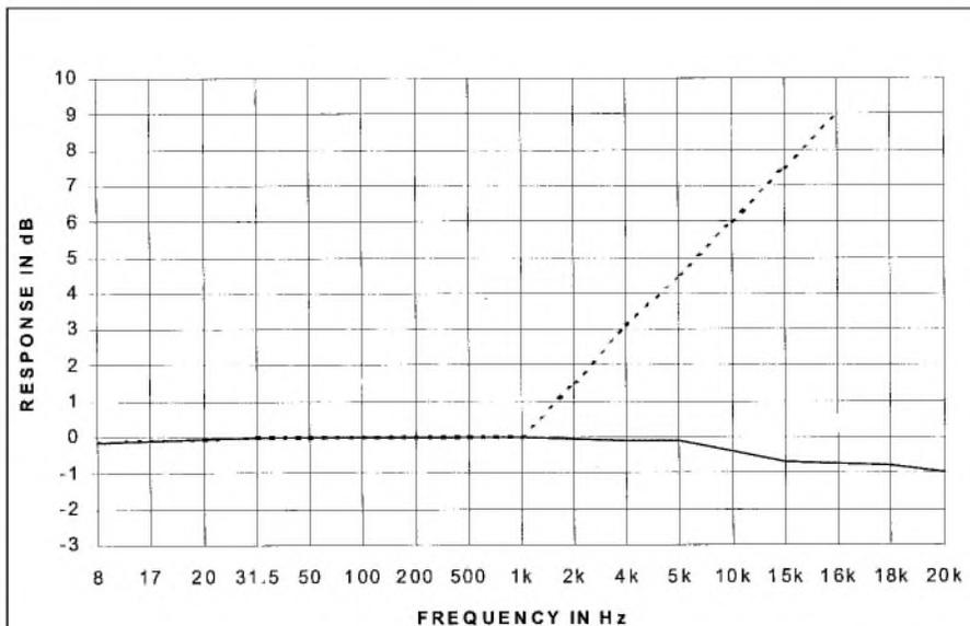
FIGURE 1: Solid line is the frequency response of the P-3A. The dashed line is the de-emphasis error. Strangely, the P-3A does not provide de-emphasis to CDs recorded with pre-emphasis.
