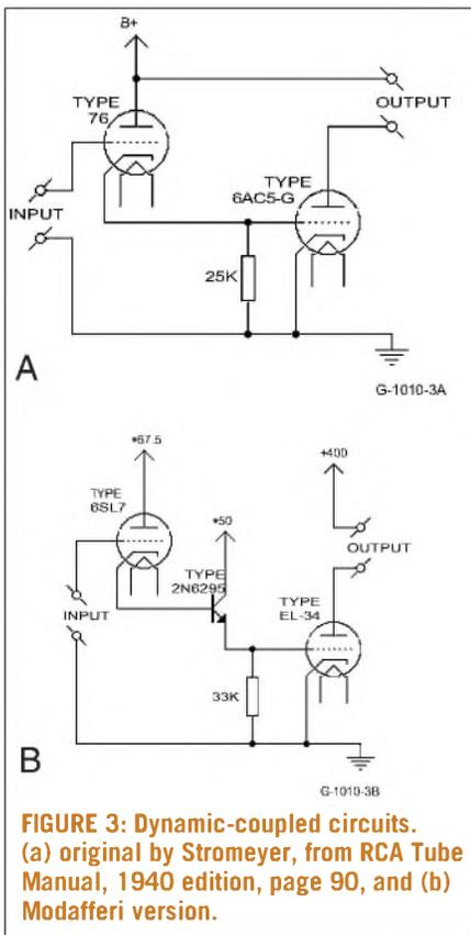
**FIGURE 3: Dynamic-coupled circuits. (a) original by Stromeyer, from RCA Tube Manual, 1940 edition, page 90, and (b) Modafferi version.**
