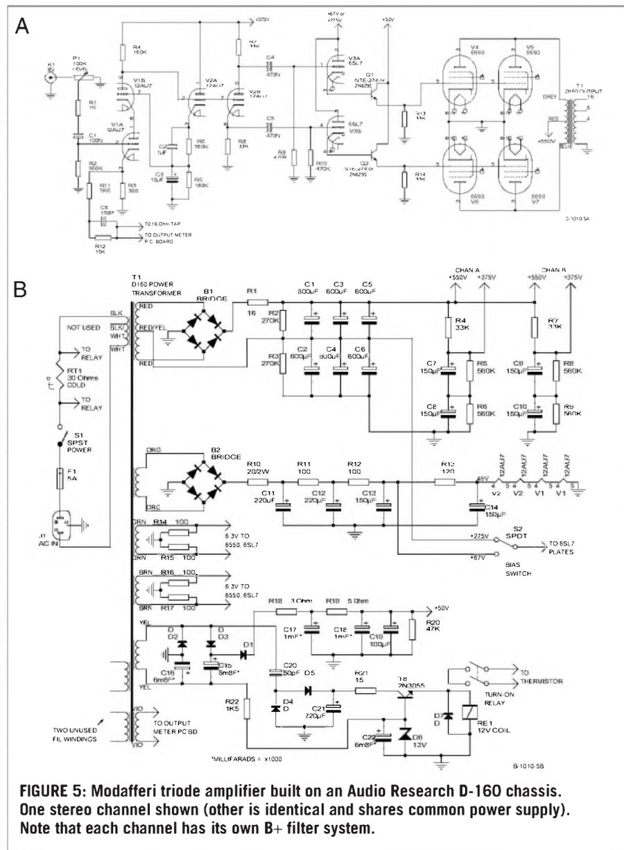
**FIGURE 5: Modafferi triode amplifier built on an Audio Research D-160 chassis. One stereo channel shown (other is identical and shares common power supply). Note that each channel has its own B+ filter system.**
