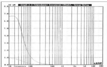
FIGURE 2: Low-frequency cone excursion simulation of the 10204 DVC in a 30 ltr sealed box at 1 and 40W.
