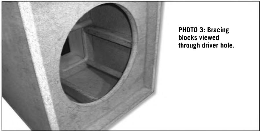
PHOTO 3: Bracing blocks viewed through driver hole.
