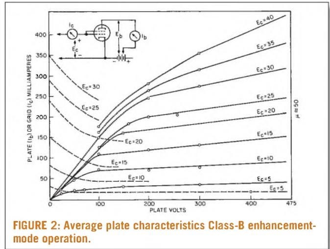
**FIGURE 2: Average plate characteristics Class-B enhancement-mode operation.**
