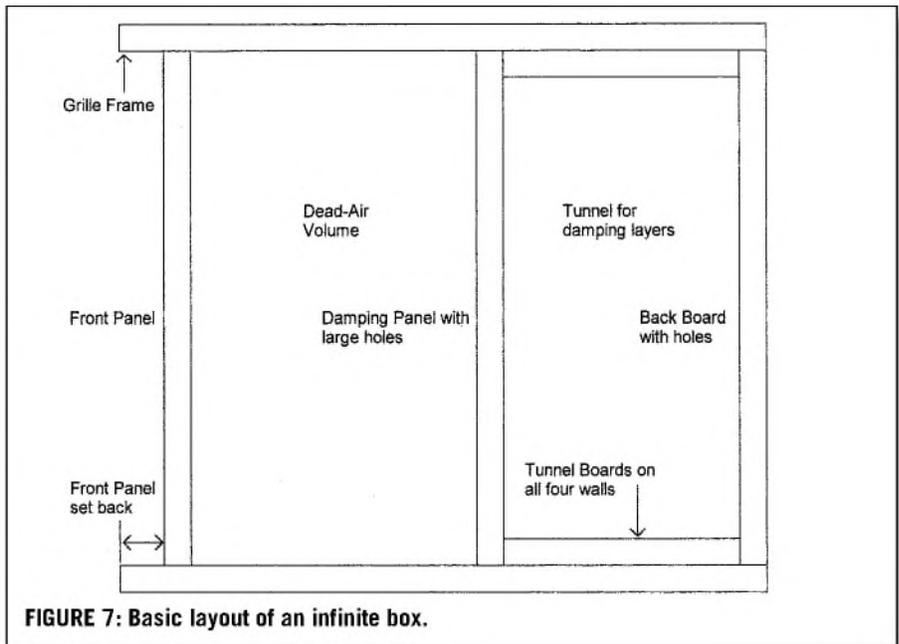
FIGURE 7: Basic layout of an infinite box.
