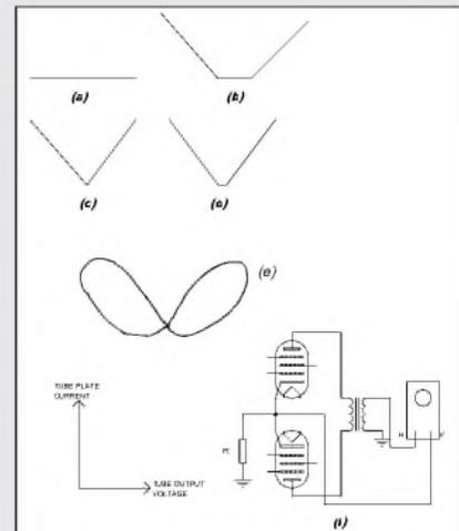
**FIGURE 12:** Output stage test waveforms. (a) ideal Class A, (b) ideal Class AB, (c) ideal Class B, (d) Opus 1 at 50W and 2kHz, (e) Opus 1 at 50W at 20kHz, (f) scope connections to output stage.
