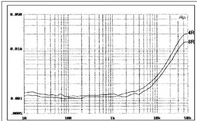
FIGURE 9: THD at 40W/8Ω and 80W/4Ω with doubled 3281/1302 output transistors. 4Ω THD has been halved compared with Fig. 8.
