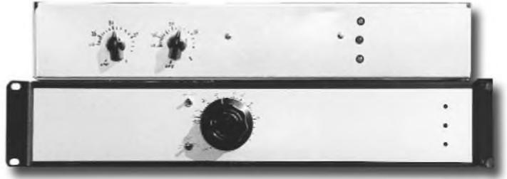
**PHOTO 1:** Basic single-channel-dual-output Big Mike preamp (bottom) and prototype two-channel Semi-Zen preamp (top).
