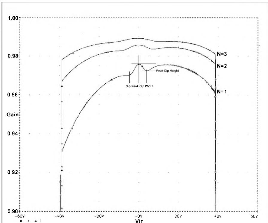
FIGURE 16: Simulation showing how as more devices are used the central gain-wobble that causes crossover distortion becomes flatter and spread over a wider range of output voltage.
