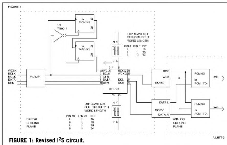
**FIGURE 1:** Revised I<sup>2</sup>S circuit.
