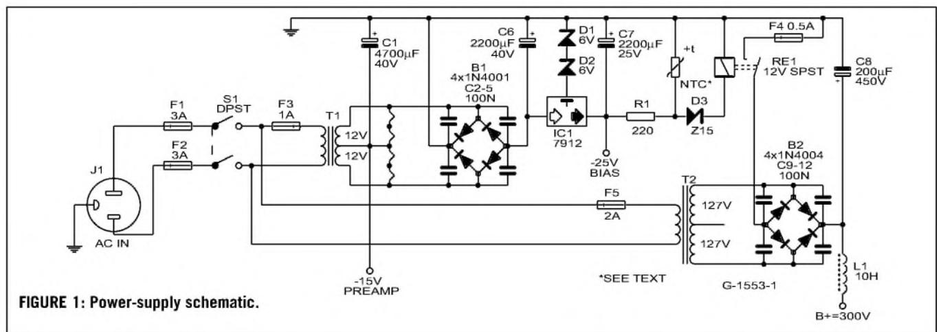
FIGURE 1: Power-supply schematic.
