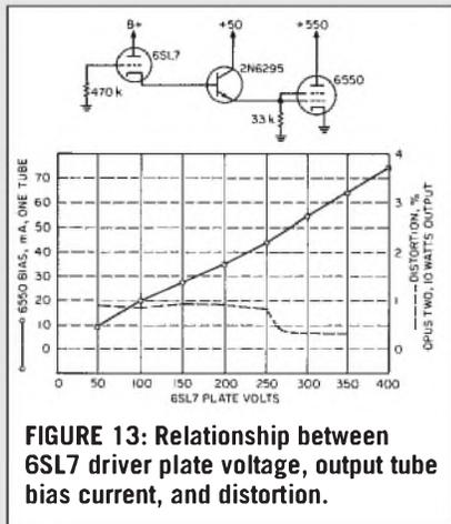
**FIGURE 13: Relationship between 6SL7 driver plate voltage, output tube bias current, and distortion.**
