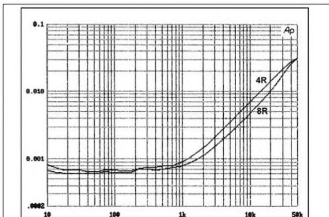
FIGURE 13: Measured THD for a triple-EF output stage with N=1 50W/8 $\Omega$ .
