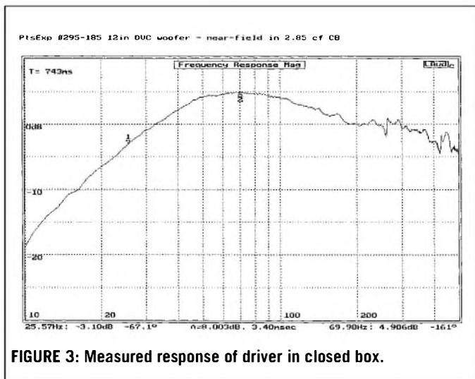
**FIGURE 3: Measured response of driver in closed box.**
