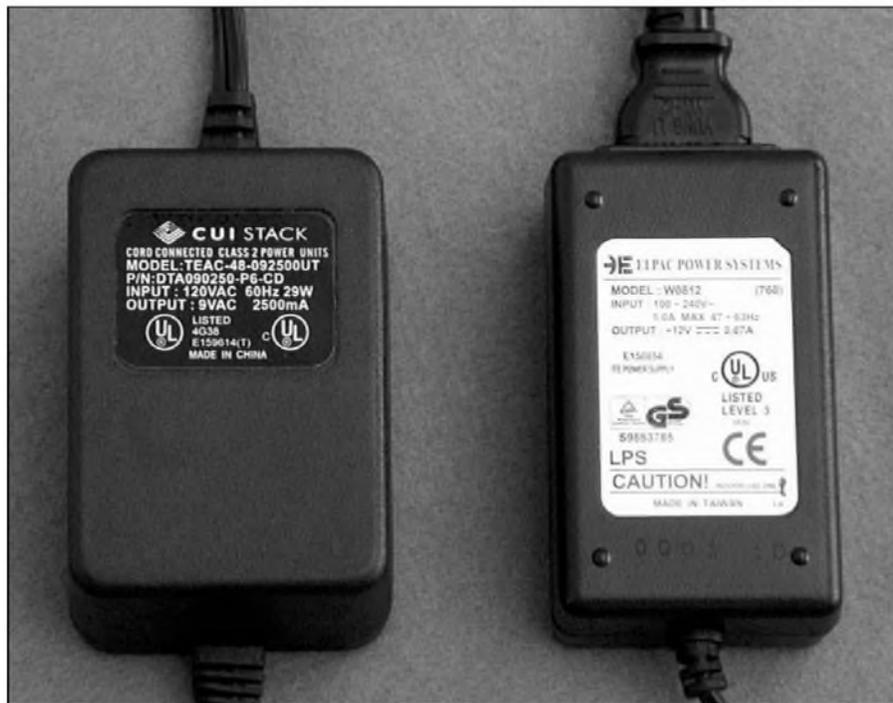
**PHOTO 5:** Outboard power supplies for the P-1A (left) and P-3A. The P-1A supply outputs 9V AC at 2.5A. The P-3A supply has an internal rectifier, and outputs +12V DC at 670mA. The DC power connectors are the same for both supplies.
