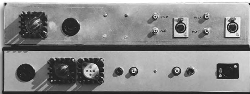
**PHOTO 2: Rear views of both preamps. The prototype Semi-Zen has two sets of RCA outputs; the upper ones have additional series capacitors to provide bass rolloff.**
