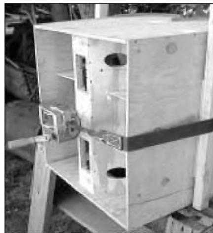
PHOTO 18: Using a webbing clamp and wooden caul to hold side in place for assembly.
