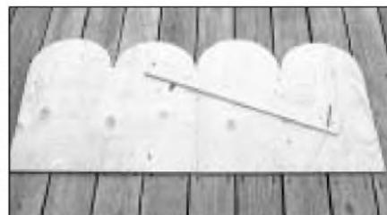
PHOTO 6: Using a long wooden compass to trace arcs.
