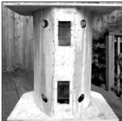
PHOTO 12: Assembly after cutting tweeter and duct mounting holes.
