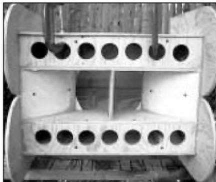
PHOTO 11: Pulling a mouth panel into place with clamps.
