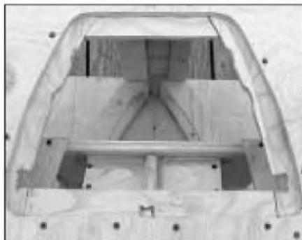
PHOTO 10: The flanged porthole. Note trimming to allow driver entry.
