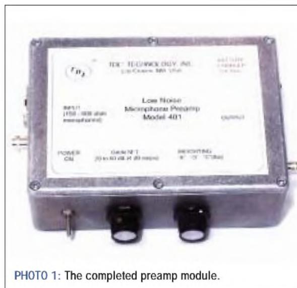
**PHOTO 1:** The completed preamp module.
