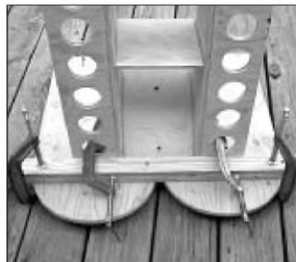
PHOTO 7: Using clamps and guideboard attaching throat horn to top.
