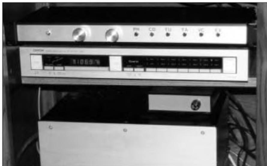
PHOTO 1: Borbely preamp shown with tuner and amplifier. Amplifier is a Borbely 60W, built using a Dynaco 150 chassis. The preamp power transformer is contained in the small enclosure above the amplifier.
