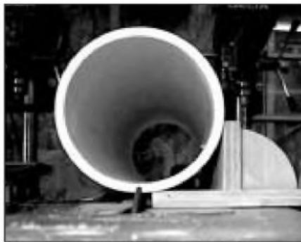
PHOTO 13: Holding PVC pipe with a jig for slicing on table saw.
