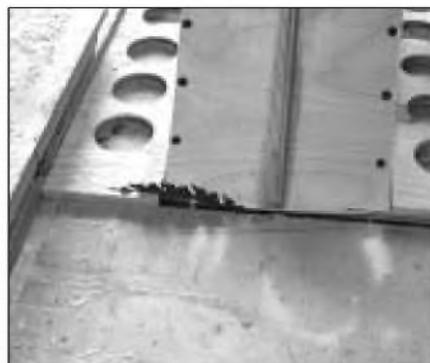
PHOTO 5: Trimming and squaring the throat horn assembly.
