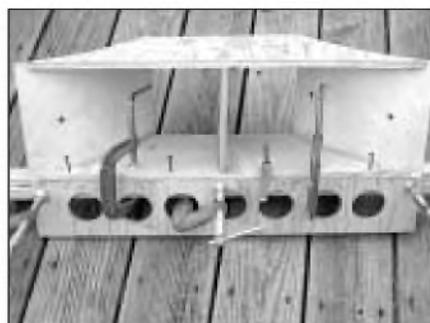
PHOTO 4: Using clamps and guideboard when attaching throat horn support.
