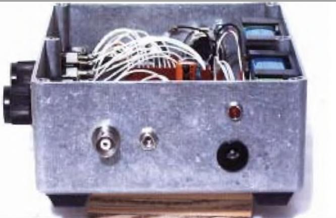
$\frac{5}{8}$ " machine screws, four internally threaded  $\frac{3}{8}$ " long nylon spacers, and four 4-40 hex nuts. Actually, only one or two nuts are needed, because the wiring helps hold the board in place. When the top cover is attached with its six screws, the result is a compact, well-shielded module.
