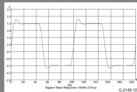
FIGURE 12: Square wave response, 10kHz 2.5Vpp 8Ω.
