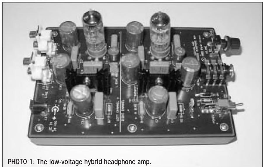
PHOTO 1: The low-voltage hybrid headphone amp.
