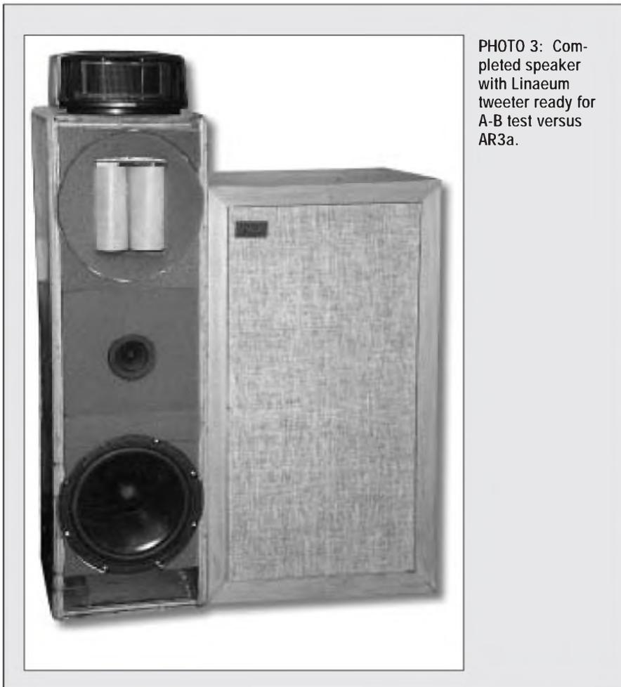
PHOTO 3: Completed speaker with Linaeum tweeter ready for A-B test versus AR3a.
