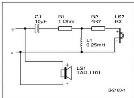
FIGURE 1: Filter configuration.
