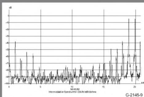
FIGURE 9: Spectrum of 19kHz + 20kHz intermodulation signal.
