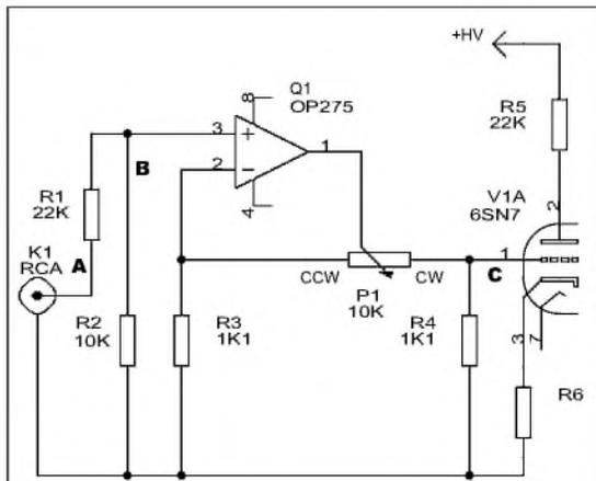
FIGURE 1: Log volume control with precision linear pot.
