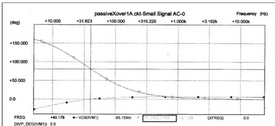
FIGURE 4: SPICE simulation of high-pass output. The input level, VM2, is +6.021dB. The output level, VM1, is -0.085dB at 40.179Hz and +6.002 at 1000Hz. The actual circuit measured within ±0.2dB.
