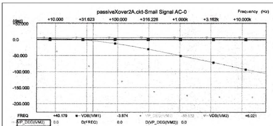
FIGURE 3: SPICE simulation of low-pass output. The input level, VM2, is +6.021dB. The output level, VM1, is -3.874dB at 40.179Hz and +2.15 at 16Hz. The actual circuit measured within ±0.2dB.
