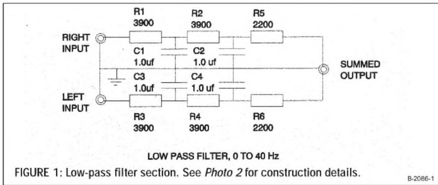
FIGURE 1: Low-pass filter section. See Photo 2 for construction details.
