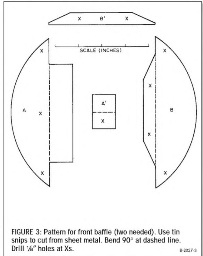
FIGURE 3: Pattern for front baffle (two needed). Use tin snips to cut from sheet metal. Bend 90° at dashed line. Drill 1/8" holes at Xs.
