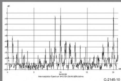
FIGURE 10: Spectrum of 9kHz + 10.05kHz + 20kHz intermodulation signal.
