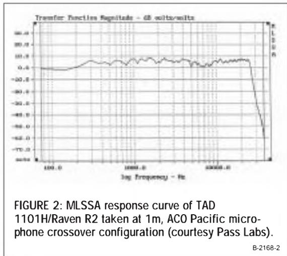
FIGURE 2: MLSSA response curve of TAD 1101H/Raven R2 taken at 1m, ACO Pacific microphone crossover configuration (courtesy Pass Labs).
