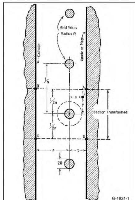
FIGURE 1: The section of a parallel plane triode.
