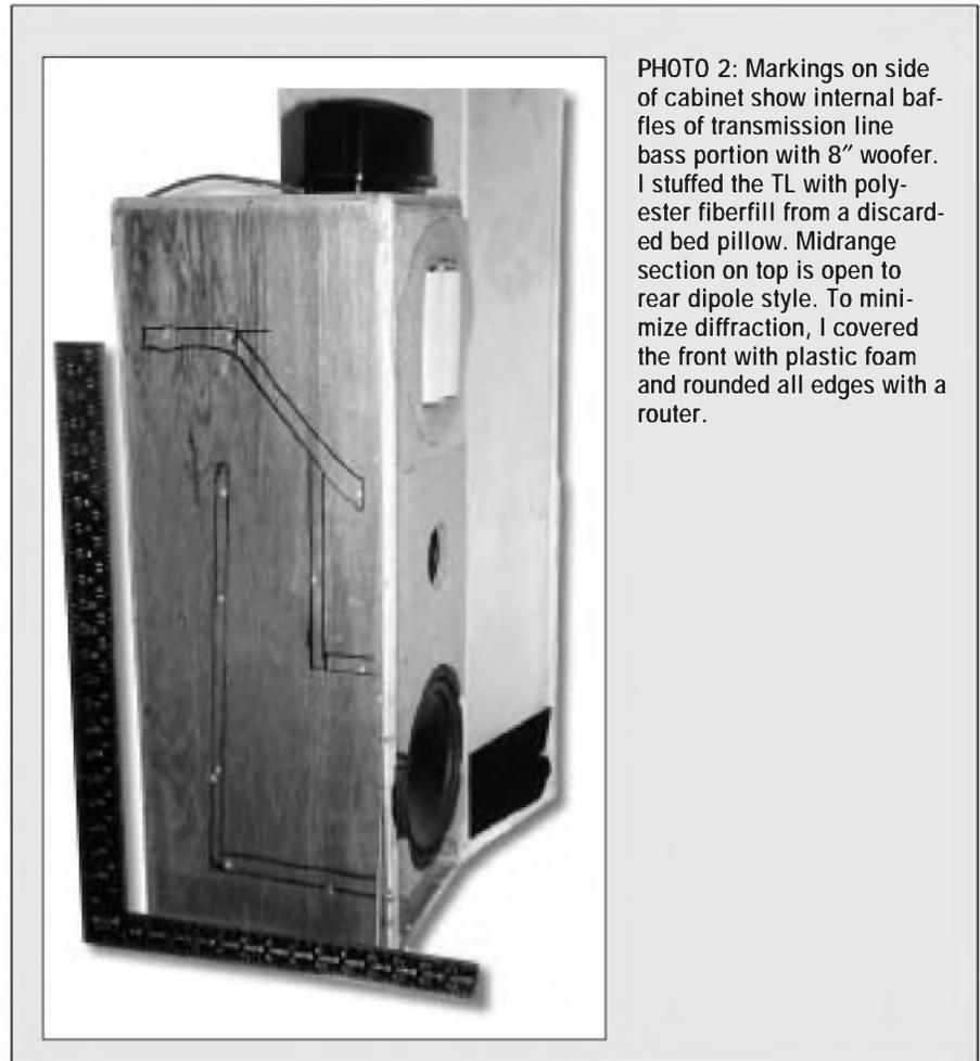
PHOTO 2: Markings on side of cabinet show internal baffles of transmission line bass portion with 8" woofer. I stuffed the TL with polyester fiberfill from a discarded bed pillow. Midrange section on top is open to rear dipole style. To minimize diffraction, I covered the front with plastic foam and rounded all edges with a router.
