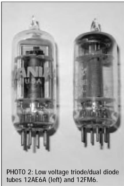
PHOTO 2: Low voltage triode/dual diode tubes 12AE6A (left) and 12FM6.
