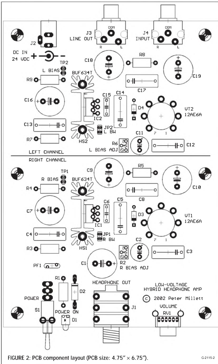
FIGURE 2: PCB component layout (PCB size: 4.75" x 6.75").
