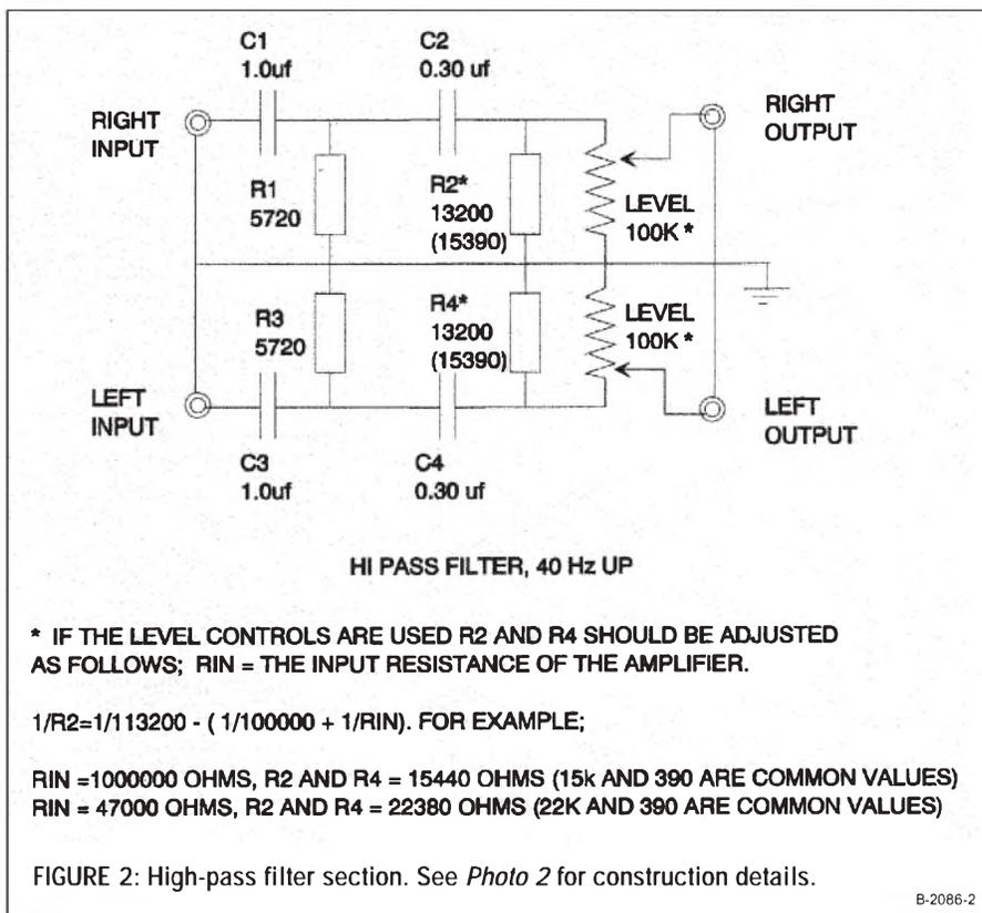
\* IF THE LEVEL CONTROLS ARE USED R2 AND R4 SHOULD BE ADJUSTED AS FOLLOWS;  $R_{IN}$  = THE INPUT RESISTANCE OF THE AMPLIFIER.
