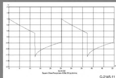
FIGURE 11: Square wave response, 40Hz 2.5Vpp 8Ω.
