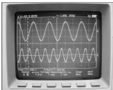
PHOTO 5: 12FM6, 13.5V bias, 1V RMS out (top) and distortion residual (bottom).
