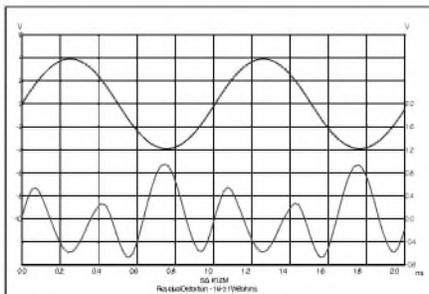
FIGURE 6: Residual distortion, 1kHz 1W 8Ω.
