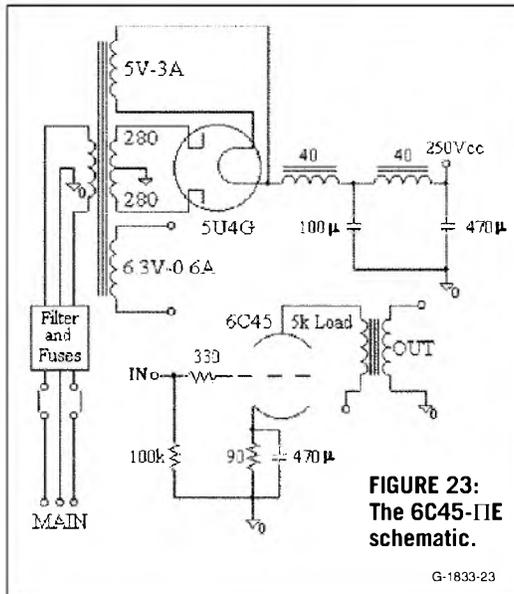
**FIGURE 23:** The 6C45-ΠE schematic.
