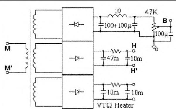
FIGURE 26: Low-voltage power supply schematic.
