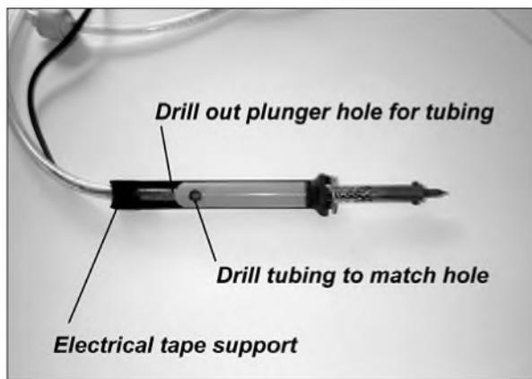
PHOTO 1: Modifications to desoldering iron.
