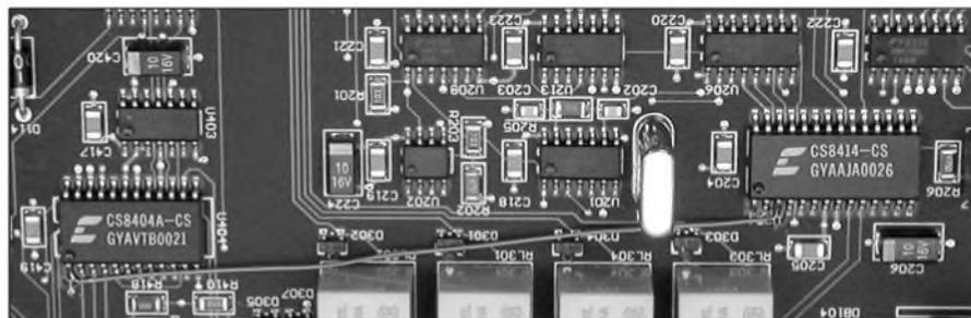
**PHOTO 1:** Close-up of the D2D-1 PC board with the de-emphasis mod installed. A piece of 30AWG wire-wrapping wire is tack-soldered between pin 1 of the CS8404A transmitter chip (left) and pin 3 of the CS8414 input receiver (right).
