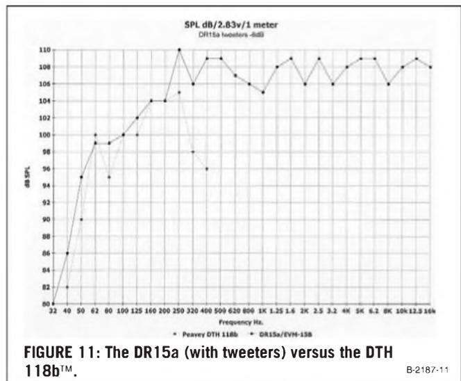
FIGURE 11: The DR15a (with tweeters) versus the DTH 118b™.
