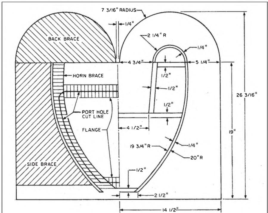
FIGURE 8: Top and bottom. Left side of view shows braces (shaded), right side shows parts locations.
