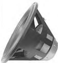
The larger woofers range from **10" to 18"** and all have **shielded magnets** and long excursions. Voice coils are from 2" diameter to 4" diameter. The 15" and 18" have **1.25"** of **x-max** in one direction.
