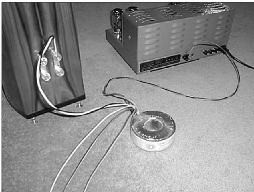
**PHOTO 1:** The ZERO speaker impedance multiplying autoformer used to multiply the impedance of any speaker so that it "feels" like the optimum load for the amplifier being used. For example, the ZERO can transform a 4 or 8 $\Omega$  speaker into a 16 $\Omega$  speaker.
