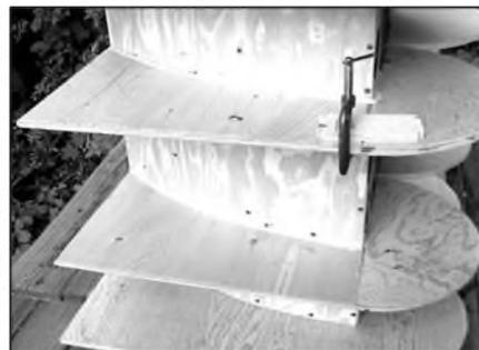
PHOTO 17: Using cauls to align a side brace.
