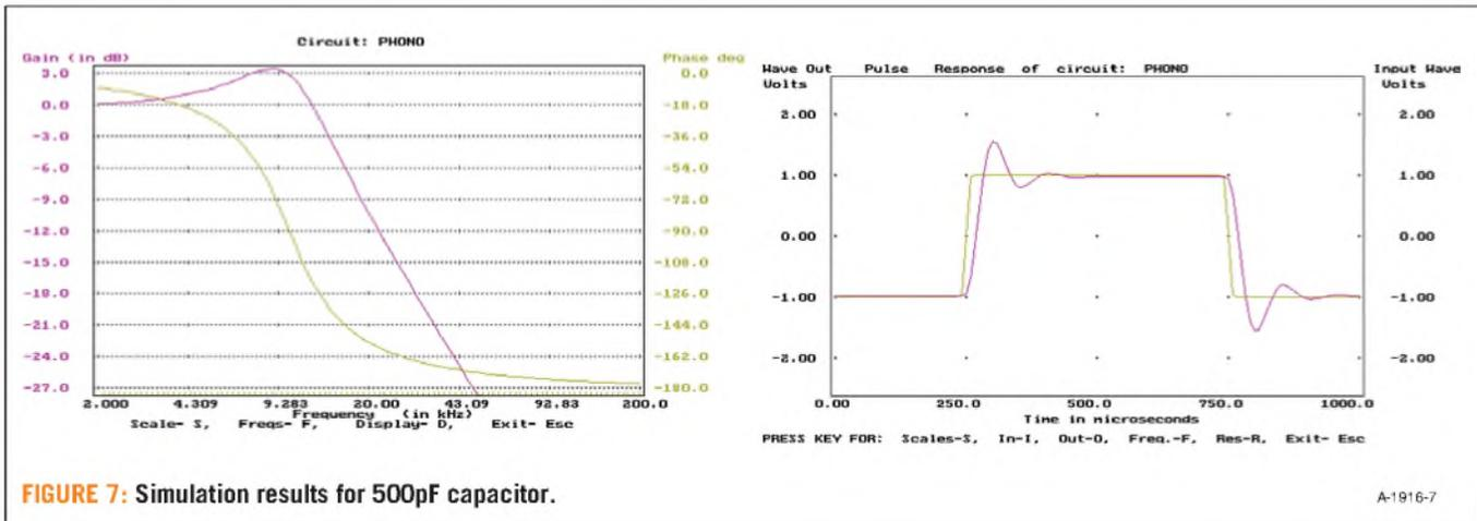
FIGURE 7: Simulation results for 500pF capacitor.
