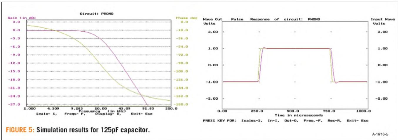
FIGURE 5: Simulation results for 125pF capacitor.
