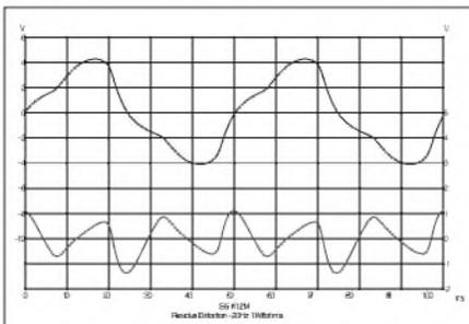
FIGURE 8: Residual distortion, 20Hz 1W 8Ω.
