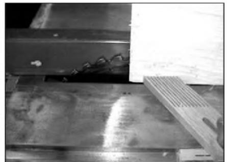
PHOTO 25: Using a featherboard with rip-guide to dado side edge.
