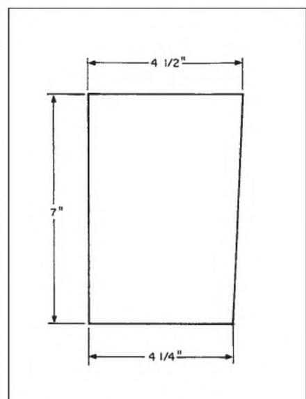
**FIGURE 6: Throat horn divider (two required).**
