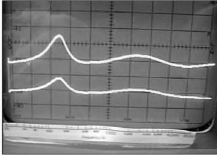
**PHOTO 2:** Frequency along the horizontal axis (log scale from 20 to 40kHz), and impedance along the vertical axis (2Ω/major line). Zero ohms is the bottom line, 2Ω on the next line above, 4Ω on the next line, and so on. The lower trace is of an actual 4Ω speaker. It exactly crosses 4Ω at the center line (1kHz). The upper trace shows the impedance of the same speaker after its impedance has been multiplied by two (2×) with the ZERO autoformer. It now crosses 8Ω at 1kHz.
