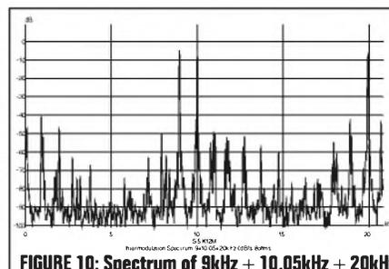
FIGURE 10: Spectrum of 9kHz + 10.05kHz + 20kHz intermodulation signal.
