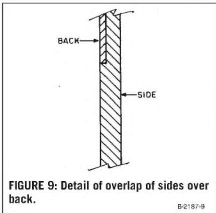
FIGURE 9: Detail of overlap of sides over back.
