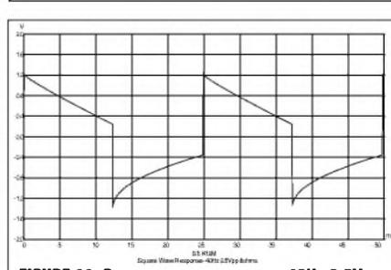
FIGURE 11: Square wave response, 40Hz 2.5Vpp 8Ω.
