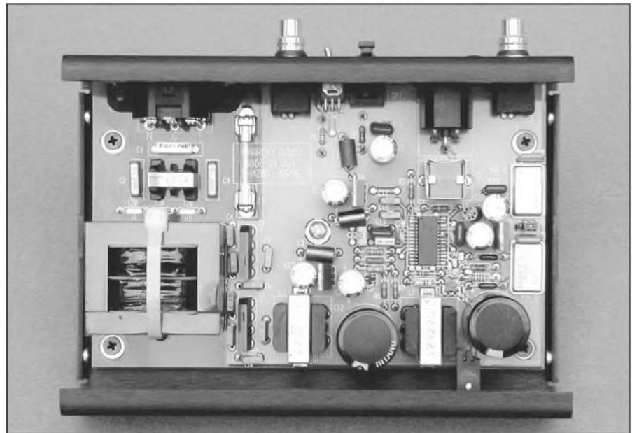
**PHOTO 3:** Inside the DIP Upsampler. You can see the industry-standard CS8420 Sample Rate Converter chip in its surface-mount package on the right. Four three-terminal supply regulators are included.
