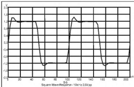
FIGURE 12: Square wave response, 10kHz 2.5Vpp 8Ω.
