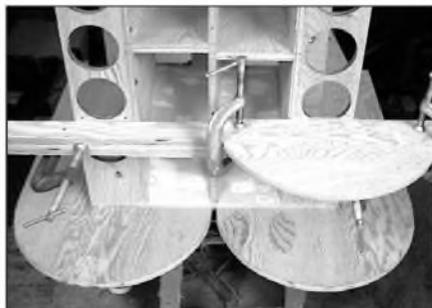
PHOTO 13: Aligning a back support.
