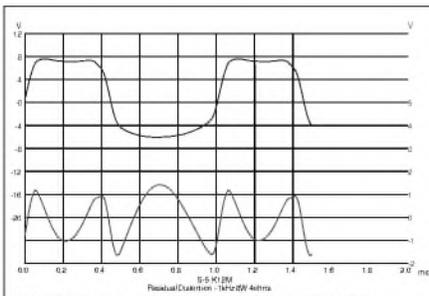
FIGURE 7: Residual distortion, 1kHz 8W 4Ω.
