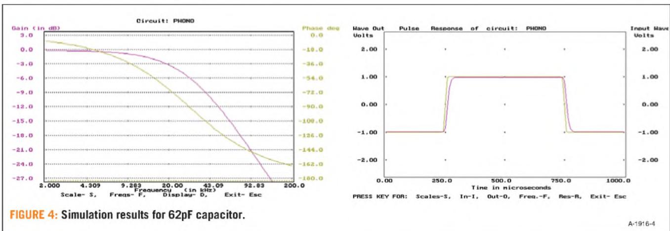
**FIGURE 4:** Simulation results for 62pF capacitor.
