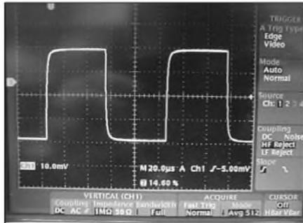
**PHOTO 7:** A 10kHz square wave signal passing through the properly loaded auto-former. The near vertical rising and falling edges along with the absence of any complex ringing shows one aspect of how much more transparent the ZERO autoformer is than a typical tube amp transformer.
