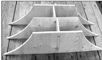
PHOTO 4: The throat horn sides/partition/divider assembly.
