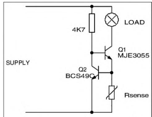
FIGURE 1B: Discrete current regulator.
