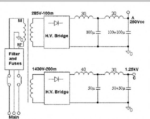
FIGURE 27: High-voltage power supply schematic.
