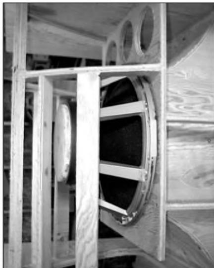
PHOTO 14: Make sure it fits! Note additional bracing.
