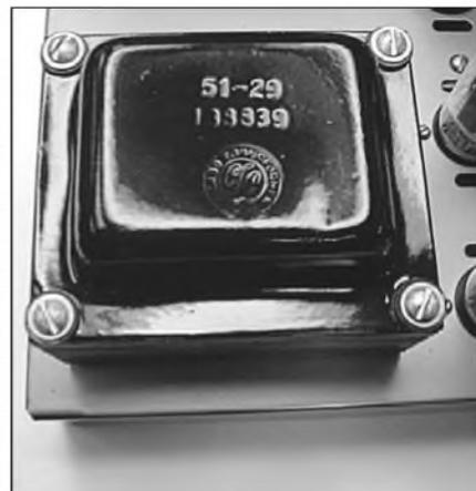
PHOTO 4: A “typical” tube amp transformer from a Heathkit UA-1 monoblock. Its 57.7:1 winding ratio provides a 13.3kΩ (plate to plate) to 4Ω impedance conversion.
