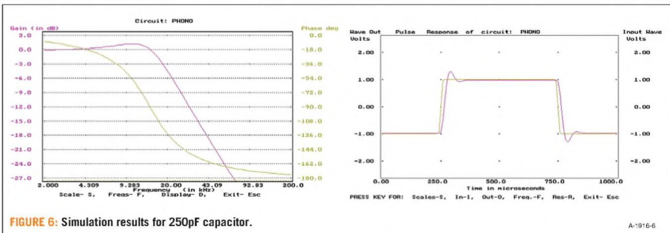
FIGURE 6: Simulation results for 250pF capacitor.
