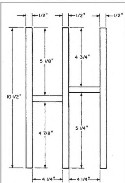
FIGURE 7: View of throat horn from baffle end, showing offset of throat dividers.
