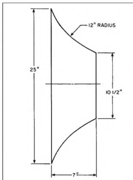
**FIGURE 5: Side view of throat horn sides and partition.**
