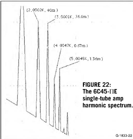
**FIGURE 22:** The 6C45-ΠE single-tube amp harmonic spectrum.
