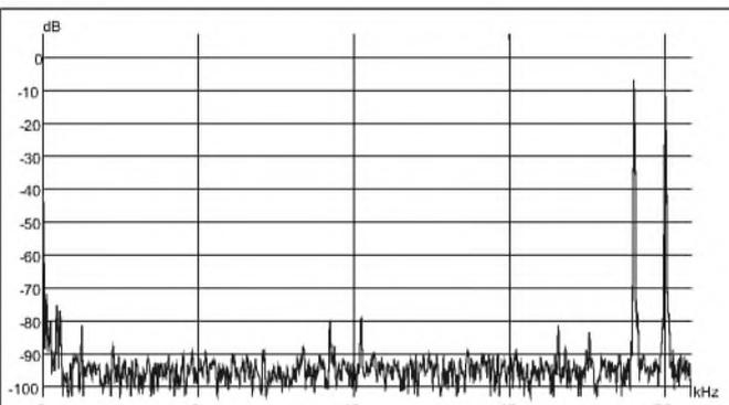
FIGURE 8: Intermodulation distortion, 19 + 20kHz 0dBfs (OPA604).
