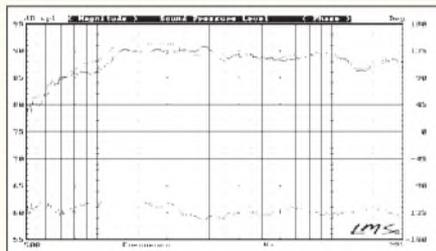
FIGURE 14: SPL of tweeter on enclosure with 4" beveled shell versus on IEC baffle (solid, lower line); difference curve raised 60dB. B-2151-14
