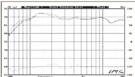
FIGURE 12: SPL of tweeter on enclosure with 1" radius shell versus enclosure without edge treatment (solid line); difference curve raised 60dB. B-2151-12
