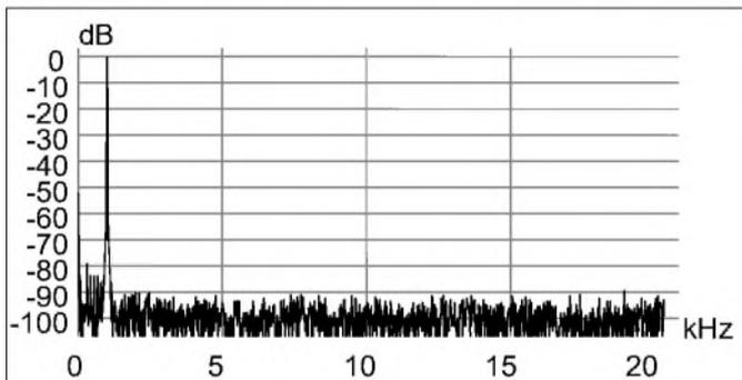
FIGURE 7: Spectrum of 1kHz sine wave. A-2169-7
