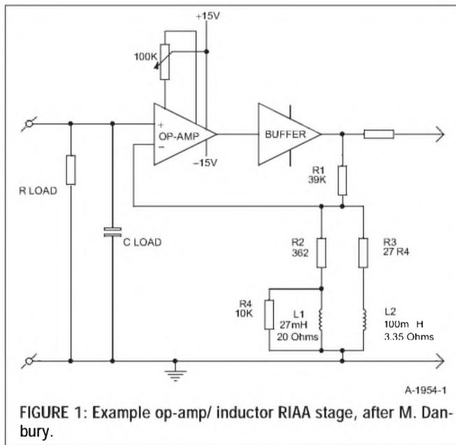
FIGURE 1: Example op-amp/ inductor RIAA stage, after M. Danbury.
