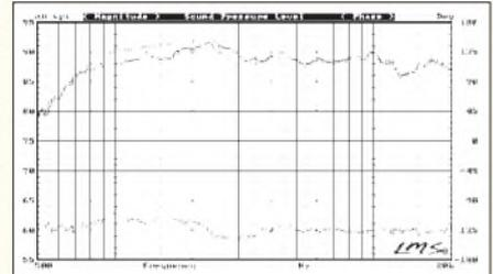
**FIGURE 3:** SPL of tweeter on IEC baffle with midbass uncovered (solid line) versus enclosure in free air; difference curve shows diffraction from enclosure edges.
