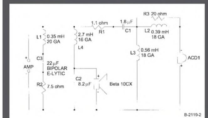
FIGURE 2: Crossover schematic (from Adire Audio assembly instructions).
