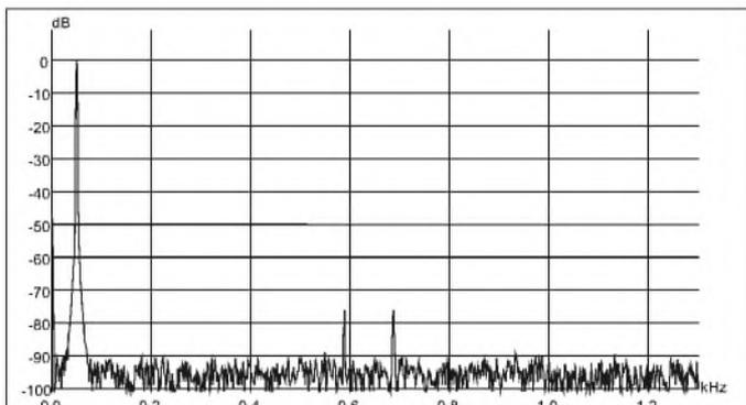
FIGURE 6: Spectrum of 50Hz sine wave (OPA604).
