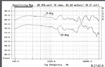
FIGURE 6: Response at 0 and 20° horizontal (20° offset -10dB).
