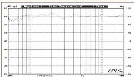
FIGURE 13: Comparison of SPL difference curve of 4" radius (lower line) versus difference curve of 1" radius. B-2151-13
