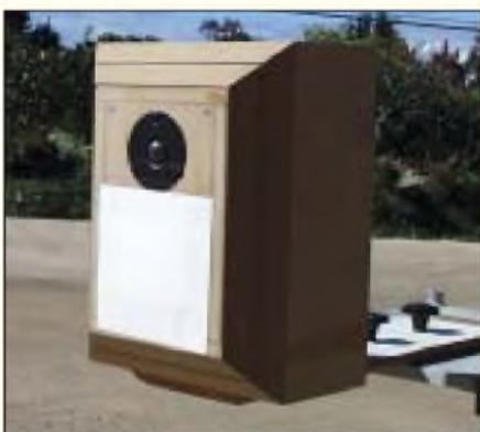
PHOTO 8: Test enclosure with 2", 45° bevel shell.
