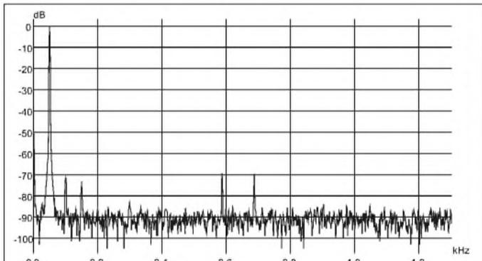
FIGURE 5: Spectrum of 50Hz sine wave (AD711).
