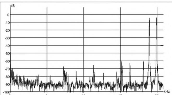
FIGURE 7: Intermodulation distortion, 19 + 20kHz 0dBfs (AD711).
