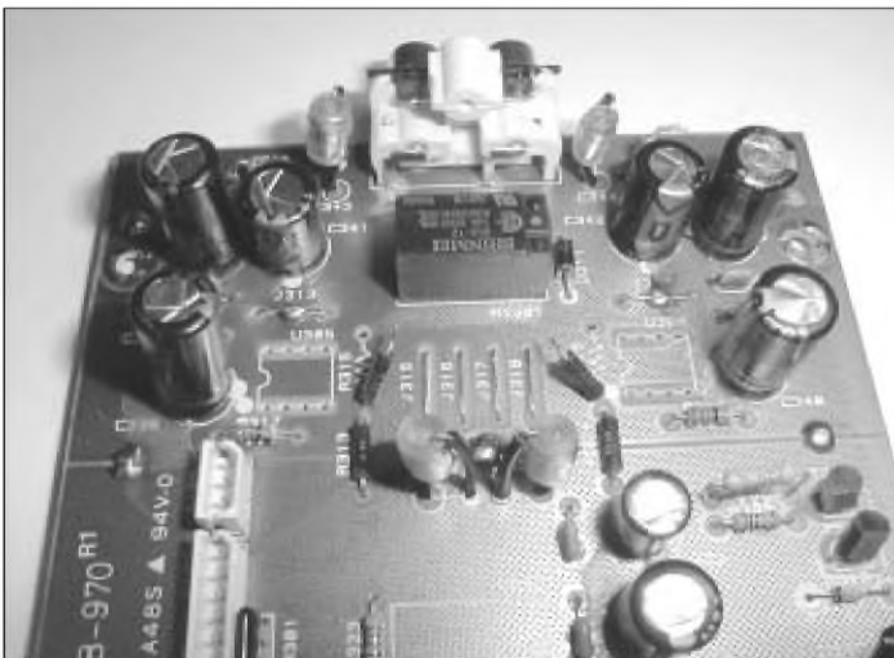
PHOTO 3: Board with ICs removed and resistors lifted.
