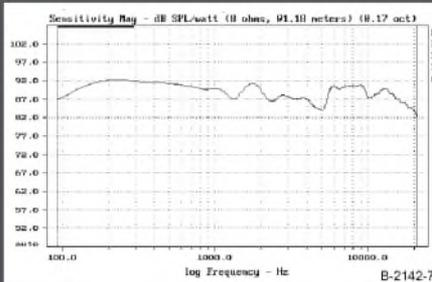
FIGURE 7: Average horizontal response  $\pm 30^\circ$ .
