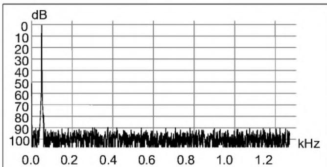
FIGURE 6: Spectrum of 50Hz sine wave. A-2169-6
