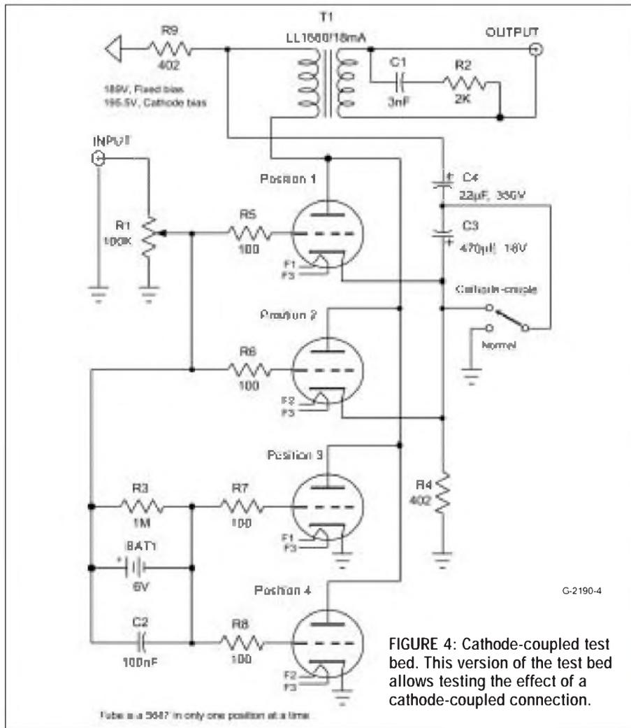
**FIGURE 4: Cathode-coupled test bed. This version of the test bed allows testing the effect of a cathode-coupled connection.**
