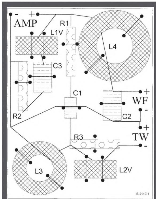
FIGURE 1: Suggested layout (from Adire Audio assembly instructions).
