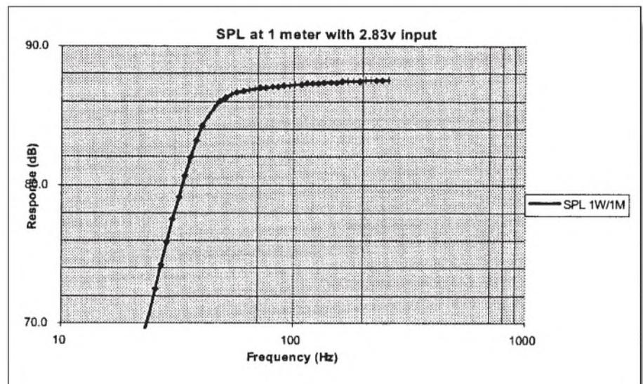
FIGURE 5: Maximum bass extension alignment for vented boxes per Weems, driver  $Q_{TS} = 0.3$ ,  $f_s = 30$ ,  $V_{AS} = 50$  ltr.
