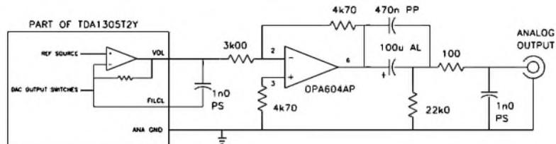
FIGURE 2: Modified analog output stage.
