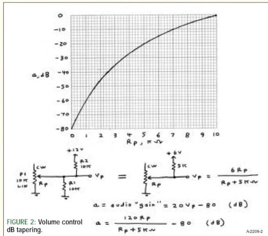
FIGURE 2: Volume control dB tapering.
