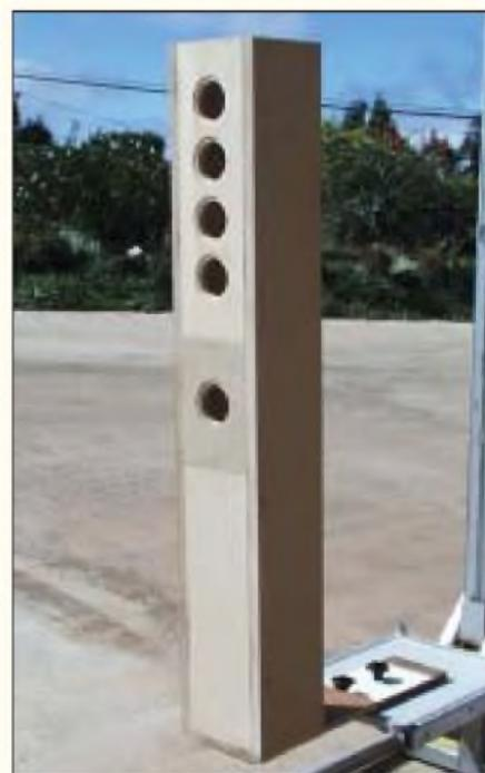
**PHOTO 3:** A test enclosure that is 8.875" wide and 56" tall.
