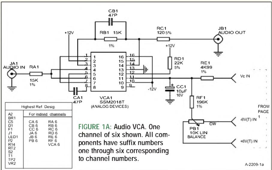
FIGURE 1A: Audio VCA. One channel of six shown. All components have suffix numbers one through six corresponding to channel numbers.
