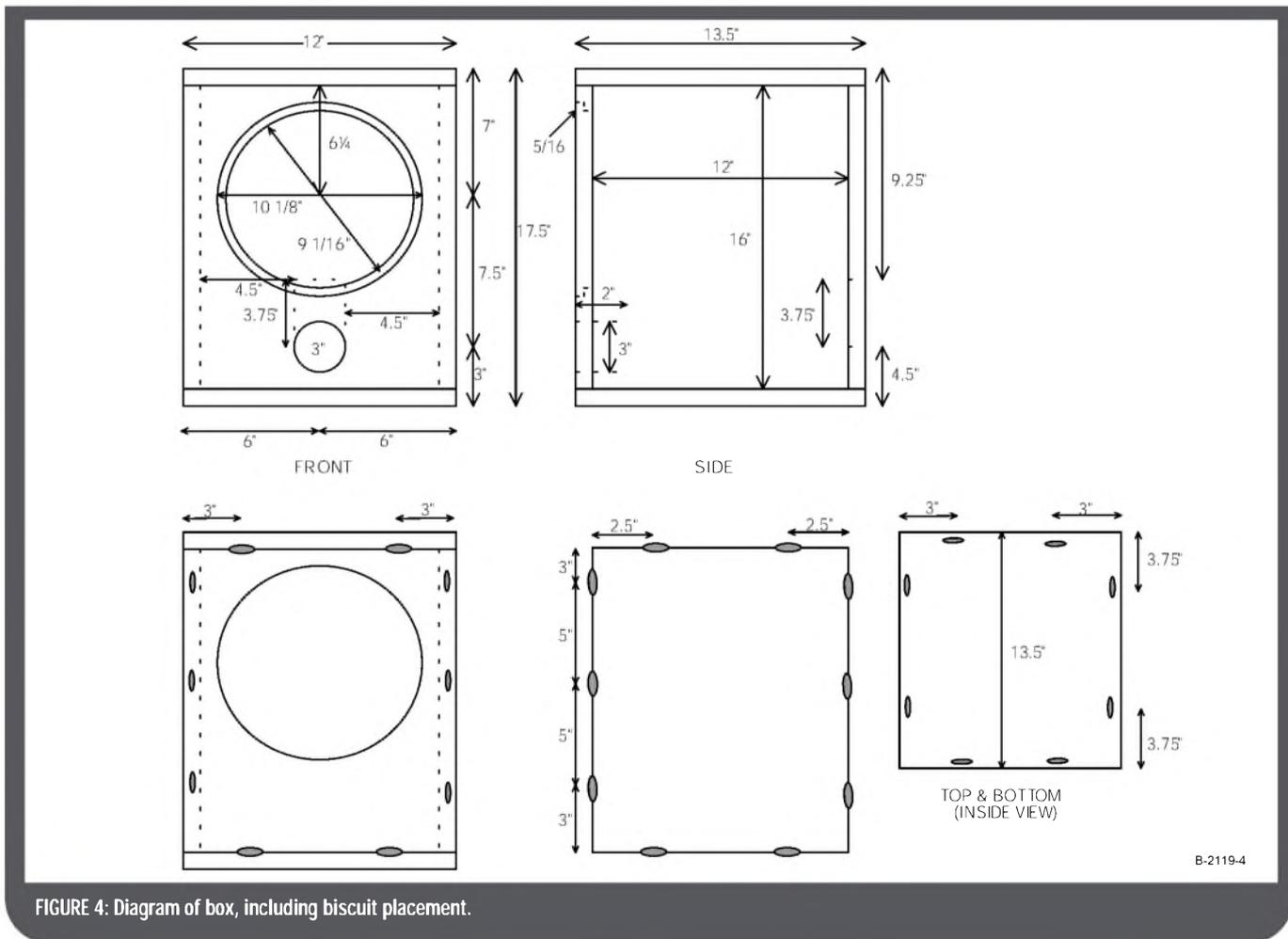
FIGURE 4: Diagram of box, including biscuit placement.
