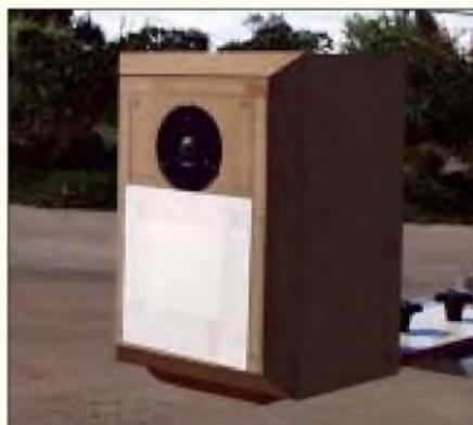
PHOTO 9: Test enclosure with 1", 45° bevel shell.
