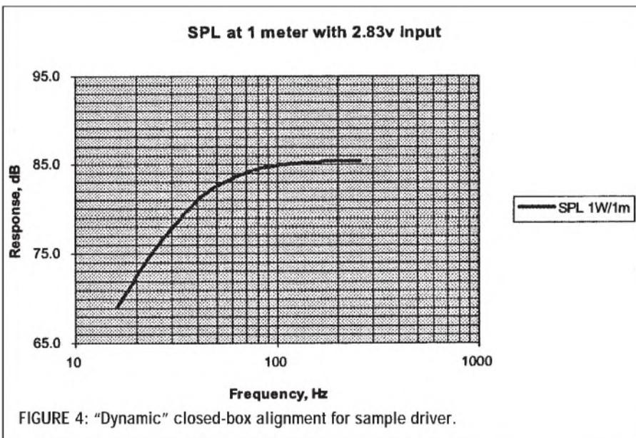
FIGURE 4: “Dynamic” closed-box alignment for sample driver.
