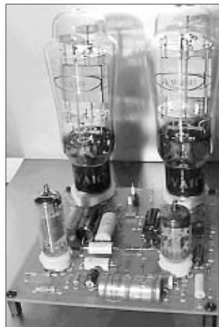
PHOTO 2: Testing THD with 6V30 power triodes.
