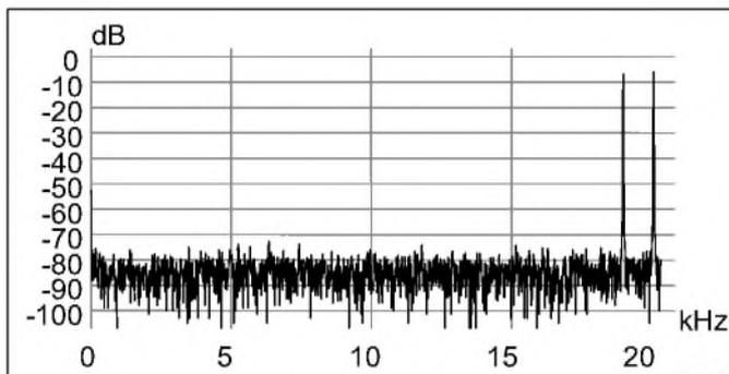
FIGURE 8: Spectrum of 19kHz + 20kHz intermodulation signal. A-2169-8
