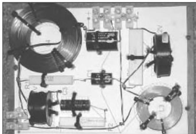
PHOTO 3: Assembled crossover with added compression connectors.
