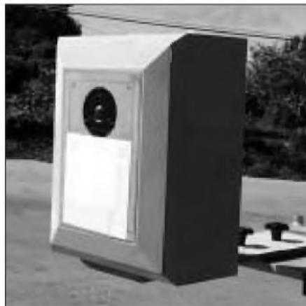
PHOTO 10: Test enclosure with dual bevel, 22°, 45° shell.
