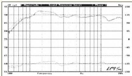
FIGURE 11: SPL of tweeter on enclosure with 2" radius shell versus enclosure without edge treatment (solid line); difference curve raised 60dB. B-2151-11
