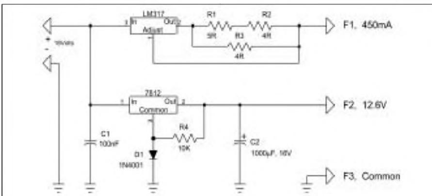
FIGURE 3: Voltage regulator and current regulator for test beds. G-2190-3
