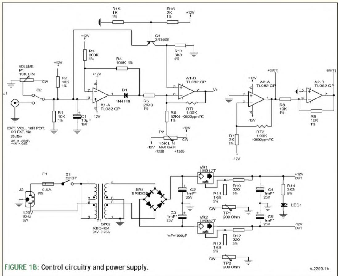
FIGURE 1B: Control circuitry and power supply.
