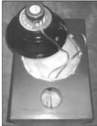
PHOTO 6: Assembled woofer and concentric tweeter just prior to installing the driver assembly.
