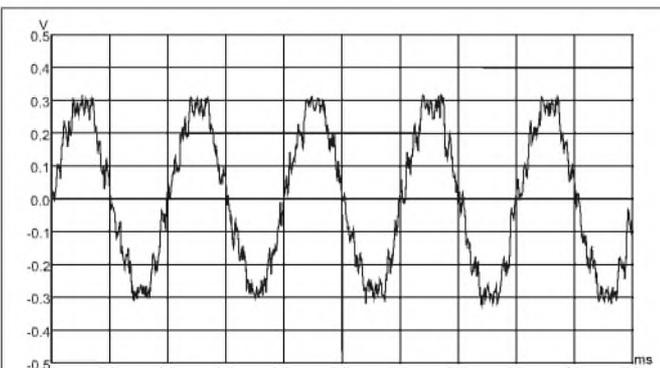
FIGURE 9: Undithered 1kHz sine wave at -90.31 dBFS.
