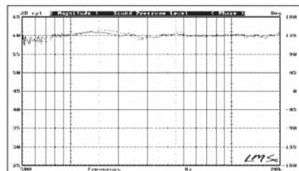
FIGURE 23: Comparison of SPL difference curve of 2" bevel (lower line) versus difference curve of dual bevel.
