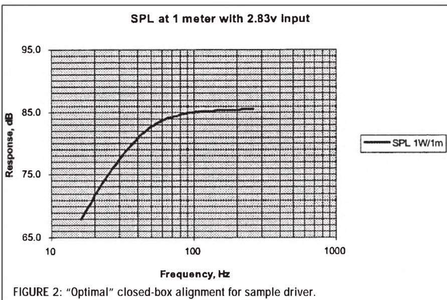
FIGURE 2: “Optimal” closed-box alignment for sample driver.
