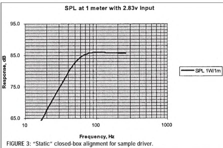
FIGURE 3: “Static” closed-box alignment for sample driver.
