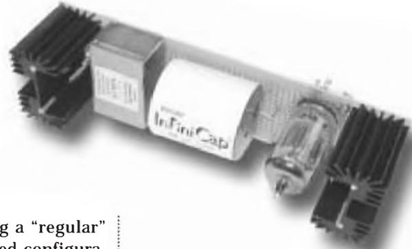
PHOTO 1: Line stage module. This is a single channel of the parafeed line stage prototype.
