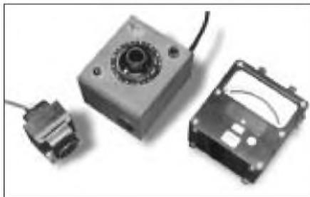
PHOTO 4: An isolation transformer, variable voltage transformer, and lab type meter are handy items for the experimenter.
