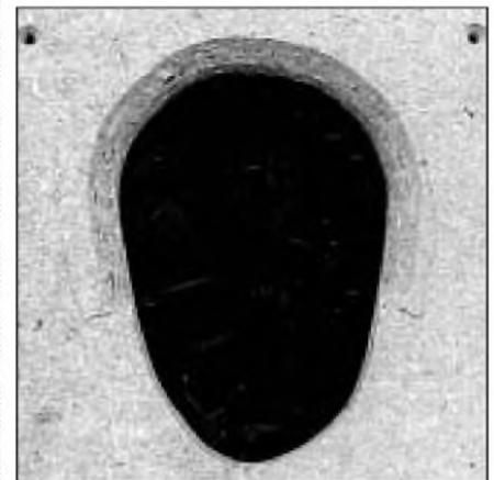
PHOTO 4: Shape of hole and relieving for Infinity plate driver.
