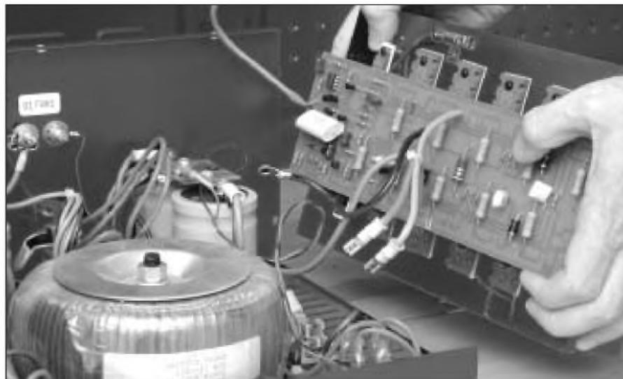
PHOTO 2: Removing a heatsink assembly.
