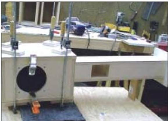
PHOTO 11: Gluing on the box sides.
