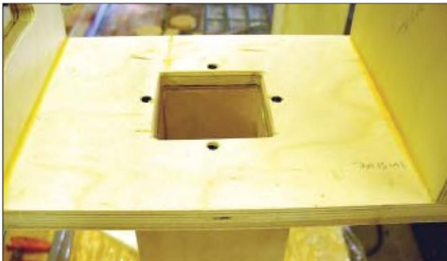
PHOTO 8: Attaching the open box to stand.
