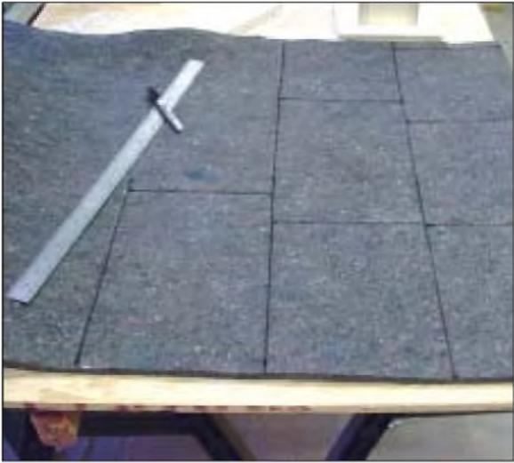
PHOTO 9: Cutting the felt.
