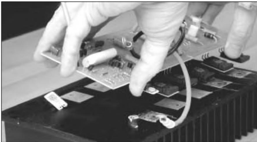
PHOTO 3: Removing the original PC board.
