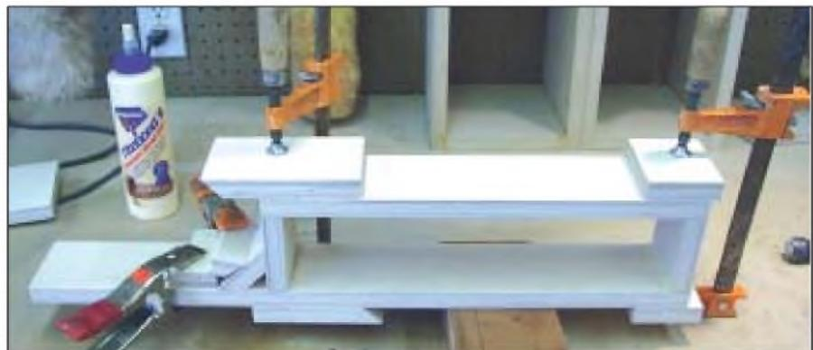
PHOTO 3: Gluing the bottom of the stand.
