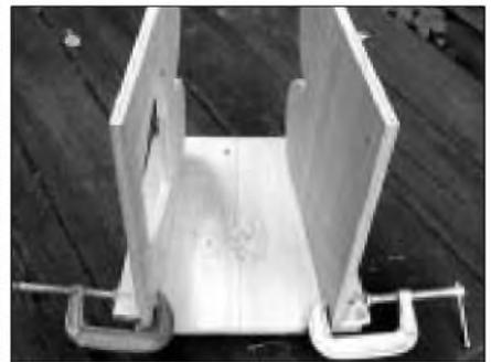
PHOTO 17: Using a jig to align the top and bottom for assembly.
