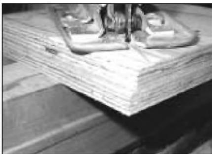
PHOTO 3: Simul-cutting throat horn sides.
