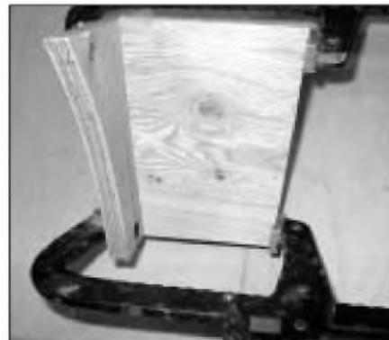
PHOTO 5: Beginning the throat horn assembly.
