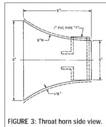
FIGURE 3: Throat horn side view.
