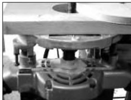
PHOTO 14: Trimming radiused parts with a table-mounted router.
