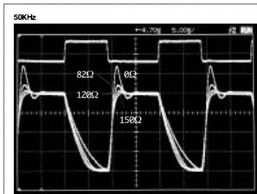
FIGURE 9: Damping resistor.
