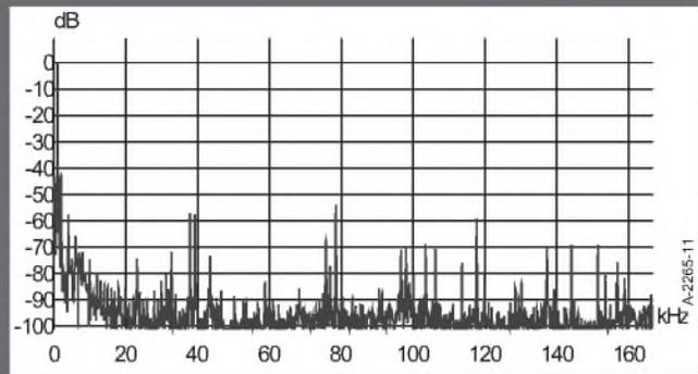
FIGURE 11: Spectrum with ATX switching power supply.
