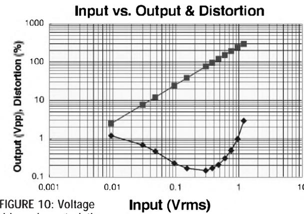
FIGURE 10: Voltage driver characteristics.
