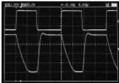
Falling Edge was degraded due to the input stray capacitance of oscilloscope probing
