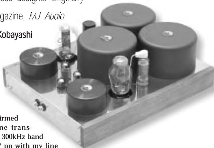
already confirmed that this line transformer has a 300kHz bandwidth at 20V pp with my line amplifier design driven by a 6N1P
