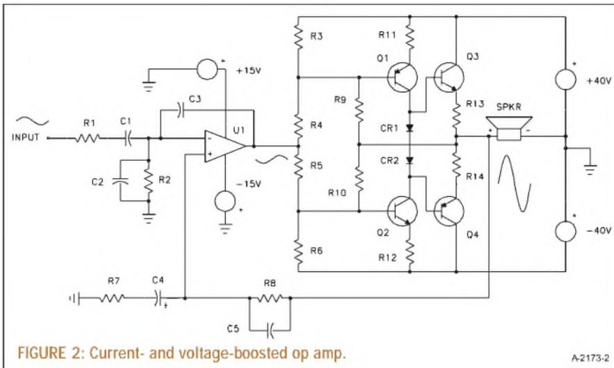
FIGURE 2: Current- and voltage-boosted op amp.
