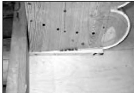
PHOTO 23: Rough-trimming the cabinet side.
