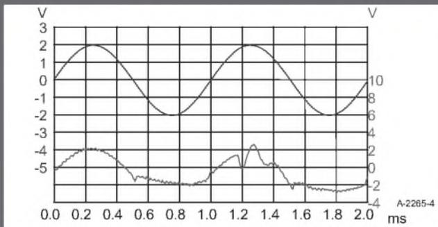
FIGURE 4: Residual distortion.
