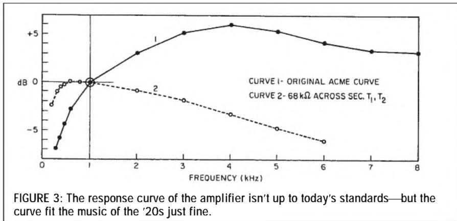
FIGURE 3: The response curve of the amplifier isn't up to today's standards—but the curve fit the music of the '20s just fine.
