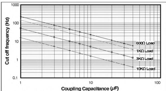
FIGURE 8: Coupling capacitance.
