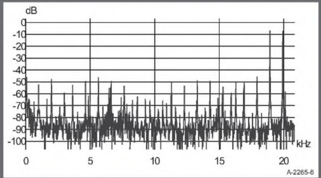
FIGURE 6: Spectrum of 19kHz + 20kHz intermodulation signal.
