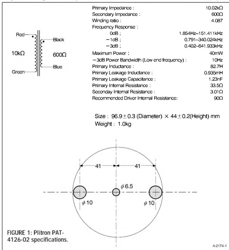
FIGURE 1: Plitron PAT-4126-02 specifications.
