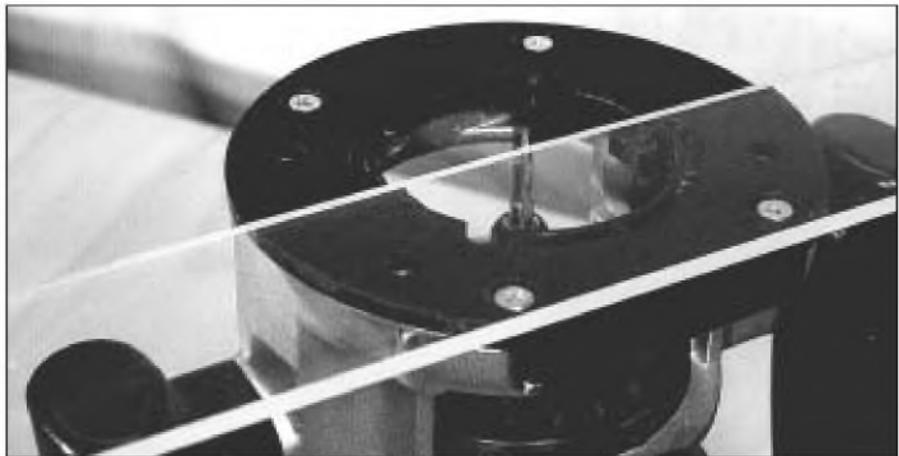
PHOTO 6: The router bar provides the distance from the bit to the edge of the router base.
