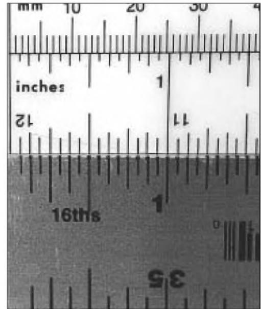
PHOTO 1: The shadow makes this look worse than it is, but the first sixteenth on the bottom scale is more like  $\frac{5}{32}$ ", making the scale unusable from the end.
