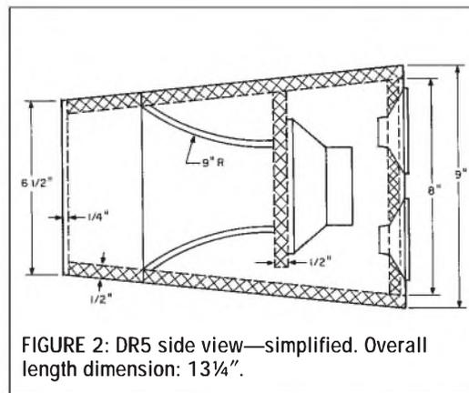
FIGURE 2: DR5 side view—simplified. Overall length dimension: 13  $\frac{1}{4}$ ".
